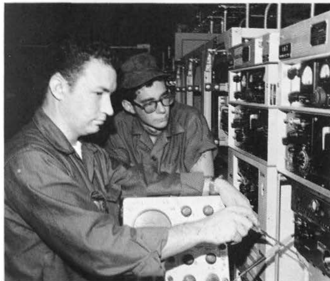
F.J. Nadeau, ET1, and D.C. Storkan, ETR3, test transmitter on oscilloscope
