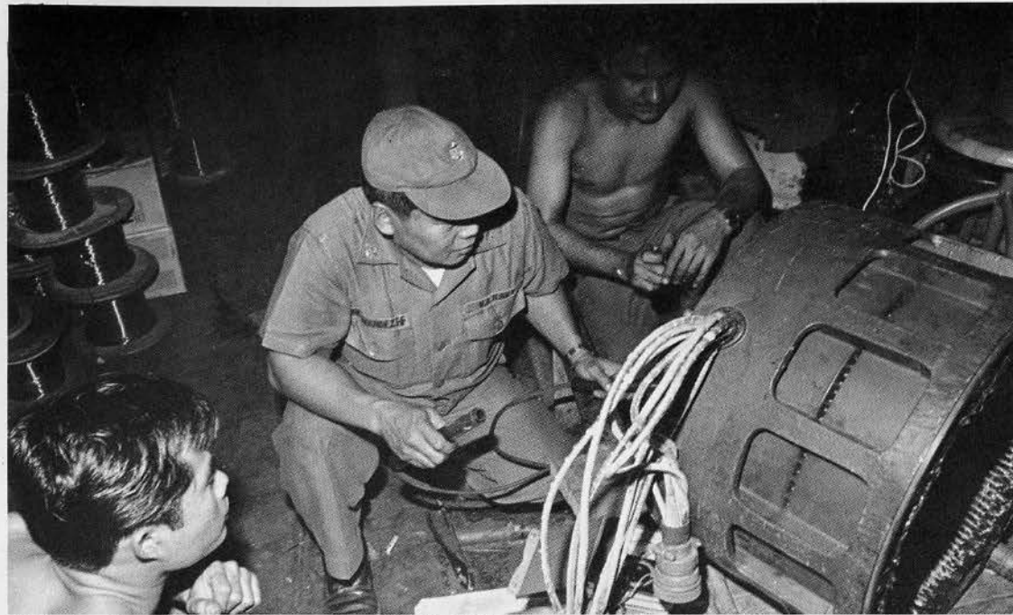
N.M. Angeles, EM1; F.F. Fernandez, EMCS; H.V. Rodgers, SD3 rewiring 400 cycle generator
