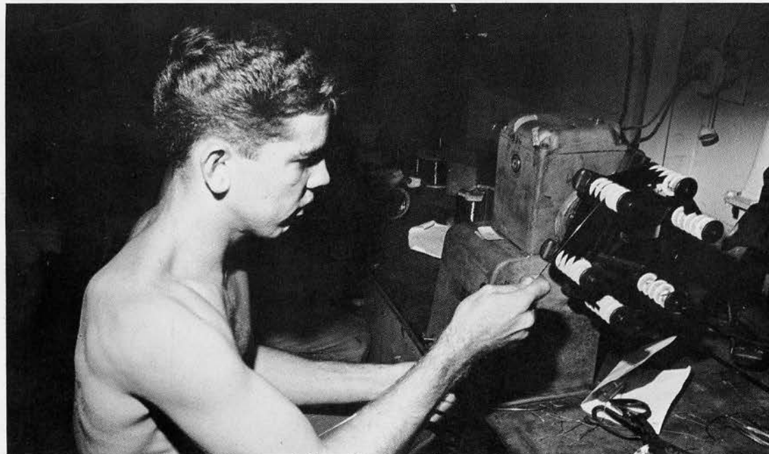
R. Bullard, CEW2, making coils on rewind machine
