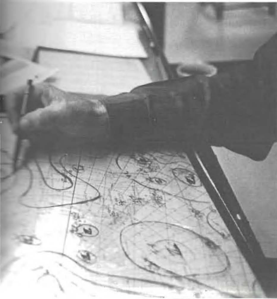
PLOTTING THE TREND of an upper air sounding chart, Airman James M. Kelly records the information from which the temperature, relative humidity and other data may be obtained.
