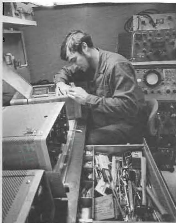
REPAIRING A CHASSIS on a field party radio transmitter, Electronics technician third class Bryan McDermott reworks it for reissue to one of the many scientific units working nearby.
