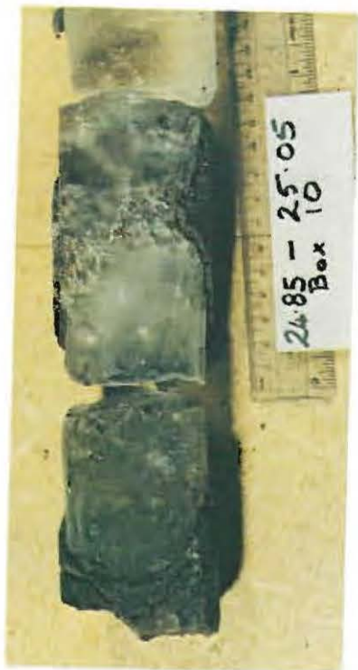
THE FIRST CORES taken from beneath Ross Island (ABOVE AND BELOW) show the permafrost extending many feet below the surface, with layers of lava-origin soil separating the different strata.
