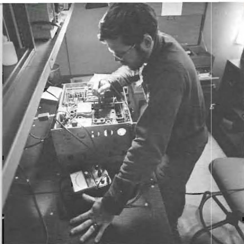
CHECKING FOR A SHORT in a radio receiver, Electronics technician third class Henry Rolin uses a multimeter to test each phase of the circuit until the malfunction is located for repair.
