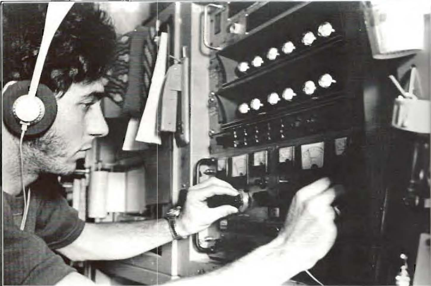
ADJUSTING THE GAIN control, Don W. Baker tunes in a satellite signal to record the data being transmitted back to earth.
