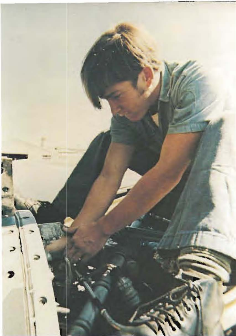
REPAIRING AN ELECTRICAL FAULT in a C-130 Hercules engine, Electrician's Mate second class Andy Piper (RIGHT) assists in a major check of the aircraft at the squadron's Christchurch facility.
