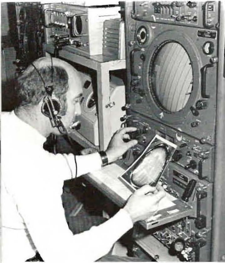
RUNNING A MAINTENANCE CHECK on the ground control approach system, (ABOVE) Air Controlman first class "Curley" Gaston adjusts a setting.
