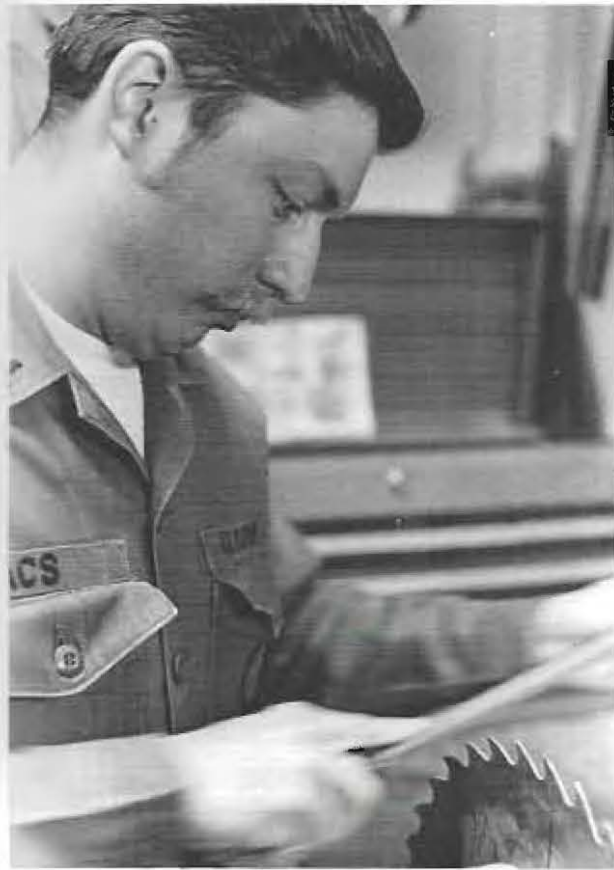
KEEPING A GOOD CUTTING EDGE, Builder first class Frank Acs, (BELOW) begins the exacting task of filing a circular saw blade.
