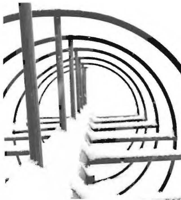
LIKE A GIANT corkscrew, the antenna (ABOVE) rotates a complete 360^\circ and can be raised 90^\circ from horizontal. When installed, it received data from ESSA VIII and Nimbus IV weather observing satellites.
