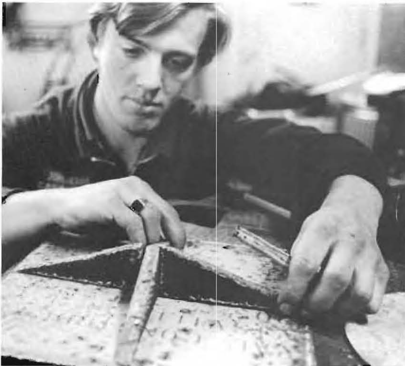
ALIGNING PARTS FOR WELDING, New Zealand Caterpillar mechanic Howard Berendt (ABOVE) repairs tractors in the McMurdo garage.
