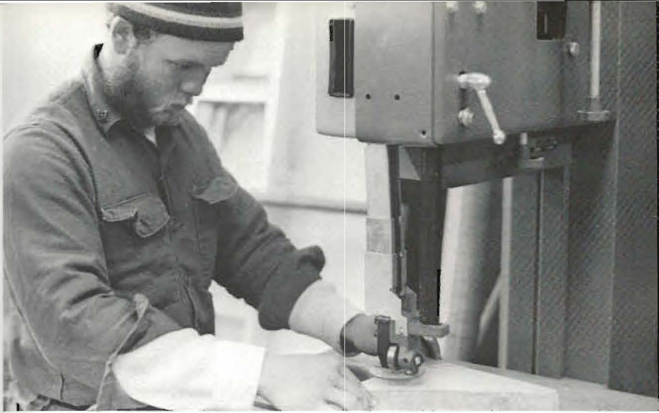
KEEPING A GOOD CUTTING EDGE, Builder first class Frank Acs, (BELOW) begins the exacting task of filing a circular saw blade.
