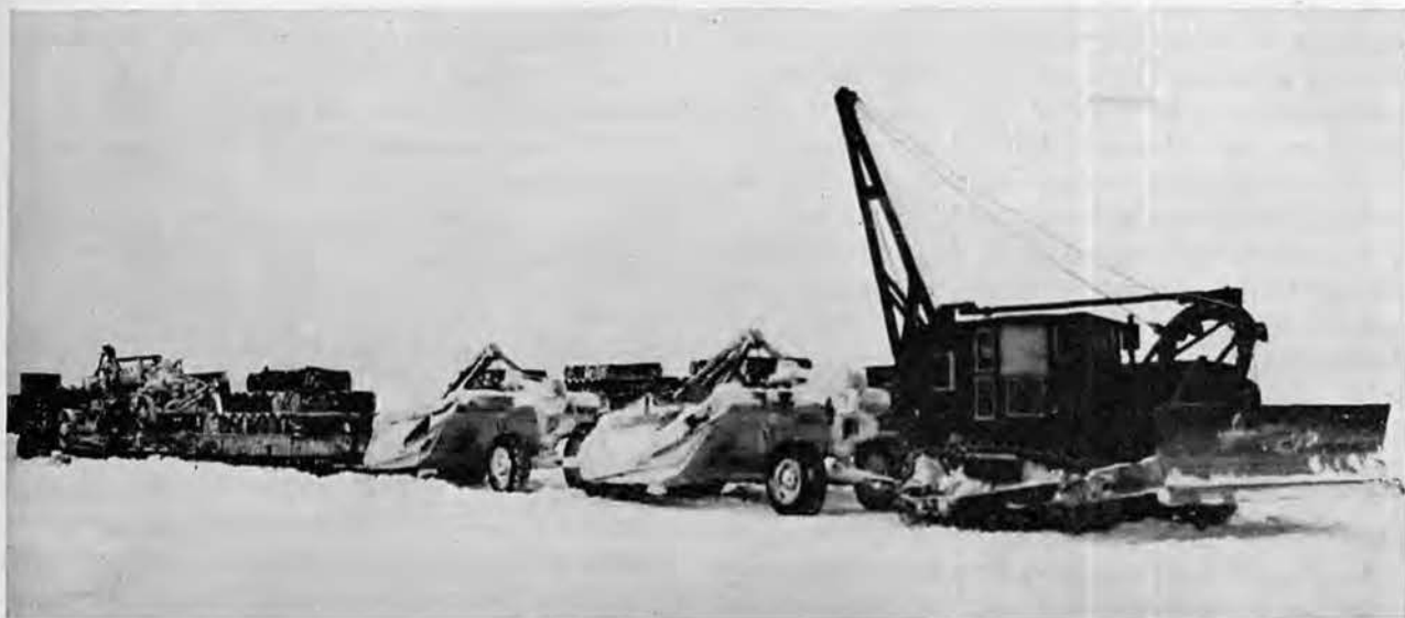
A POINT BARROW SUPPLY TRAIN Seabees use a D-8 to haul supplies to Umiat, February 1945
