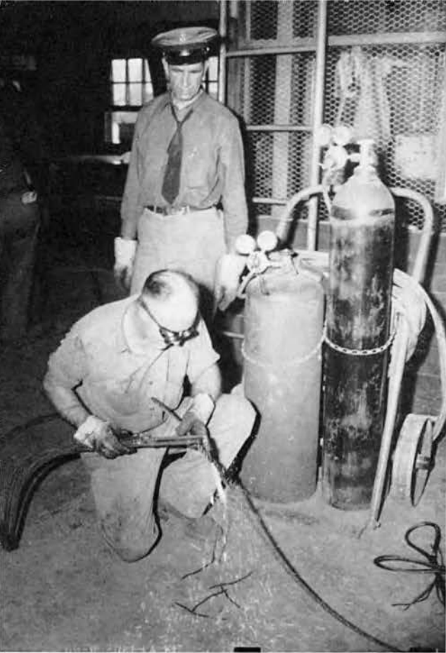
The Rigging School operates a shop for practice and instruction. Man shown in the picture above is welding a splice.
