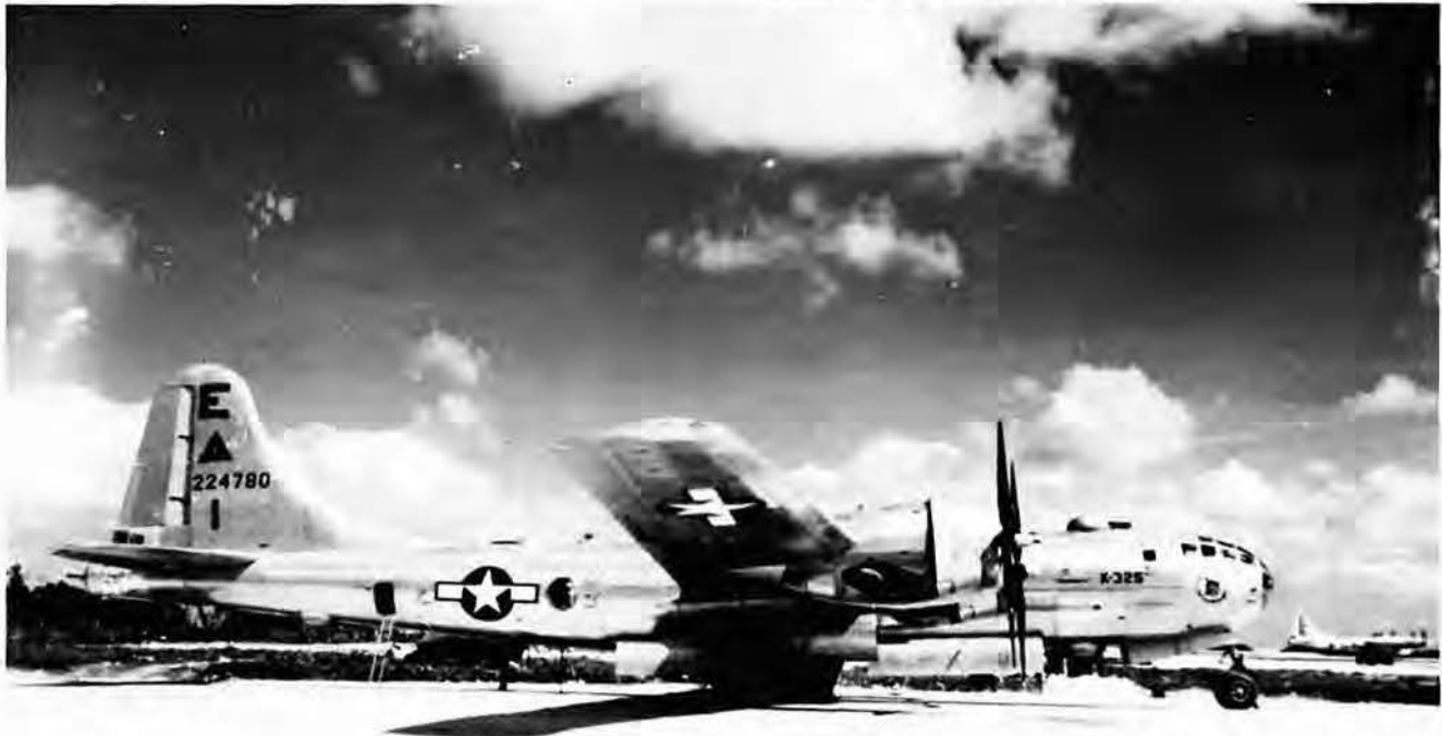
B-29 parked on one of Tinian’s hardstands. This B-29 carried a full armament load, dating the picture prior to General LeMay’s July 1945 switch to low-level incendiary bombing attacks. The B-29’s were stripped of their normal armament except for tail guns, to save weight, and increase bomb load. Photo, Elmer F. Goodwin.
