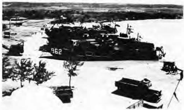
135th's equipment is landed on the beach. Landing Craft Tanks (LCT's) grounded on the beach as cargo is moved from the LST's and ships to the shore. Crane is located in front of LCT's to off-load heavy equipment onto open bed trucks from movement inland. Photo, Lloyd Ringrose.
