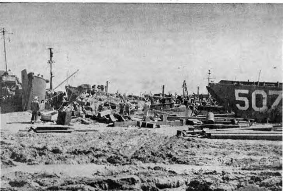
The landing craft weathered the typhoon better than any of the other vessels. They were built for shallow water.
