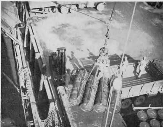
Two Tons a Draft, Forty Tons an Hour With a Chine Hookup
