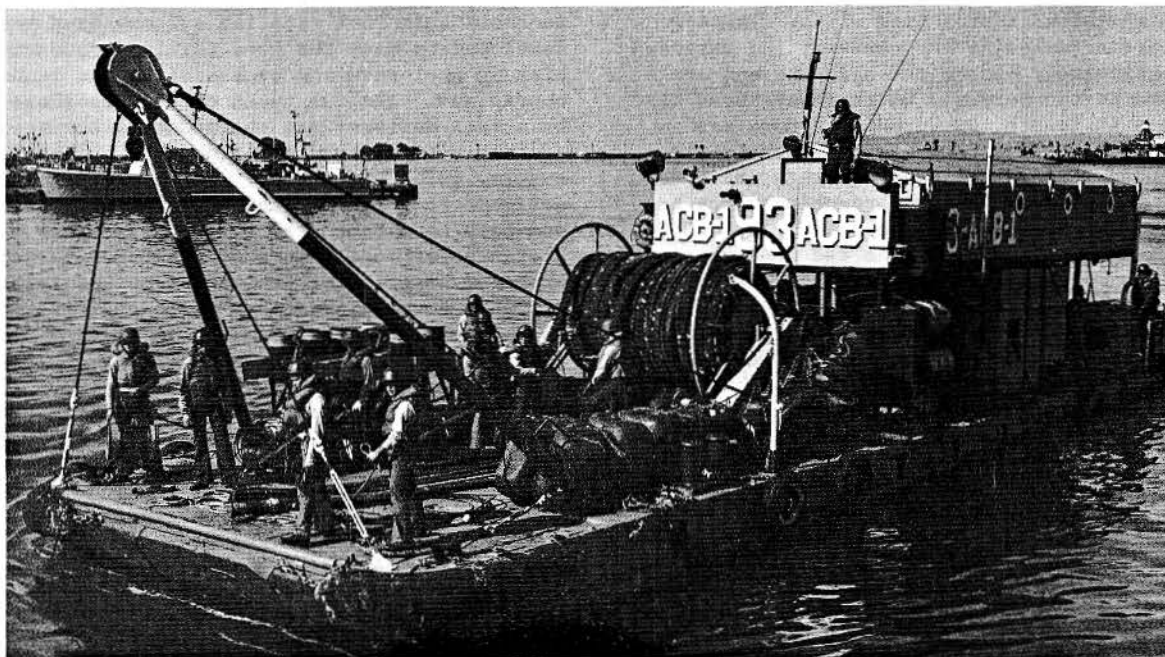
FIGURE 54 BUOYANT FUEL SYSTEM
