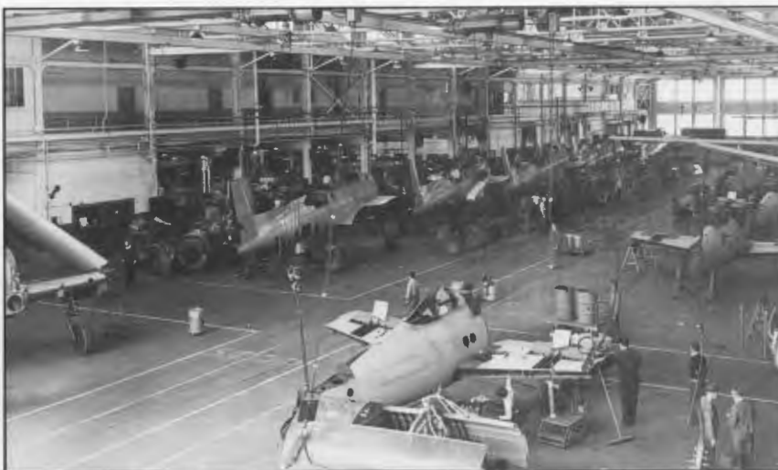
Fuselages from Grumman TBM Avenger torpedo bomber/minelayer undergoing overhaul at NADEP, Norfolk's fuselage repair facility inside Building V-28 (March 1950 U.S. Navy photo)
