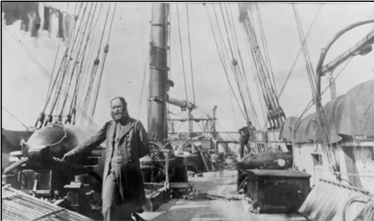
Figure 7. Historic photograph illustrating a Fawcett, Preston & Co. 32-pounder, an ordnance chest and the tangent sight on the breech of the stern pivot gun of the CSS Alabama .
