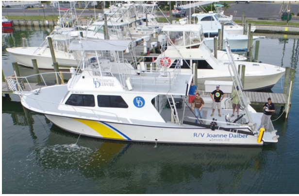
Figure 17. University of Delaware Research Vessel Joanne Daiber with the Edgetech 6205 sensor suspended over the water off the vessel's port quarter. (Image courtesy of the University of Delaware.)
