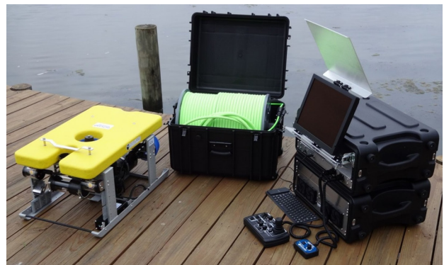
Figure 19. Outland 1000 Remotely Operated Vehicle similar to the one to be utilized by University of Delaware in the investigation of the USS San Diego wreck site. (Image courtesy of Outland.)
