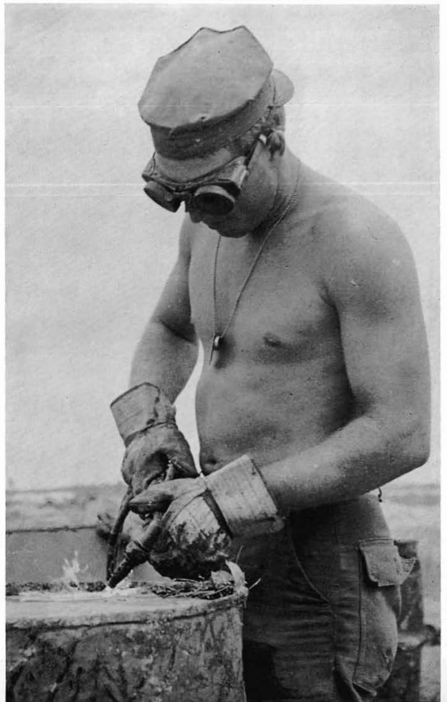
SWF3 McMINN utilizes a cutting torch to remove the lid off a 55 gallon drum.
