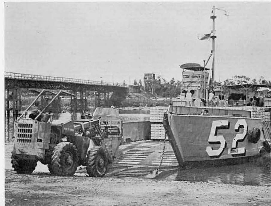
A rough terrain forklift unloads a LCU at the Dong-Ha Ramp on the Song Hieu Giang River.
