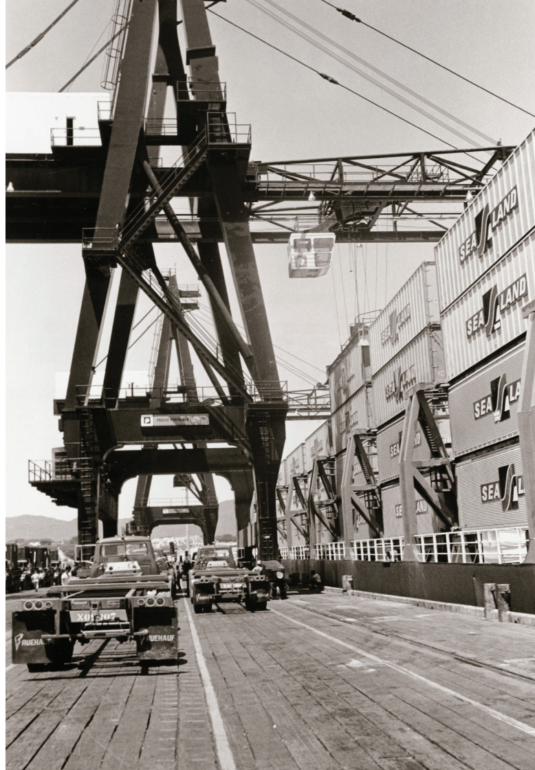
In July 1968, Sealand trailer trucks line up to receive one of 609 vans carried by the transport vessel, each of which can carry 20 tons of cargo. ( Journalist 1st Class Joseph D. Sheets/ Naval History and Heritage Command image )
