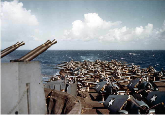
USS Essex (CV-9): Scene on the flight deck, looking aft from the carrier's island during her shakedown cruise, 20 March 1943. Planes parked on deck are F6F-3 Hellcat fighters (in foreground, with wings folded) and SBD-4 Dauntless scout/dive bombers (80-G-K-698).
