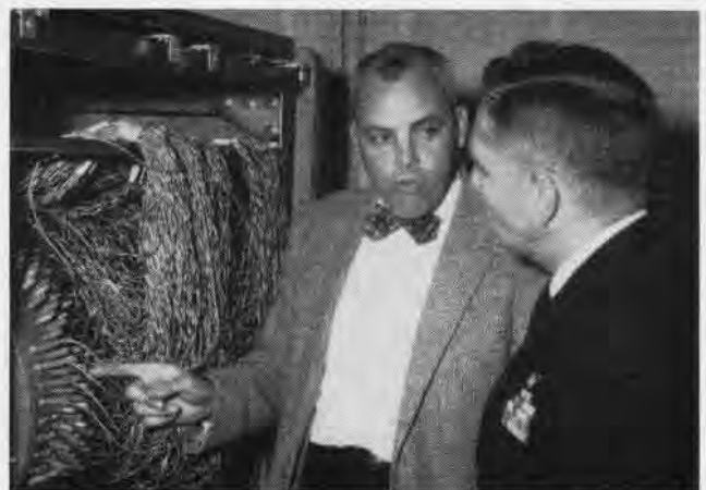
STANLEY KINGHAM , Senior Air Traffic Controller, N. Y. ARTCC, tells how UNIVAC "memory drum" stores essential air traffic information.
