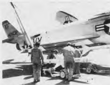
NAVY CREWMEN on the USS Midway (CVA-41) load Sparrow III missiles on Navy fighter.
