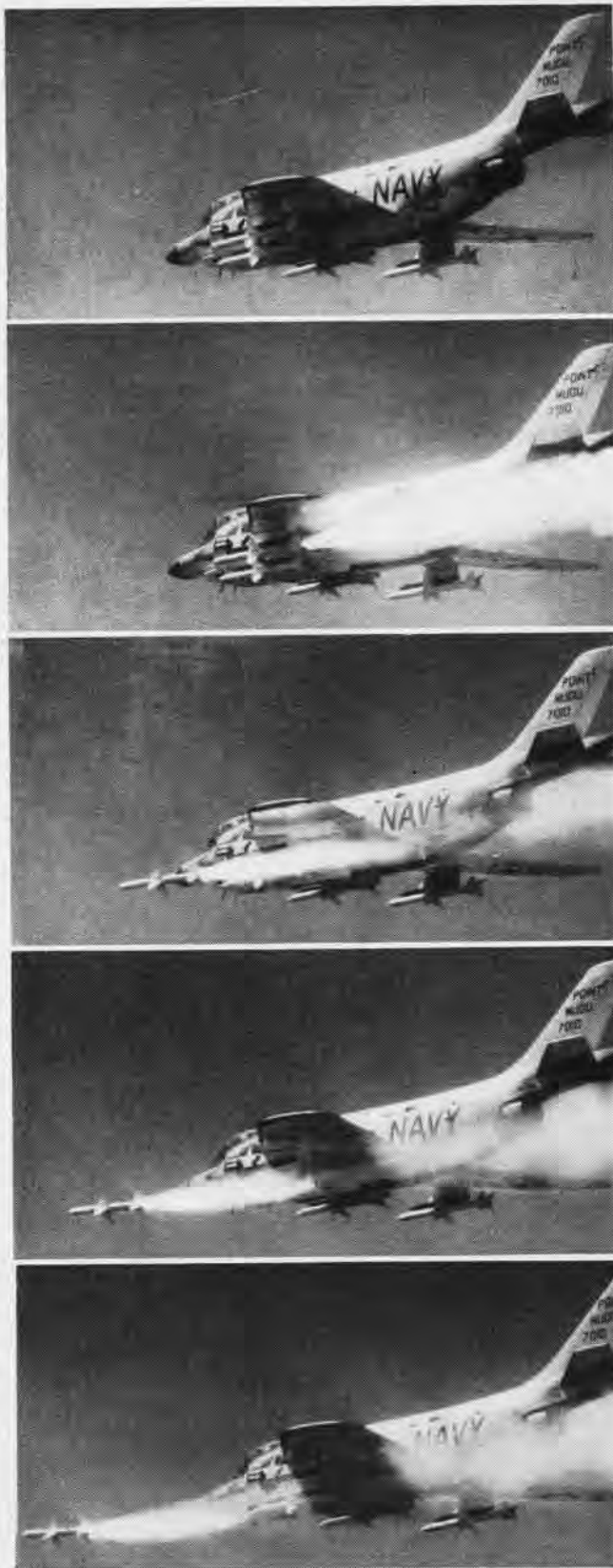
THESE UNUSUAL PICTURES depict, instant by instant, the launching of a Raytheon Sparrow III missile, its progress from the moment of launch until it reaches a point just ahead of the Demon aircraft.
