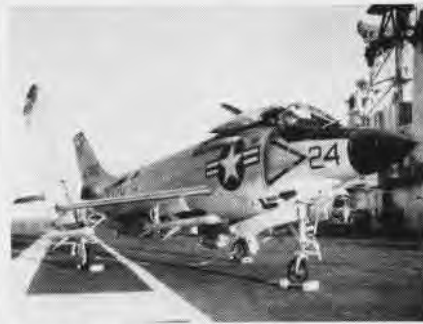
CLOSE-UP of the new missiles, mounted and ready on the McDonnell F3H Demon fighter.
