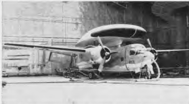
NESTLED in a corner of the vast climatic hangar at Eglin AF Base is this WF-2 Tracer as it went through climate qualifications in 1950's.
