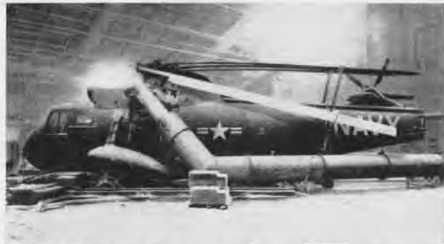
DUCTING CARRIES the jet exhaust from the twin T-58's of this HSS-2 out of the hangar as starting and other tests are run at -70 degrees.
