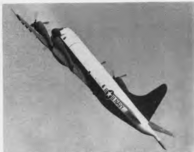
ORION COMING UP! This husky new ASW P3V-1 is due to become operational this summer. Most powerful submarine hunter in U.S. Naval Aviation history, its prime mission will be to seek out and sink enemy submarines. Carrying a 10-man crew at level-flight top speeds of 450 mph, they will first supplement, then replace, older P2V models.
