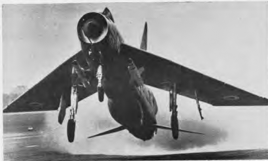
ENGLISH ELECTRIC LIGHTNING IS POWERED BY TWO ROLLS ROYCE AVON TURBOJET'S
