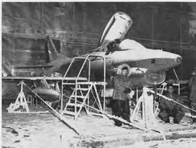
NATO STRIKE fighter, Fiat G-91, undergoing climate testing in mid-1961. Changes based on tests will be incorporated in production models.
