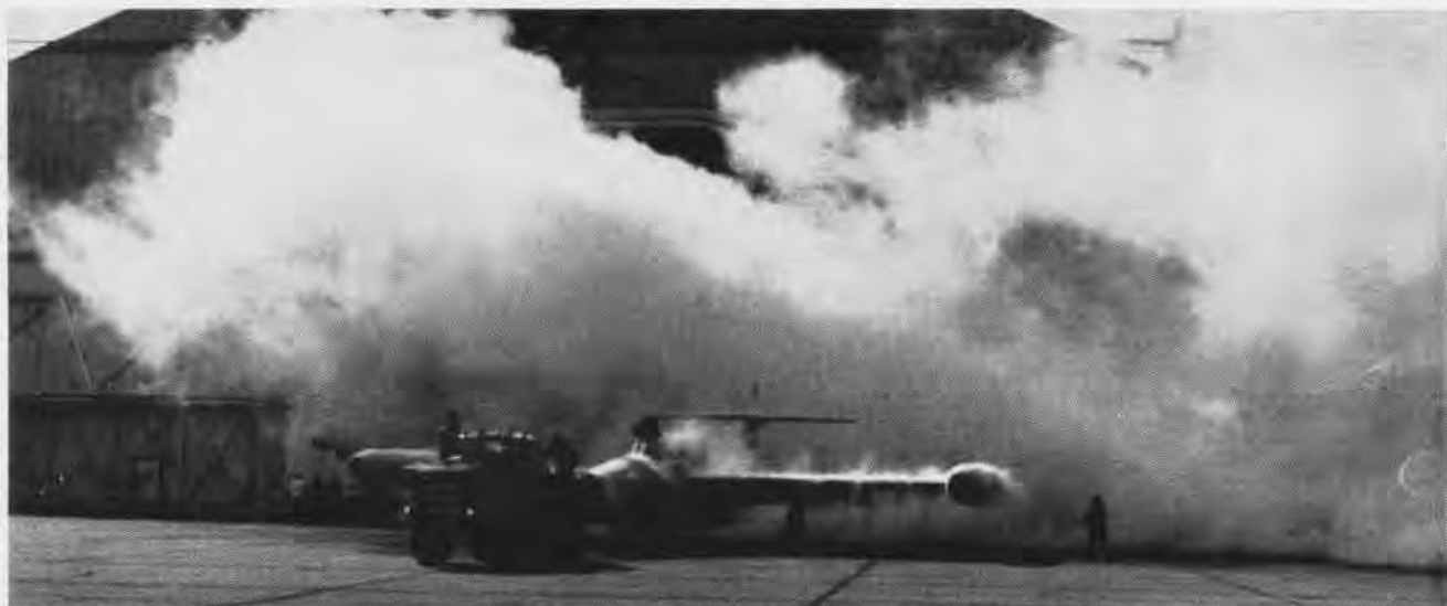
COLD-SOAKED for 72 hours at minus 65° F., this F-89 was towed into sunshine and started. It climbed to 30,000 feet for armament system
