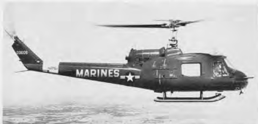
A NEW ASSAULT support helicopter, turbine-powered with 1100 hp, is to be built for the Marine Corps by Textron's Bell Helicopter Co. Specifications include a payload of 800 lbs., 50 nautical miles radius of operation and a minimum cruising speed of 85 kts. Basically it will be the HU-1B Iroquois which set six world records in 1960. The helicopter will be used for observation target acquisition, reconnaissance, command control and casualty evacuation.
