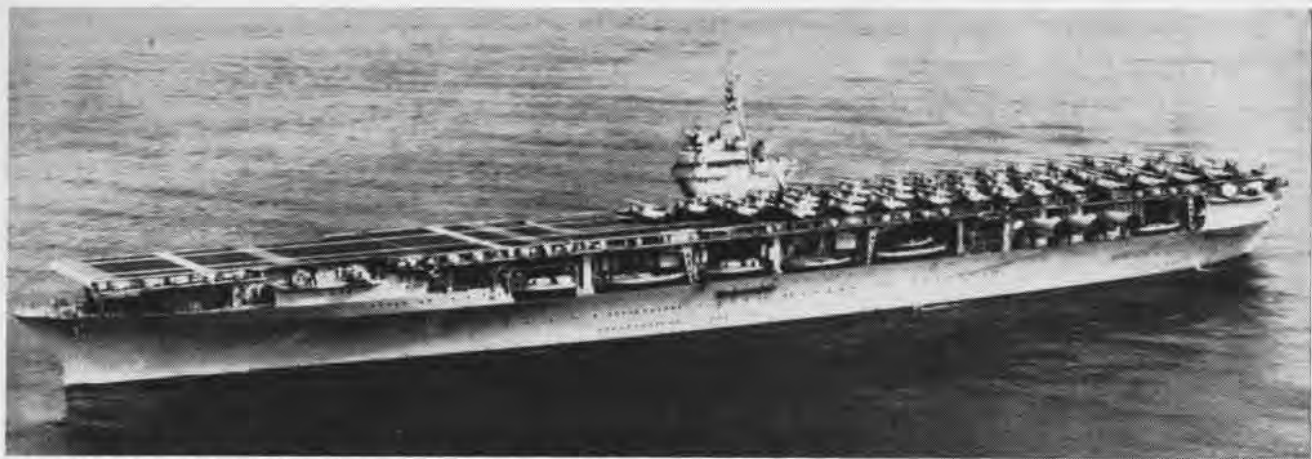
OPERATING WITH THE FLEET , USS Ranger had a 14,500-ton displacement. Unusual features were bow arresting gear, small island, stacks at stern. On deck are parked Vought scout bombers, Grumman fighters, Martin dive bombers in 1937 view. Capt. A.L. Bristol was first C.O.
