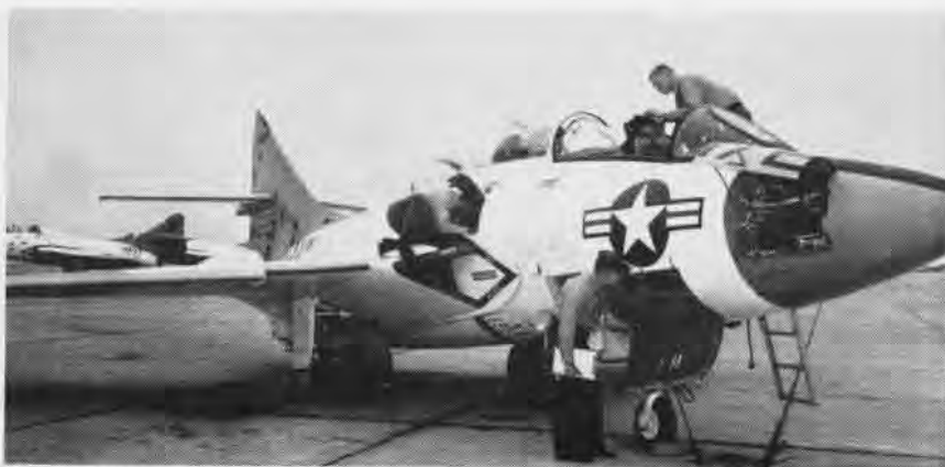
LEAVE NOTHING TO CHANCE. Four-man pre-flight crew checks every detail of VT-22 F9F-8T prior to clearing the aircraft for student flights. (Fourth man is under the wing at left.)
