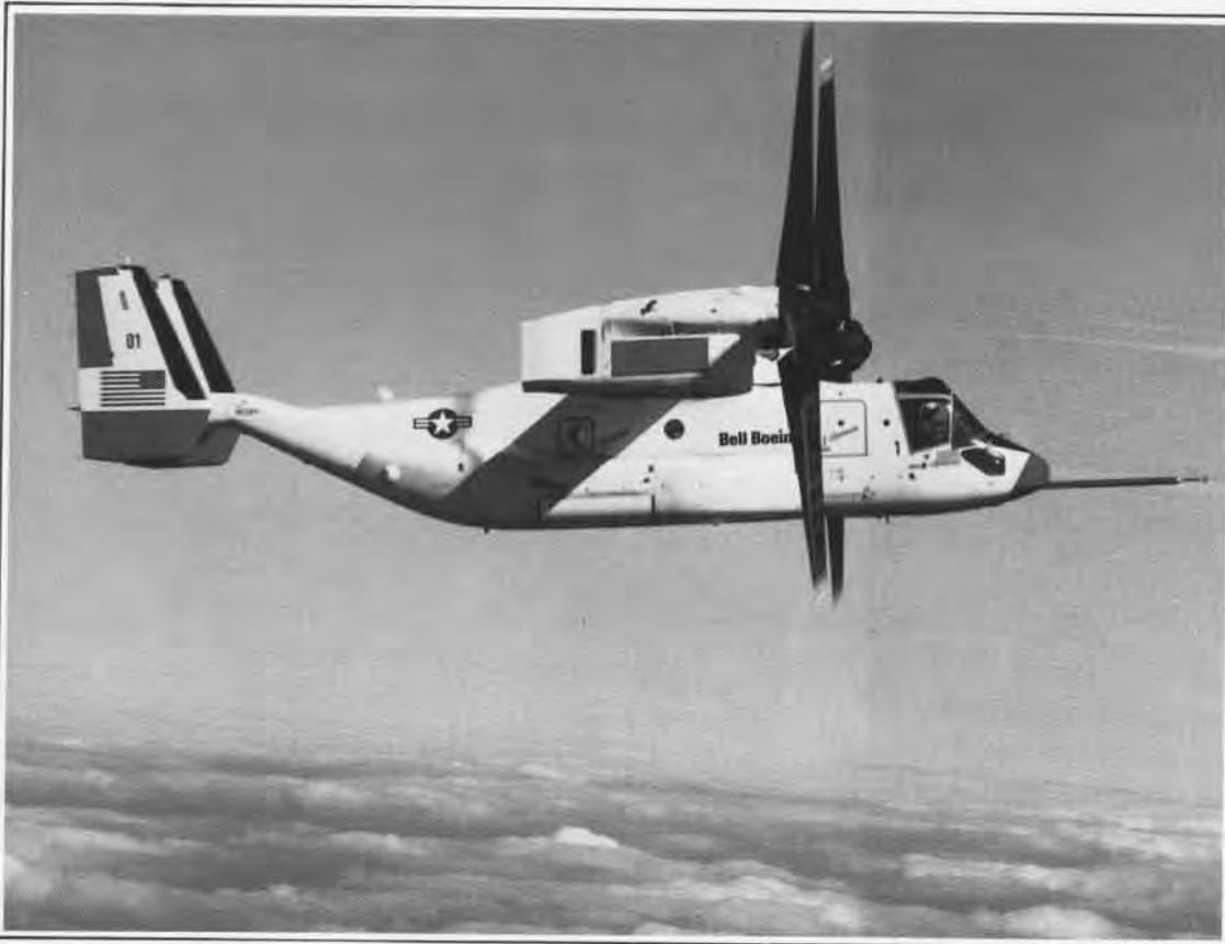
Left, on September 14, the V-22 Osprey tilt-rotor aircraft achieved full in-flight conversion from helicopter mode to airplane mode. The conversion is accomplished by rotating the engine nacelles and propellers from 90 degrees (vertical) through zero degrees (horizontal). During this tilting of the 38-foot-diameter propellers, the airplane's forward-swept wings progressively generate more lift, and the propellers function increasingly like propellers and less like helicopter rotors.
