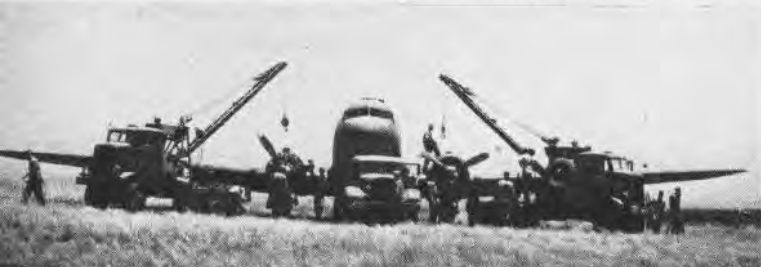
CRANE CRASH TRACTORS LIFT BELLIED PLANE TO LOW-BODY TRAILER
