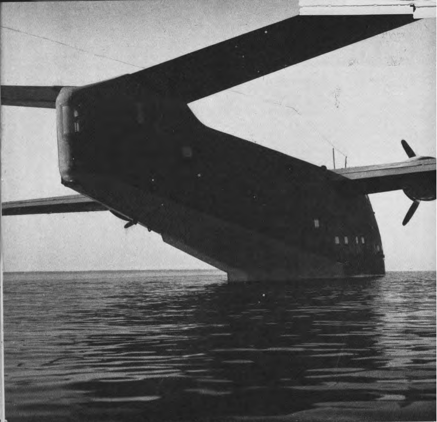
MODERN VERSION OF NOAH'S ARK, THE PB2Y COVERS AIR SEAS FOR NATS. IT HAS USEFUL LOAD OF 27,000 LBS., MAXIMUM RANGE OF 3700 MILES
