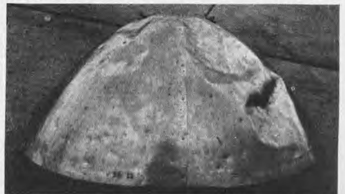
NOSE OF SAME PLANE SHOWS IMPACT OF HAILSTONES DURING FLIGHT
