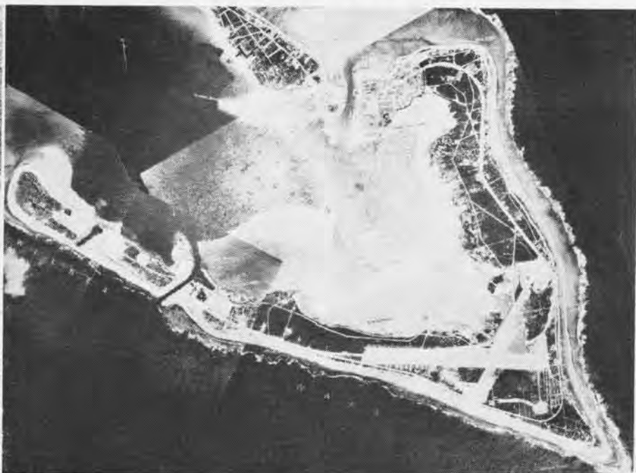
MOSAICS combine vertical photos to compose aerial map of enemy territory showing all features of defensive installations. This mosaic of Wake Island required several passes over the area from constant altitude and with proper spacing between each flight
