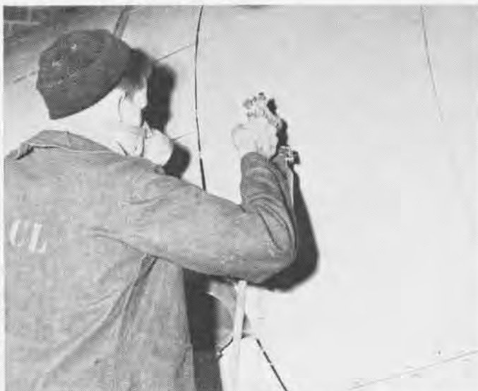
5 PAINT scheme then applied to aircraft for more tests after scheme is tried out on paper and on models
