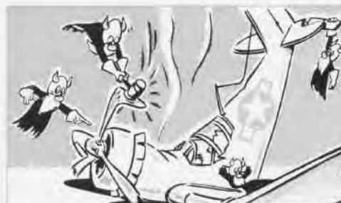
18 Don't land with your wing de-icers on. They will act as "spoilers."
