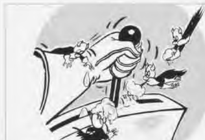
20 Before approaching for a landing, make sure ice is not jamming the carburetor butterfly valve. Test by moving your throttle back and forth several times.
