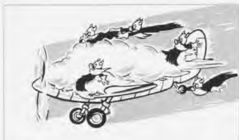
17 Don't attempt a three-point landing when you are loaded with ice. Fly in under power.
