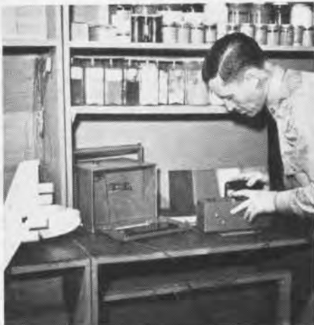
3 REFLECTION power of paint surface is measured by this device
