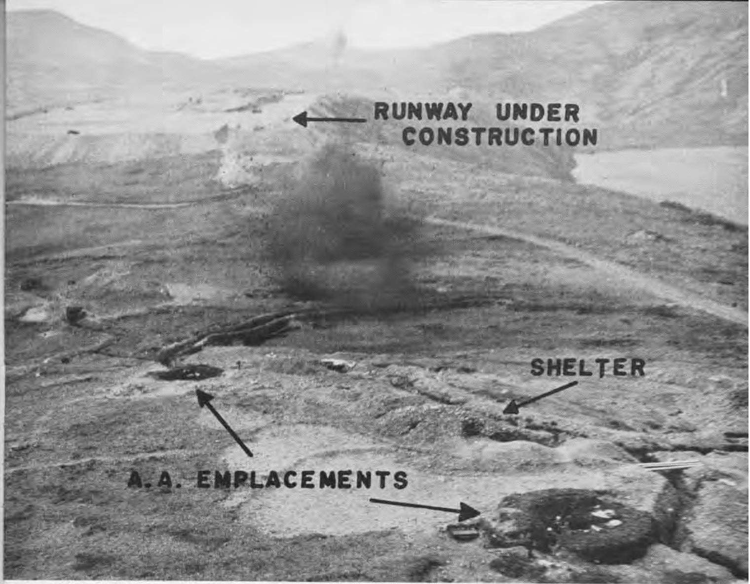
DICER SHOTS of Jap installations on Kiska gave photo interpreters pre-invasion close-up of construction activity, types of guns and other vital information. An overlapping series of low obliques may be joined together to present a panoramic view of special areas
