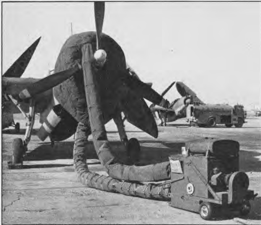
INSULATED AIRCRAFT ENGINE COVER HELPS WARM UP AIR-COOLED ENGINES IN COLD COUNTRIES
