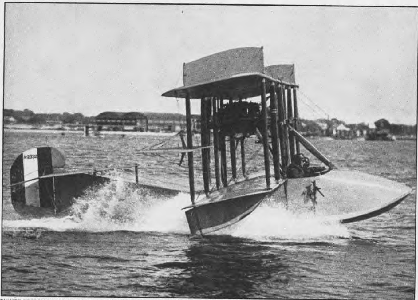
PUSHER PROPELLOR, SKID FINS AND ELONGATED STABILIZER FEATURE THIS NAVY F-BOAT USED AT PENSACOLA TO TRAIN EMBRYO BOMBERS BACK IN 1918
