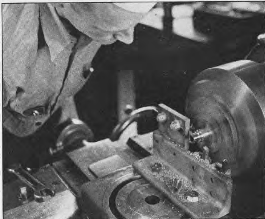
DALLAS A & R SHOP DEVELOPS A NEW TYPE FIXTURE TO SPEED UP MAKING OF SUN GEAR BUSHINGS
