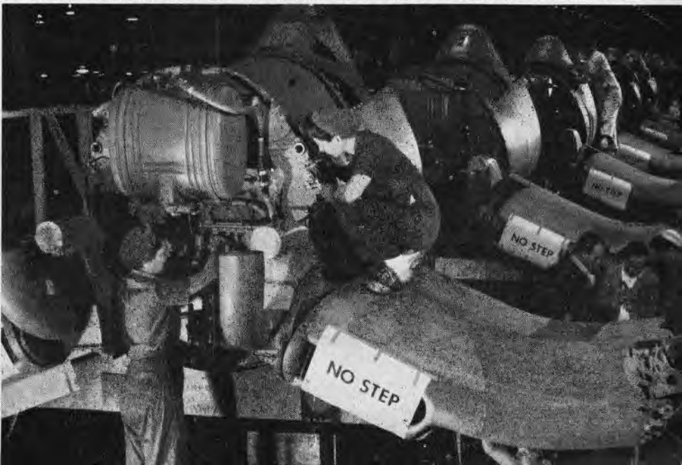
SERVICE PERSONNEL MAKE THE FINAL CHECK OF THE PLANE BEFORE ITS FLY-AWAY TO THE NAVY WOMEN ARE ASSEMBLING OIL TANKS AND AIR DUCTS ON THE CENTER SECTION OF THE NEW PLANE
