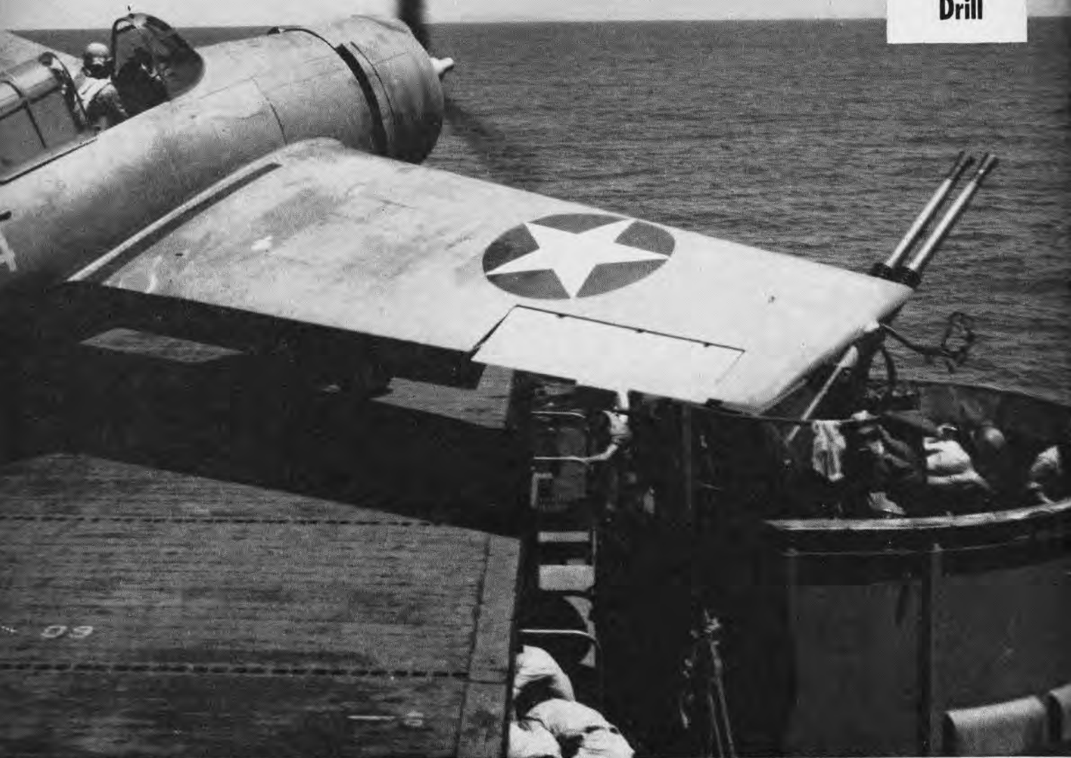
THOUGH A PLANE USUALLY GROUNDLOOPS TO THE LEFT, THIS ONE SWERVED TO THE RIGHT, SENDING CRAFT OVER STARBOARD SIDE, THUS HITTING GUNS
