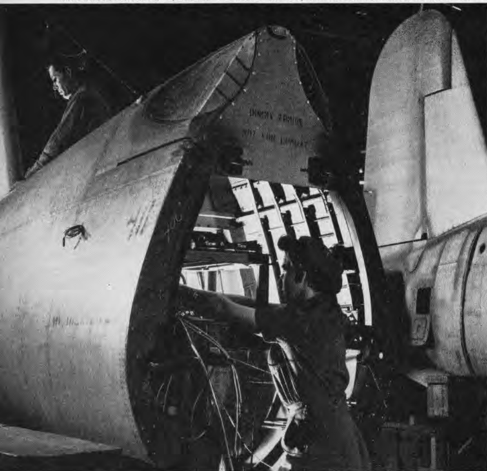
SERVICE CHECK-UP ON THE WING FOLDING MECHANISM IS BEING MADE BEFORE TEST FLIGHT GIRL INSTALLS RADIO EQUIPMENT IN AFTER SECTION, WHILE THE MAN TESTS RIGIDITY OF FIN
