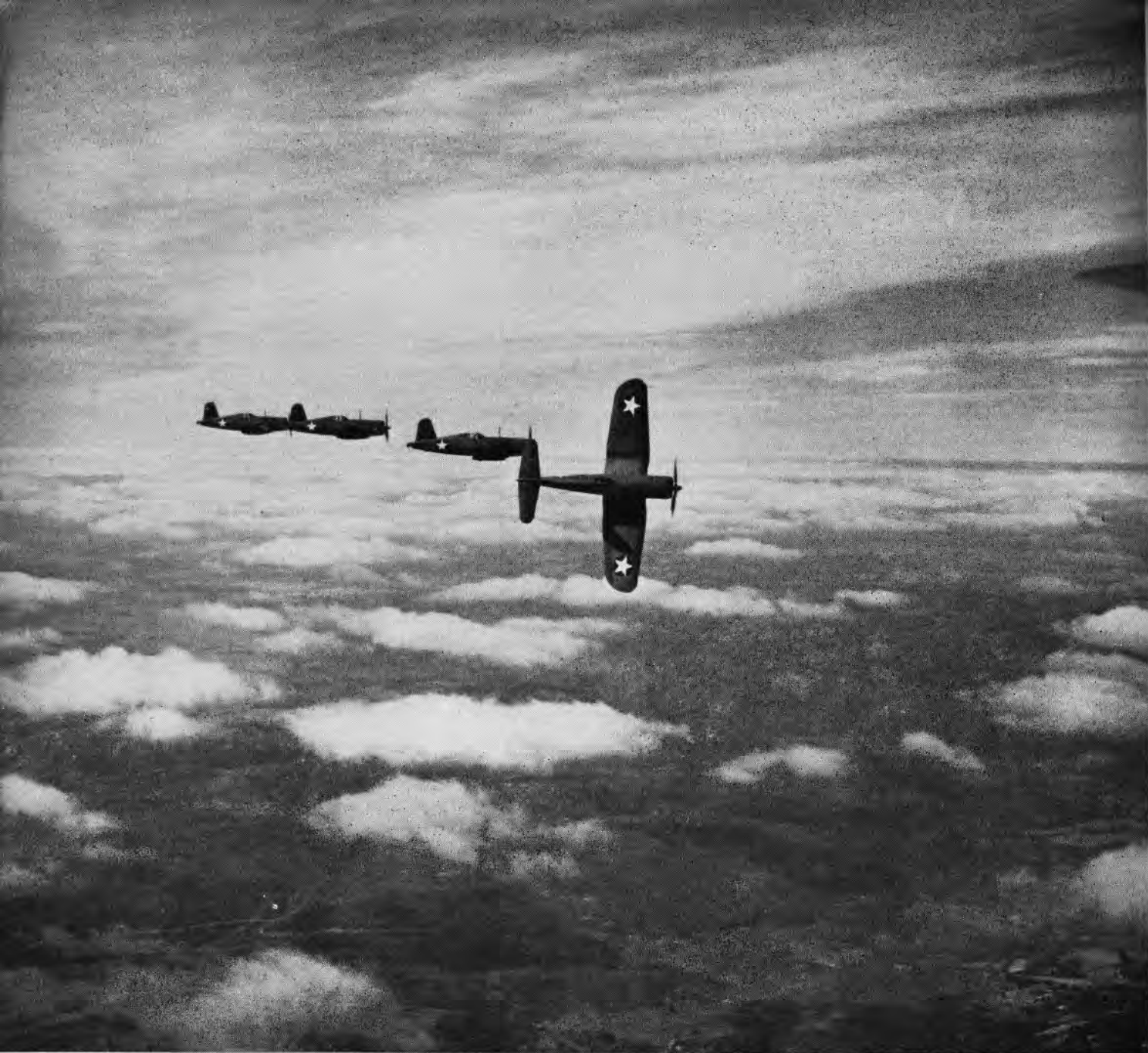
THE F4U, ALL-AROUND STURDY FIGHTER, HAS HIGH TOP SPEED, GOOD RATE OF CLIMB, EXCELLENT DIVING CHARACTERISTICS AND GOOD AILERON CONTROL
