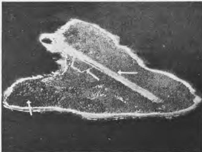
Typical development of Jap airfield in coconut plantation on small island. Only runway and small taxi strip have been developed, and no clearings as yet have been made for AA positions. Trees effectively camouflage stores, personnel, activity
