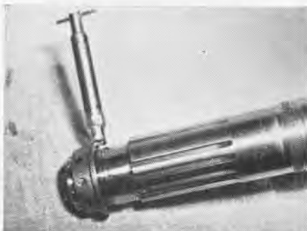
TOOL SIMPLIFIES CRANKSHAFT THREAD CUTTING
