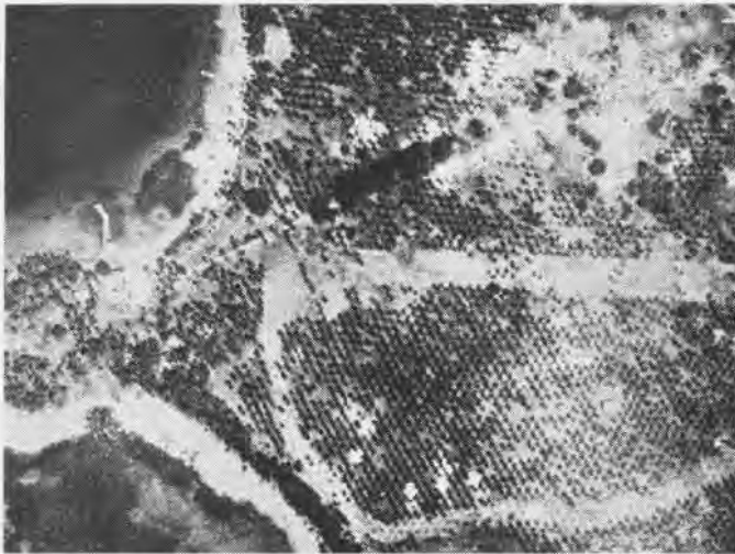
Naval air photography records development of typical Japanese airfield in a coconut grove. Plantation buildings and pier facilities are visible. Runway and taxi strips come into sight as Japs begin to remove trees. Four fighter revetments are in progress
