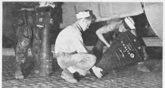
Crew of Liberator used as photographic plane loads a K-18 aerial camera into bomb bay racks; plane's first photographer checks flight log by recording camera, film numbers
