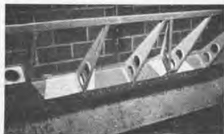
SPAR-SPLICE IDEA SPEEDS AILERON REPAIRS
