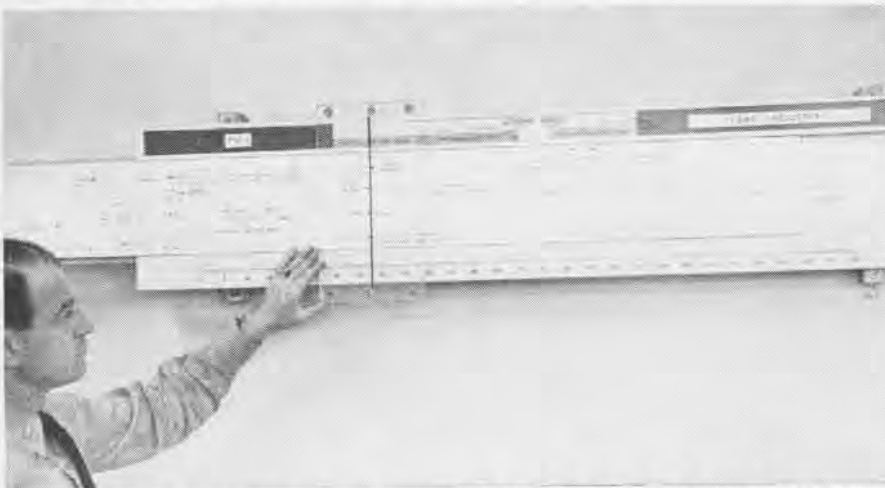
BUILT LIKE GIANT SLIDE RULE, PV-1 LOAD ADJUSTER CAN BE ADAPTED TO OTHER PLANE TYPES
