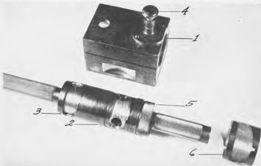
1. BODY, 2. CAM SHAFT, 3. MASTER CAM, 4. GUIDE PIN, 5. CLAMPING NUT, AND 6. FINISHED CAM
