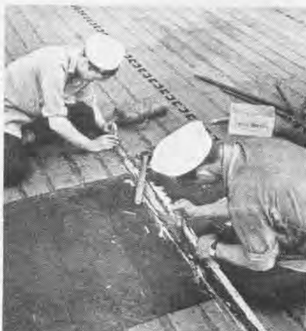
Ship's carpenters calk oakum in deck of carrier to repair damage to wood planks
