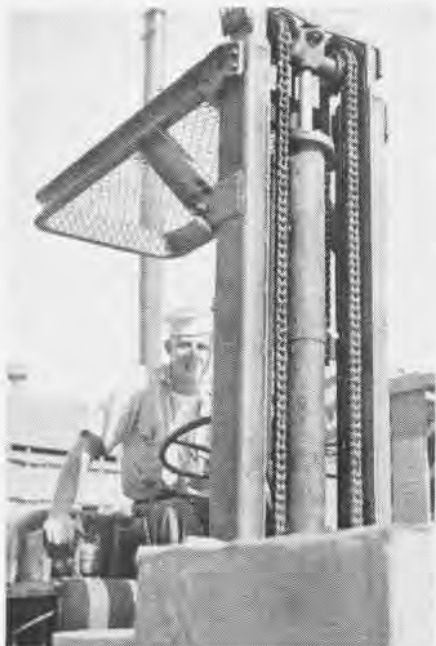
FRAME PROTECTS WORKER ON FORK TRUCK LIFT
