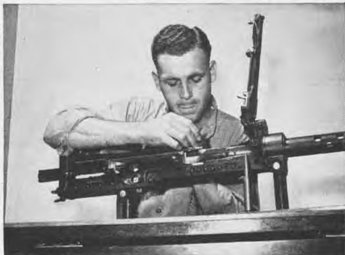
Stripping a .50 cal. machine gun and assembling it in short order is one of the things Adams learns at the Jacksonville technical training center along with his radio work. An aerial gunner must be able to fix a jammed gun quickly if a battle is being fought
