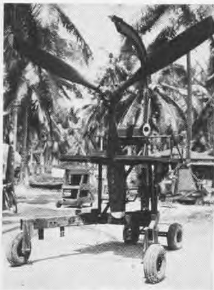
PROP IS CARRIED ON CART IN THIS POSITION
