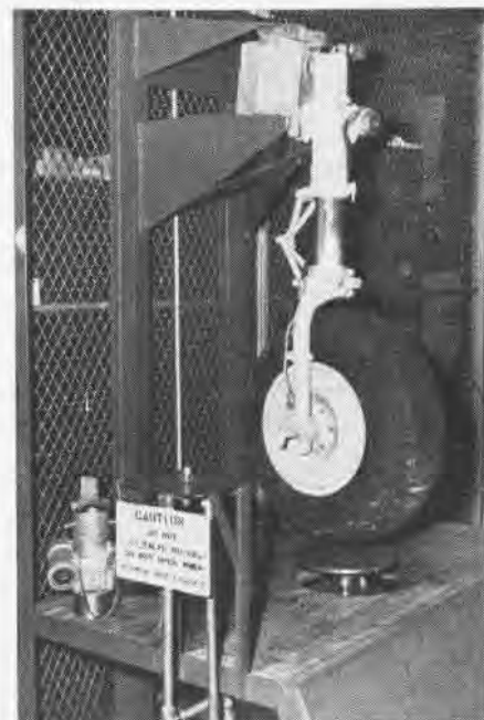
DEVICE TESTS LANDING GEAR PISTON LEAKAGES
