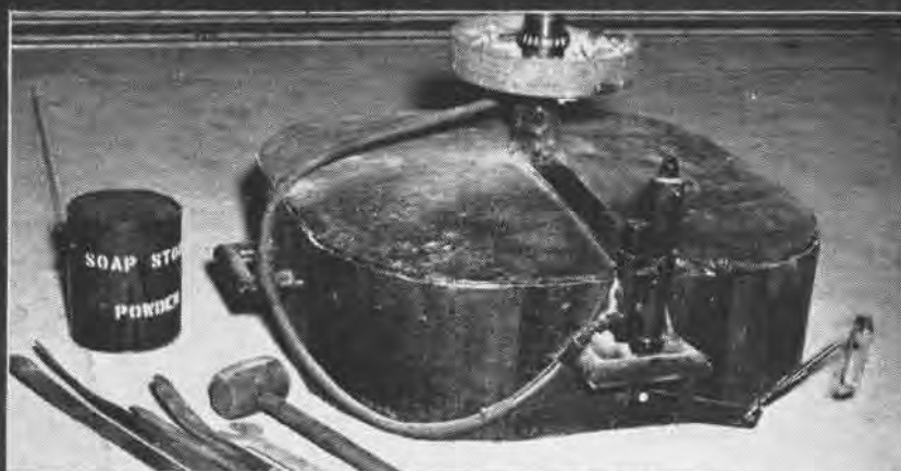
AN OLD AXLE TO HOLD WHEEL, PLUS ADEQUATE TOOLS, MAKES TIRE CHANGE SIMPLE
