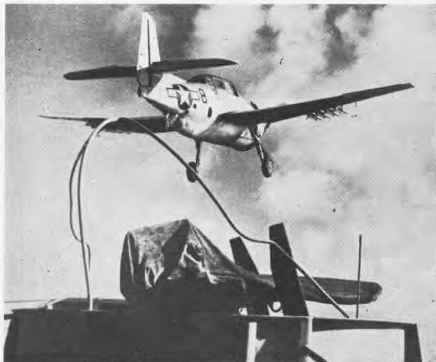
EIGHT ROCKETS NESTLE in their chutes underneath the wings of an Avenger as it soars out from the deck of a carrier in this first released picture showing rocket installations on a Navy plane. Armed with rockets, machine guns, bombs or torpedoes, the TBF becomes one of the toughest fighters in naval aviation. These new missiles have been used by American planes against U-boats in the Atlantic, and shipping in the Pacific.
