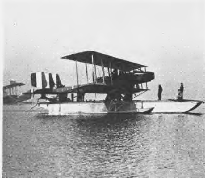
Sea sled traveling at full speed, plus the maximum rpm of a plane engine assured the successful take-off of the Caproni bomber
