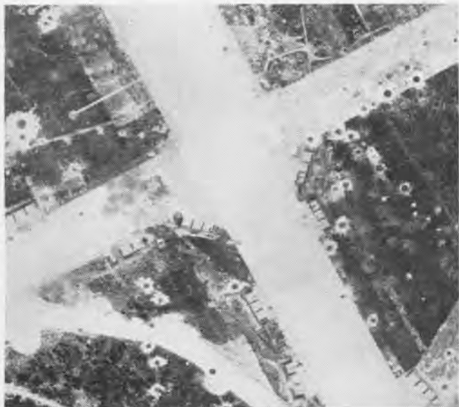
Planes parked in multiple revetments built adjacent to runway at Mili. Direct hits on shelters leave some sections undamaged
