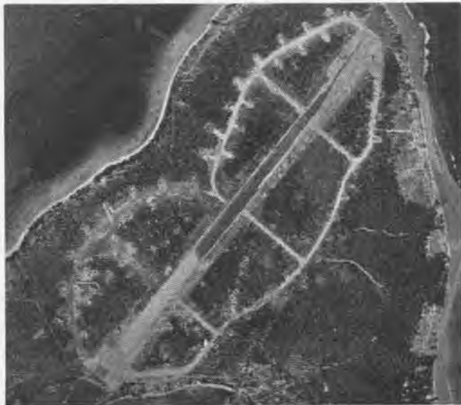
Jap airfield setup on small island shows use of protective covering of trees as camouflage for the widely dispersed plane shelters
