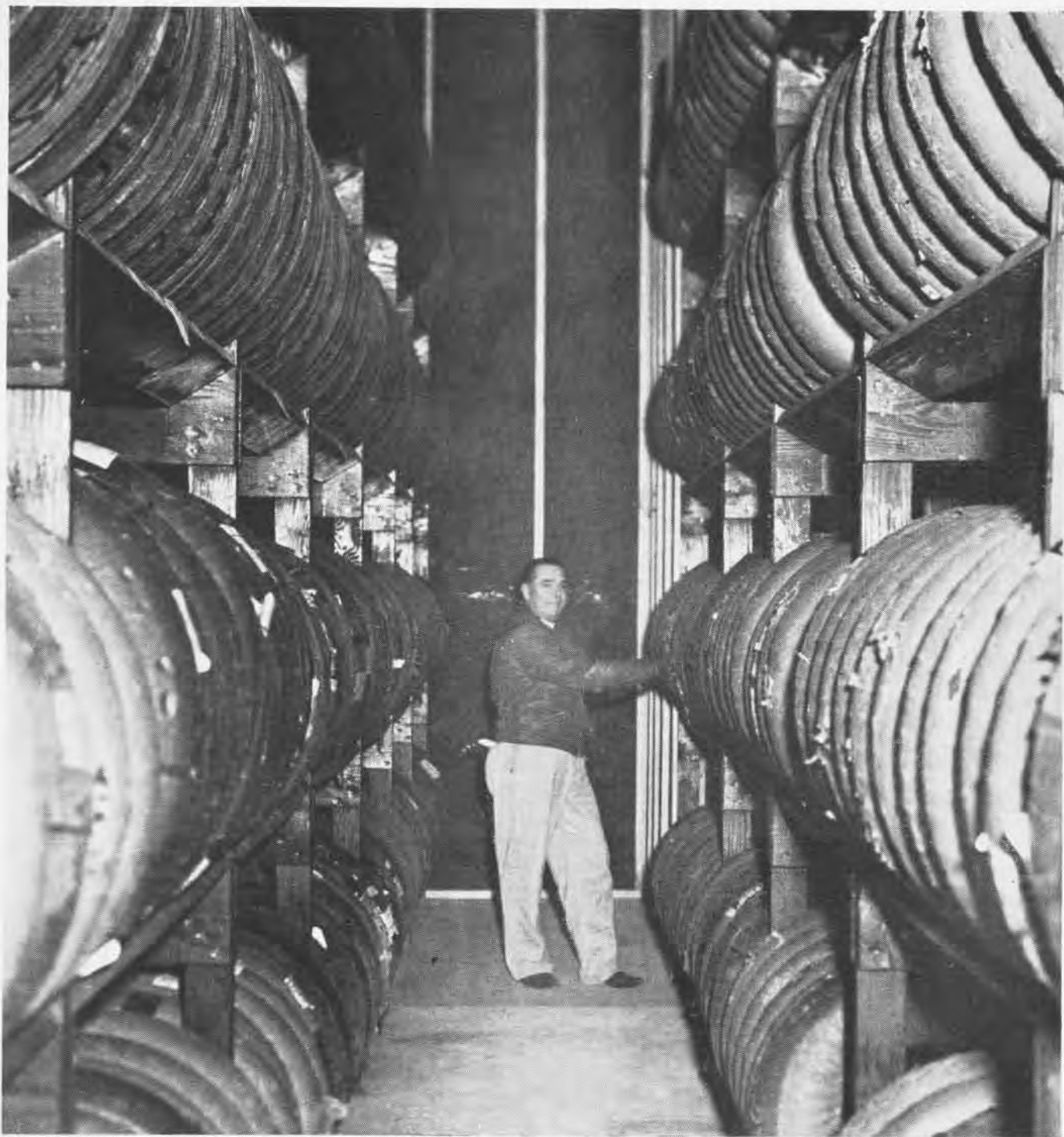
RUBBER CONSERVATION SHOULD START WHEN TIRES ARRIVE. PLACE IN UPRIGHT RACKS IN A DARK, DRY, COOL STORAGE ROOM, WITHOUT SQUEEZING
