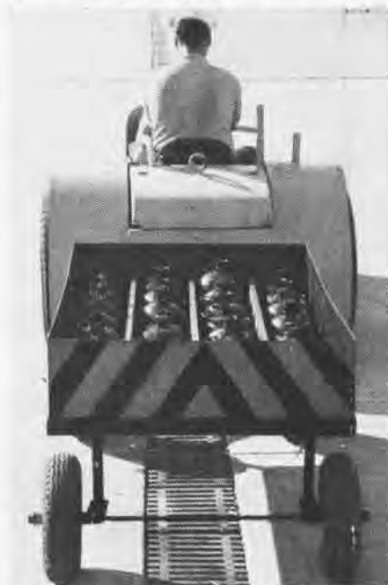
CART HOLDS POTS UPRIGHT, PREVENTS SPILLING
