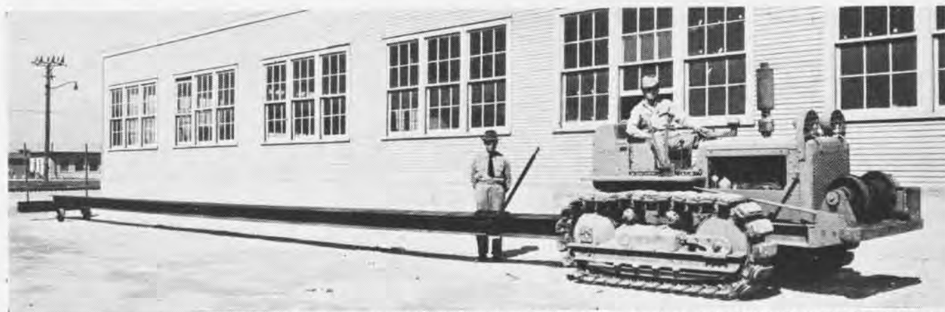
TRACTOR-DRIVEN SEAPLANE RAMP SCRAPER PAYS BIG DIVIDENDS BY REMOVING SHELLS FROM WATER-COVERED CONCRETE, WHERE TIRES MIGHT BE CUT
