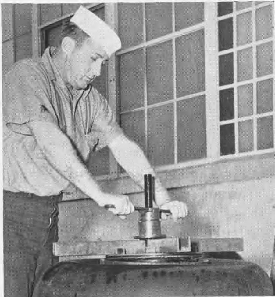
BEAD BREAKING PRESS REDUCES INJURY TO TIRES AND MAKES WORK EASIER FOR THE REPAIRMAN
