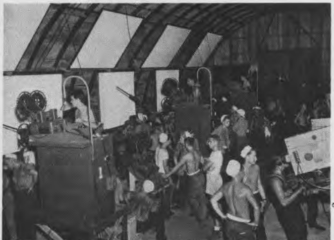
Both torpedo and dive bombing attack training are now available with 20 mm. guns using the Mk. 14 sight in Seabee hut
