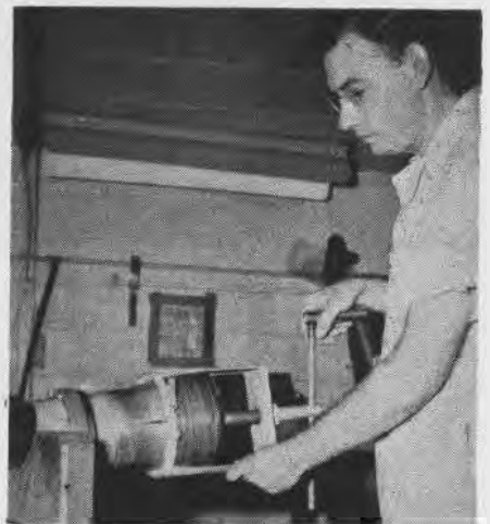
EMPLOYEE SHOWS JACK IN PLACE ON PROP HUB
