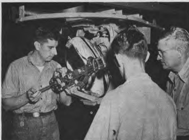
Highly polished reflector of huge searchlight shows intricate gear for positioning carbon arcs which generate tremendous candlepower
