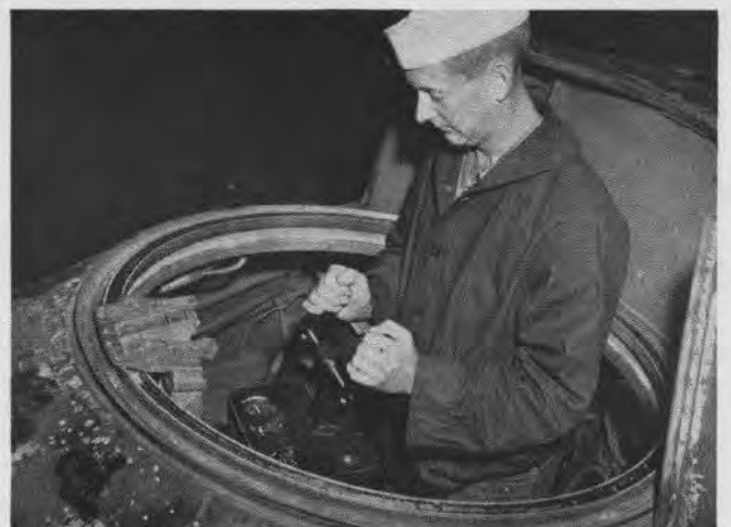
Gear installed in forward cockpit of Catalina enables aircrewman to track and train searchlight and pick out targets in the dark
