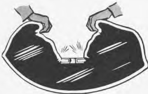
BENDING CELLS AT FITTINGS CAUSES BREAKS
