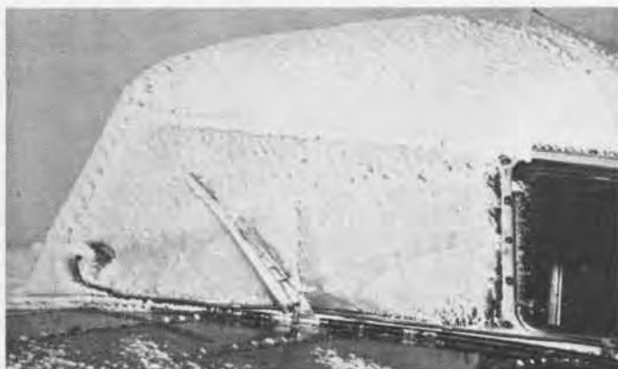
ALCOHOL formed a thin anti-freeze solution on small forward window on port side. Pilot removed ice sheet by hand from side
