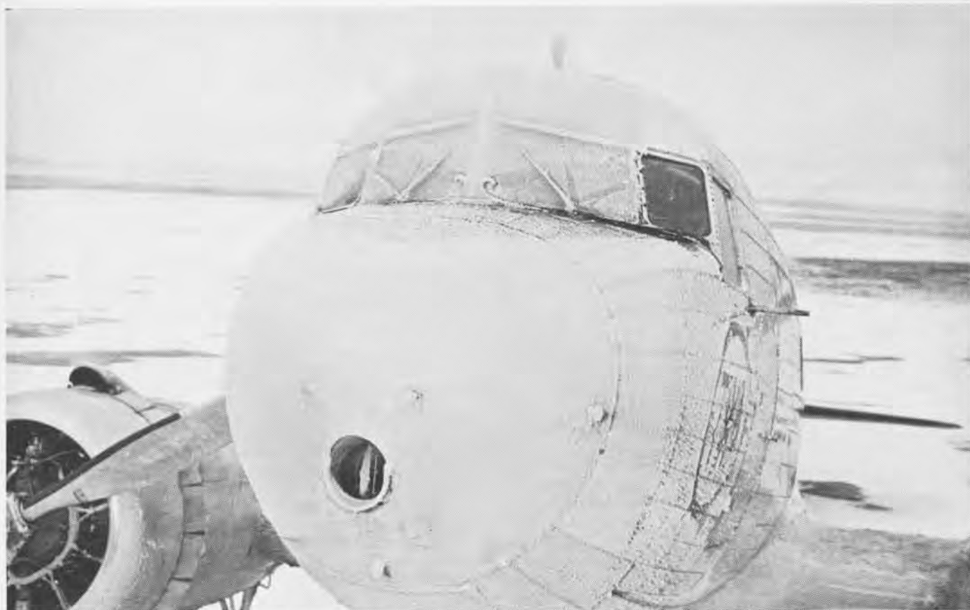
WINDSHIELD iced over completely. Pilot made no attempt to keep it clear with alcohol, choosing to conserve his supply for de-icing propeller. Some alcohol was used to keep small forward window on port side clear. Alcohol was put on glass when ice was encountered
