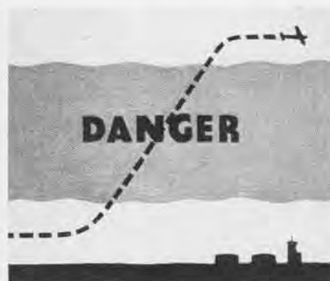
PILOT CLIMBS THROUGH DANGER AREA TO AVOID ICE GETS INTO ABOVE-FREEZING REGION AND LEVELS
