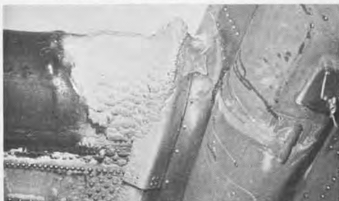
TENACIOUS and hard form of clear ice that coated leading edge proved tough job for de-icers. Ice was still on wing after landing
