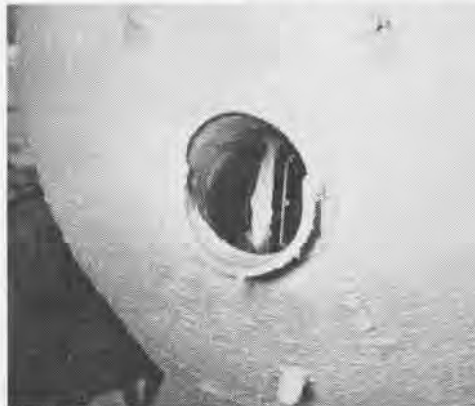
ICE RIMMED ventilation air scoop on nose fuselage. Maximum thickness was about 1/2 inch.
