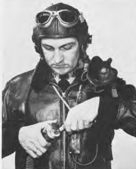
1 IMPROVED breathing tube coupling allows quick connecting, disconnecting
