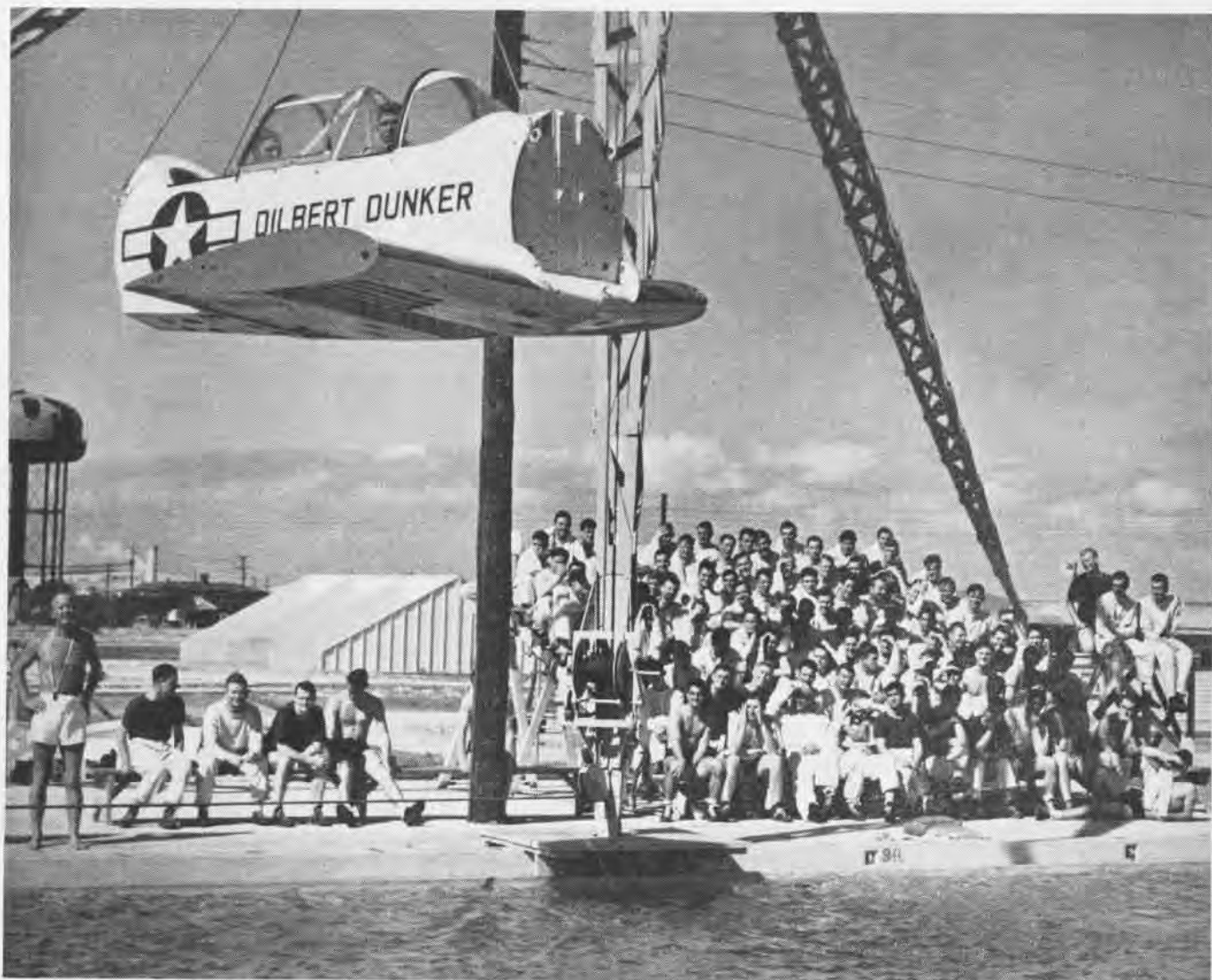
MECHANICAL "DILBERT DUNKER" IS PORTION OF PLANE FUSELAGE RIGGED UP TO SIMULATE WATER LANDING. TRAINING CREWS IN ESCAPE PROCEDURE
