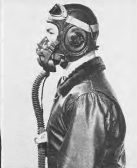
5 SUITABLE clearance between bridge of nose and mask is boon to wearer
