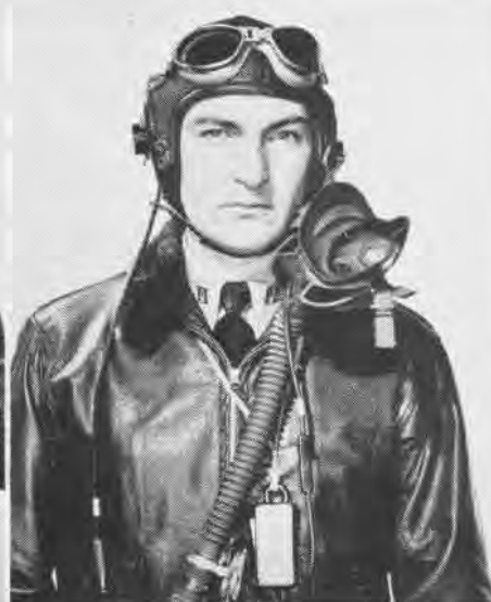
2 NORMAL position of mask prior to use of oxygen shows microphone in front
