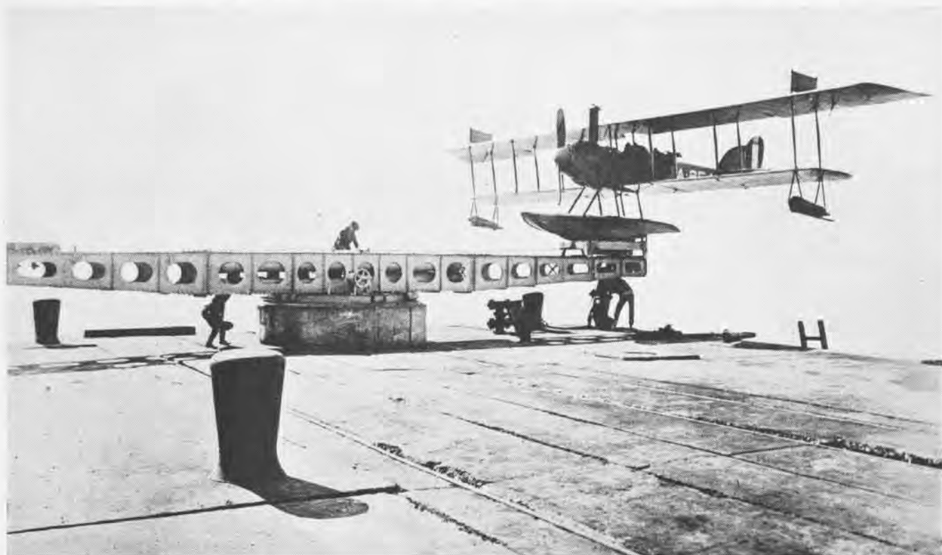
NAVY'S FIRST TURNTABLE CATAPULT, FORERUNNER OF PRESENT-DAY TYPES, WAS CONSTRUCTED AND INSTALLED ON U.S.S. MARYLAND IN 1921
