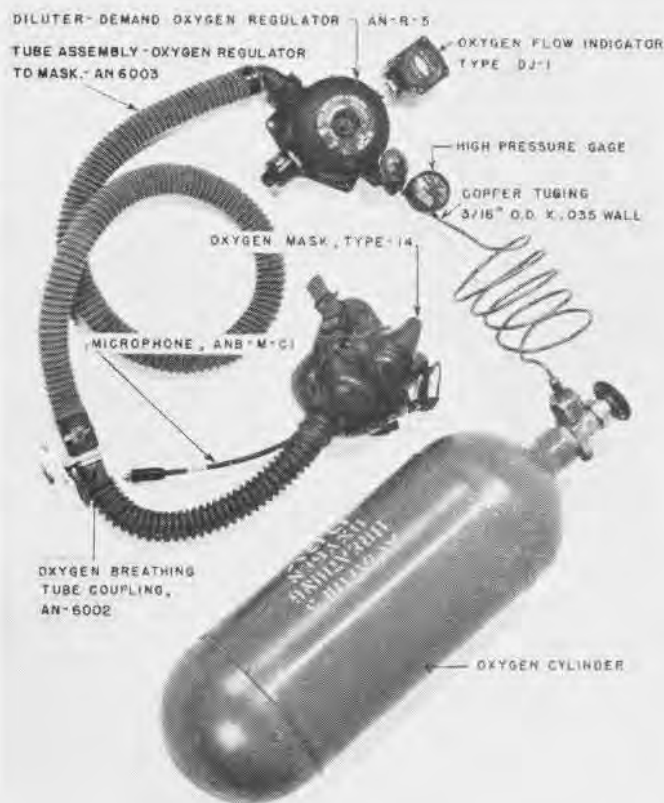
INSTALLATION OF MICROPHONE IN TYPE-14 MASK IS READILY ACHIEVED. DILUTER-DEMAND REGULATOR ASSEMBLY WILL BE AVAILABLE SHORTLY.
