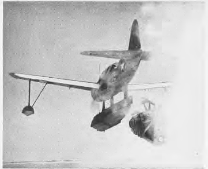
Cadets in observation scout training practice catapult take-offs in preparation for battleship, destroyer or seaplane tender duty
