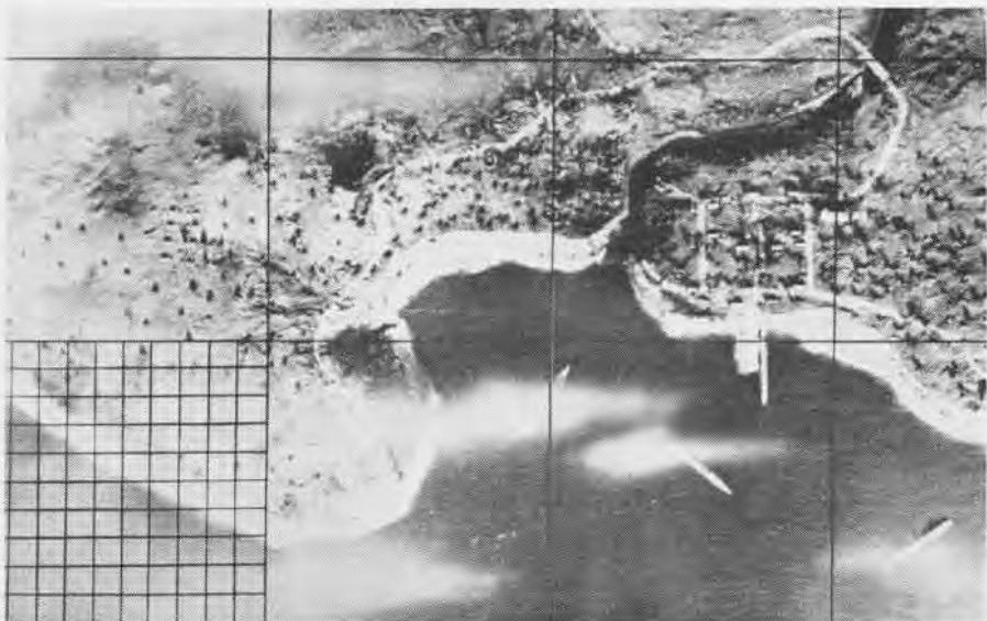
"M" Square grid imposed over photograph helps spotter to orient shell hits and report his corrections in range and deflection back to ship; miniatures help simulate reality of action
