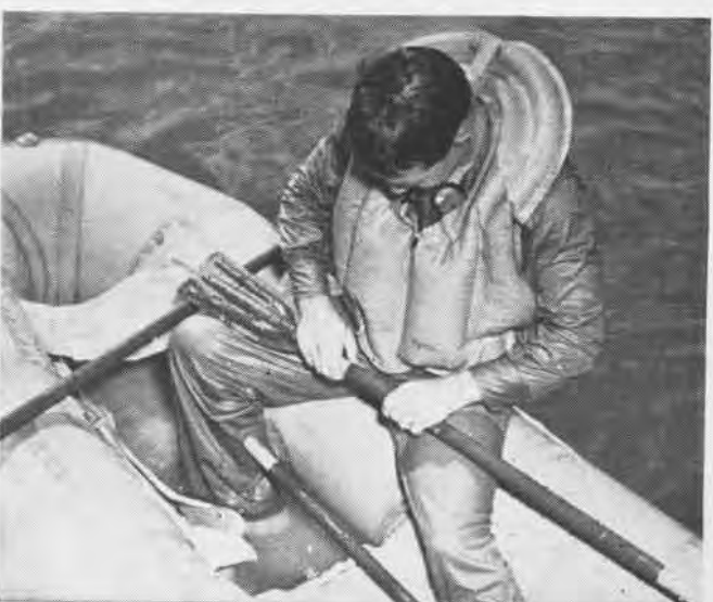
7 To control the raft, assemble the demountable oars which are in the large pocket seen in the left-hand side of the photo
