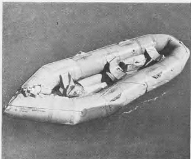
4 Raft is opened after pulling release handle. Important thing to remember is hang on to raft so wind, waves do not drift it
