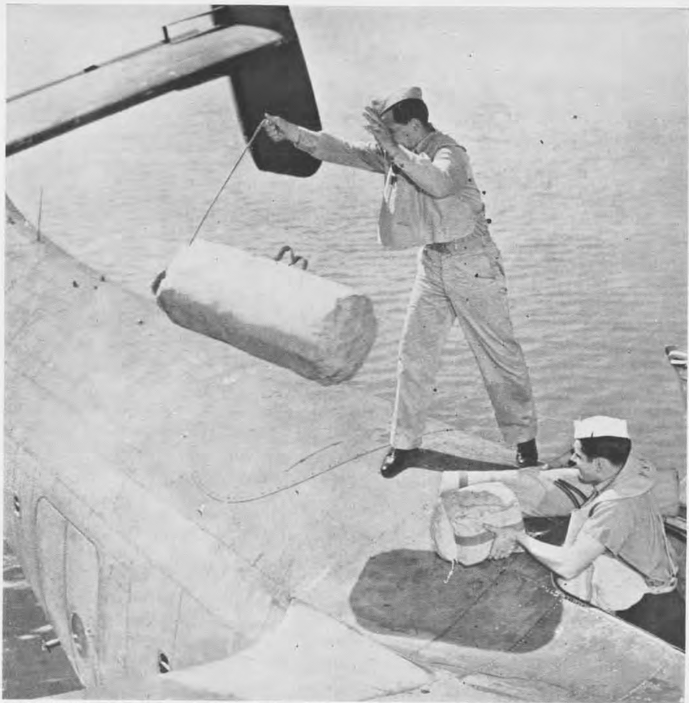
1 Throw the raft overboard from top escape hatch, followed by "Gibson Girl" (emergency radio set). Be sure to hang on to bow line so the raft will not drift away before someone can take to water and control it. Top hatch is usually best for quick exits
