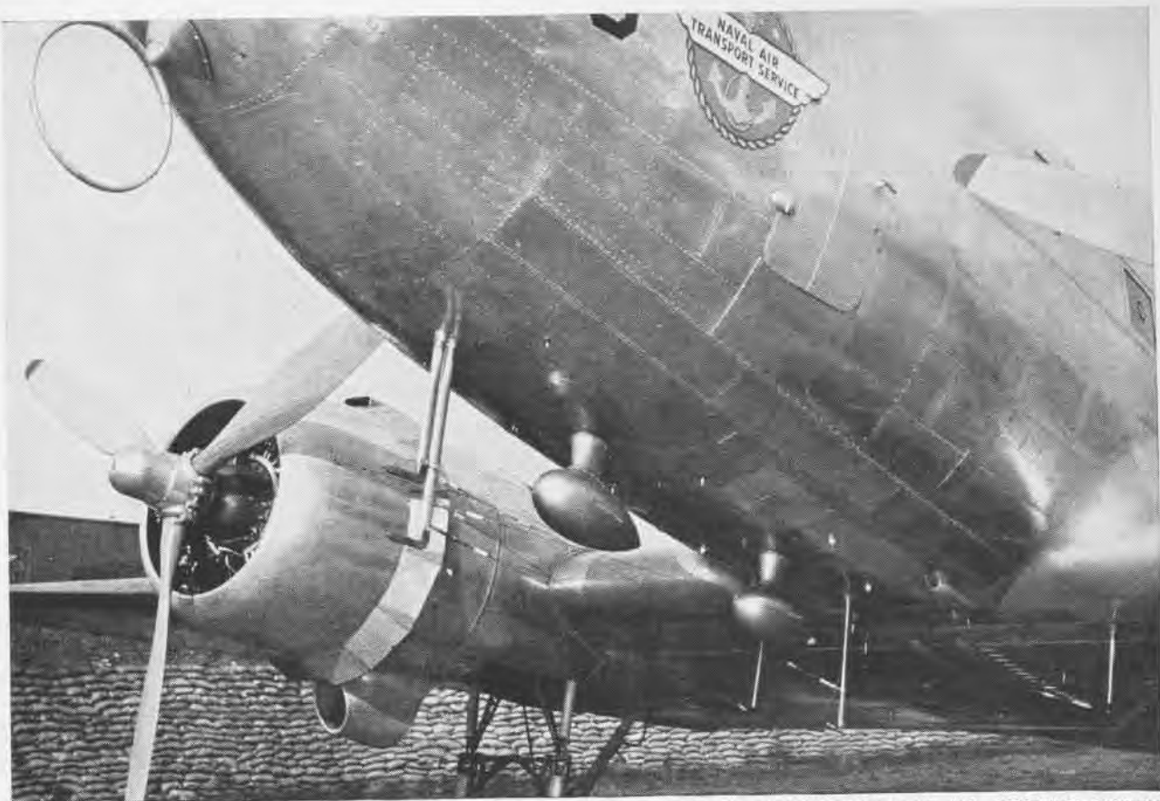
NATS PLANE HAS STREAMLINED ADF LOOPS, FIXED ANTISTATIC LOOP, "T" SENSE AND RANGE ANTENNAS, 75 MC. RECEIVING ANTENNA
