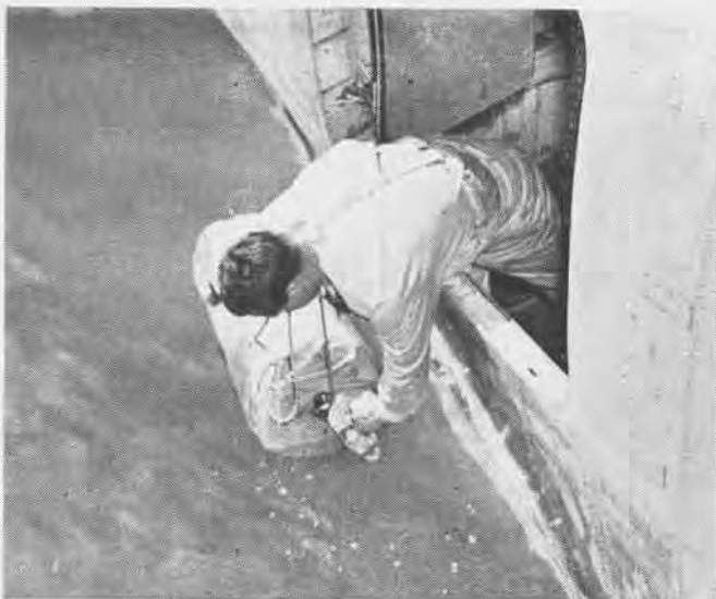
2 If the plane is sinking slowly, the raft can be launched from side emergency hatch. Notice left hand holding release handle
