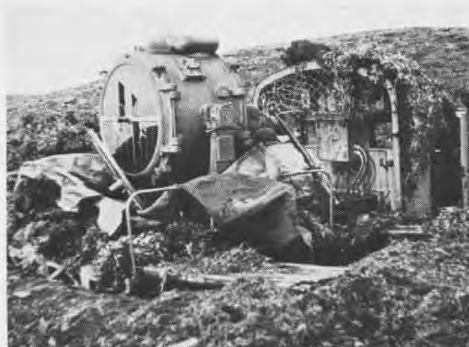
Mounted on a well-revetted camouflaged truck, this 98 cm. searchlight was captured at Little Kiska; truck generator gave power
