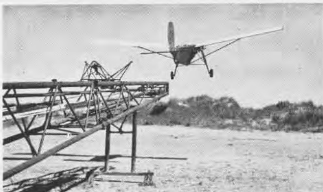
Bungee-powered catapult shoots TDD in air; BuAer furnishes special catapults for ship use; airplane can do many stunts to evade gunners
