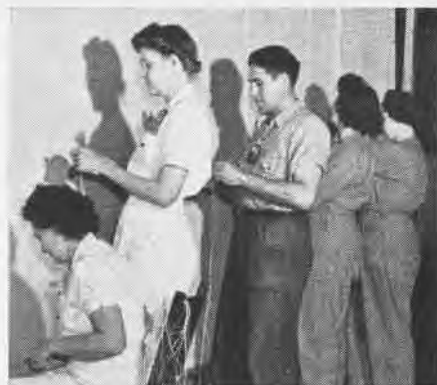
Skilled fingers of naval and civilian personnel work nimbly to rib-stitch a wing
