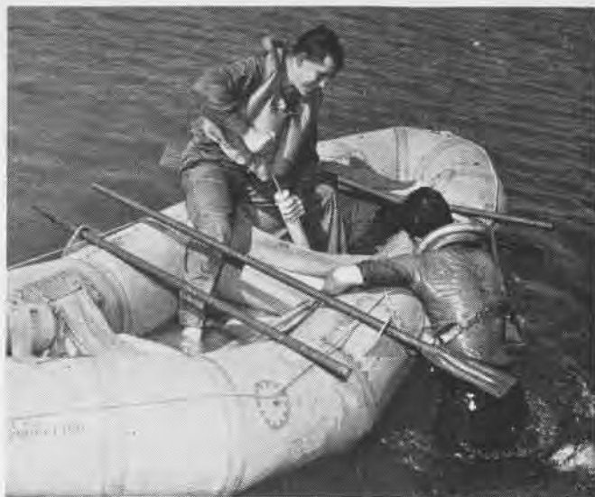
9 Pump up remaining two sections of the life raft with hand-operated pump and balance the raft as others climb aboard
