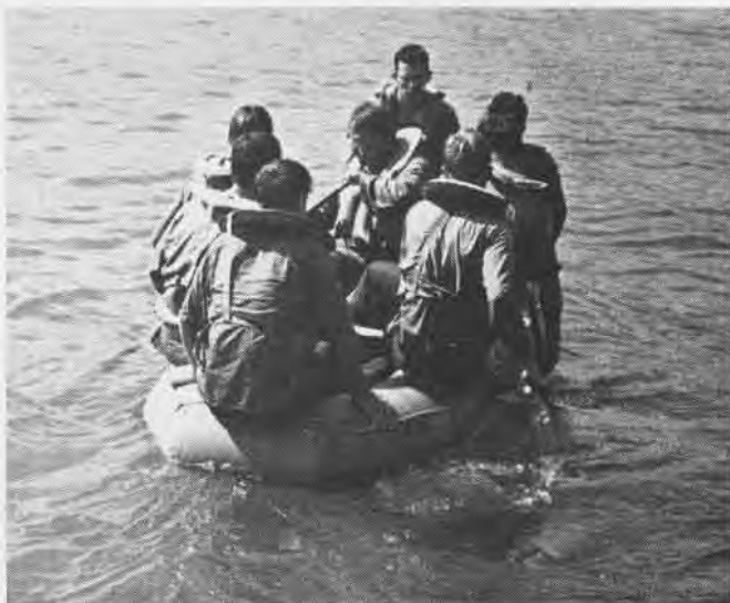
11 MK 7 raft overloaded with eight men, using shortened oars as paddles. Boarders should avoid grabbing lines or seats
