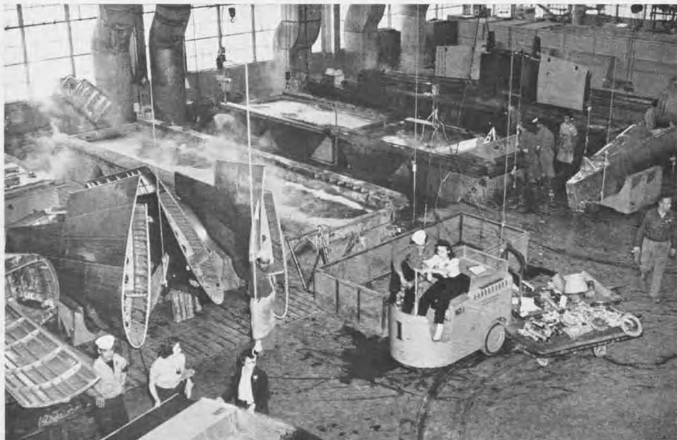
IN THIS BUSY SHOP OF THE A&R DEPARTMENT, PARTS AND SECTIONS OF AIRCRAFT ARE DIPPED INTO GIANT VATS OF BOILING SOLVENT FOR CLEANING
