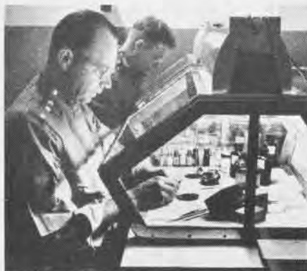
Lettering of instrument dials with radium is one of many intricate jobs A&R performs
