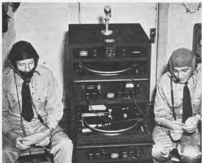
Acoustics room where pilots, wearing lip or nose-shield microphones, test voice intelligibility over engine noises
