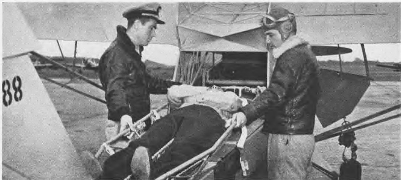
PIPER CUB AMBULANCE PLANE AT PENSACOLA IS EQUIPPED TO CARRY PILOT & SINGLE INJURED MAN; WIRE BASKET IN REAR OF FUSELAGE CARRIES LATTER
