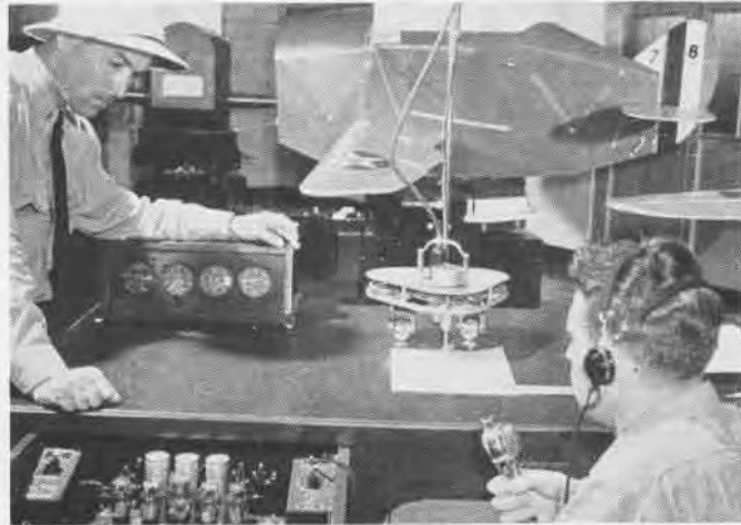
Link trainer gives cadets a chance to test their hands at flying blind, using only plane's instruments for piloting
