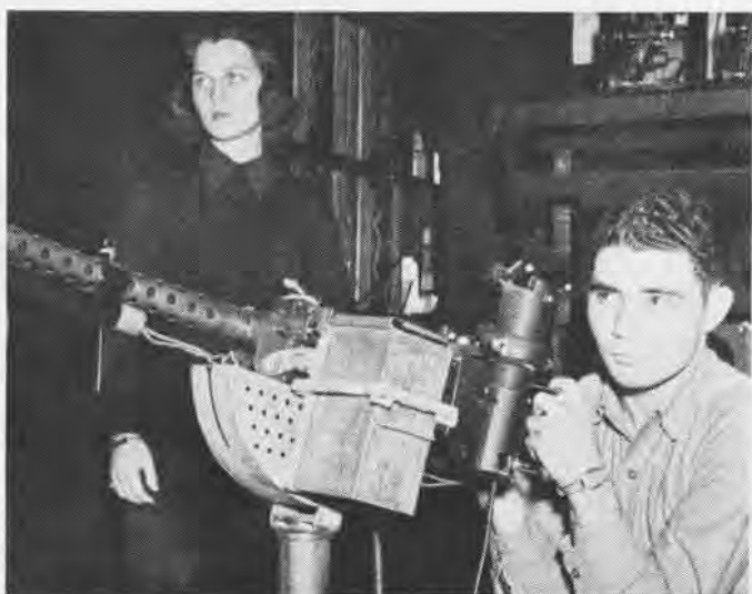
Synthetic training devices are widely used at Pensacola to help gunners; motion picture sighting trainer proves popular
