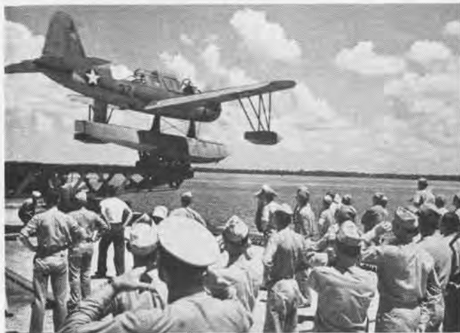
Catapulting of OS2U gives pilots training in type of take-off which they will use if assigned to battleship, cruiser
