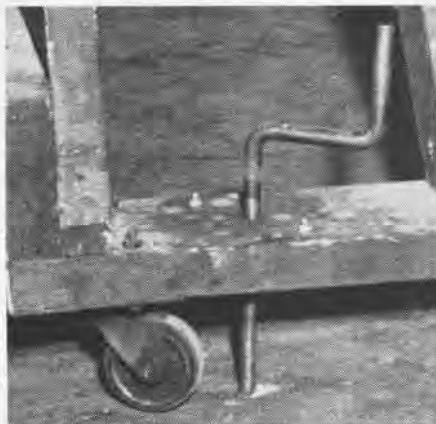
JACKS UP ENGINE STAND TO PREVENT MOVING
