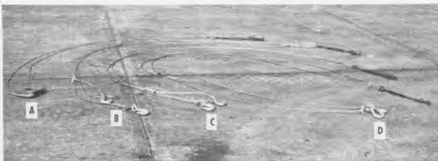
FOUR STEEL CABLES, WITH FITTINGS TO ATTACH TO PADEYE AND PLANE, ARE EASILY ADJUSTED
