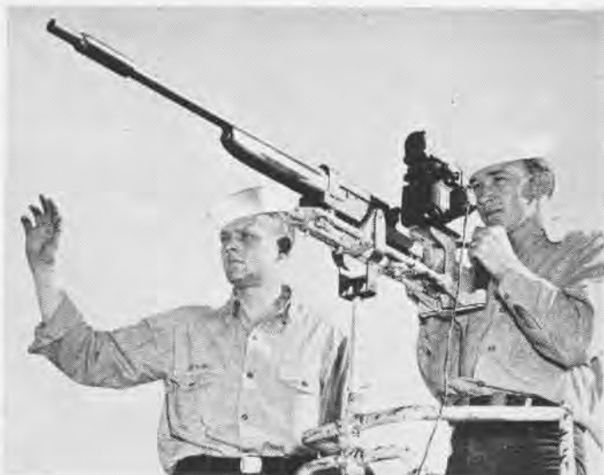
Shotgun mounted on swivel with spade grip is used to fire at incoming target; helps stress correct lead and follow-through
