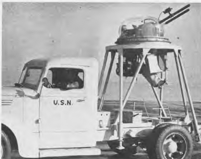
Turret firing is vital to air gunners; here turret mounted on truck aids mobility; gun camera mounted on right barrel
