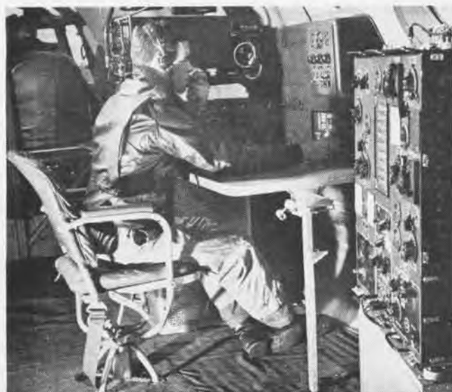
Radio "shack" of the Mars , behind the pilot's cockpit, has ample room; operator has 24 contact points inside the plane
