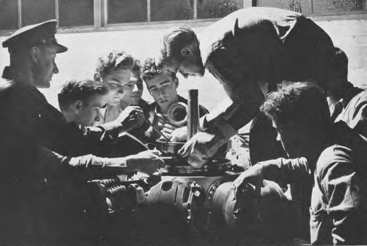
STUDENTS WORKING IN SMALL GROUPS, UNDER CAPABLE INSTRUCTORS, LEARN TO DISASSEMBLE AND ASSEMBLE THE SBD'S POWER PLANT, THE R-1820
