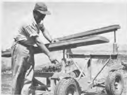
BOMB TRAILER AND JACKS MAKE UP WING DOLLY
