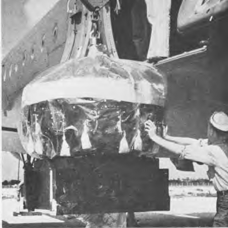
Aircraft engine being hoisted aboard NATS plane is packaged in pliofilm bag, with numerous containers of silica gel dehydrating agent inside to absorb moisture. A rusty engine would be useless
