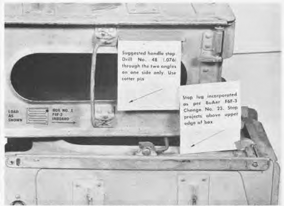
ELIMINATE PROTRUDING STOP LUG WHICH MAKES REMOVAL OF F6F AMMUNITION BOXES DIFFICULT
