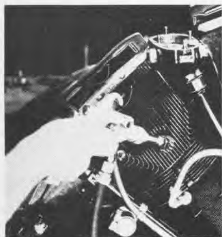
SLUSH CYLINDER THROUGH SPARK PLUG HOLE
