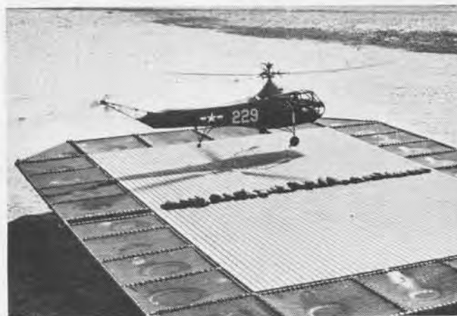
Helicopter can hover a few inches from "practice deck," which can be made to roll, simulating landing conditions on a ship
