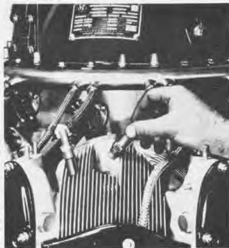
CYLINDER DEHYDRATING PLUG KEEPS INSIDE DRY
