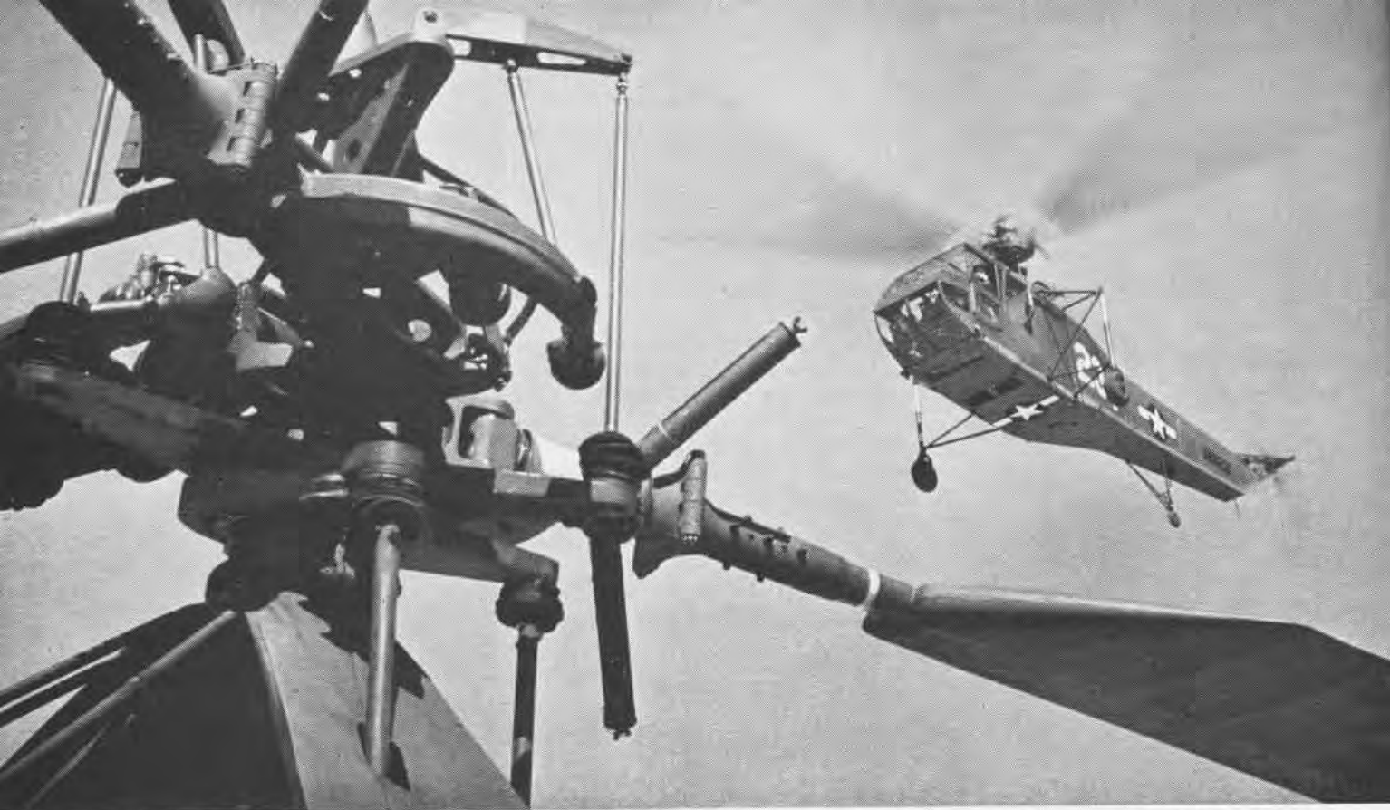
HELICOPTER HOVERS AFTER TAKING OFF FROM SHIP; ROTOR HEAD OF SECOND HNS-1 MODEL IN FOREGROUND SHOWS COMPLEXITY OF MECHANISM
