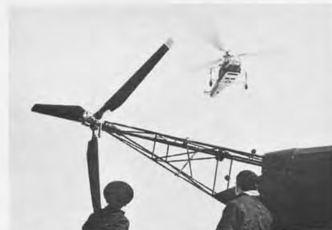
Tail rotor on helicopter compensates principally for engine's torque; gets power from same engine that drives main rotor
