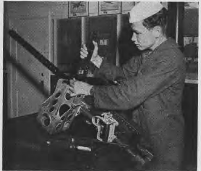
Stripping his gun , this mech learns the names of parts and how they are assembled. Many hours of training are spent on this job
