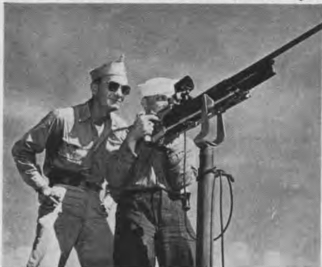
Shotgun with spade grip, mounted on swivel, give gunner practice in firing at clay pigeons tossed into air from varied angles
