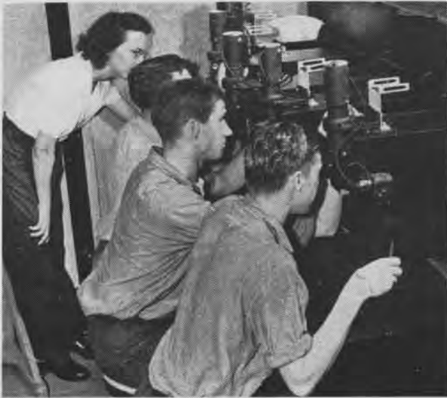
Range estimation device, equipped with movable mirrors, gives student practice in using ringsight to figure attacker's range
