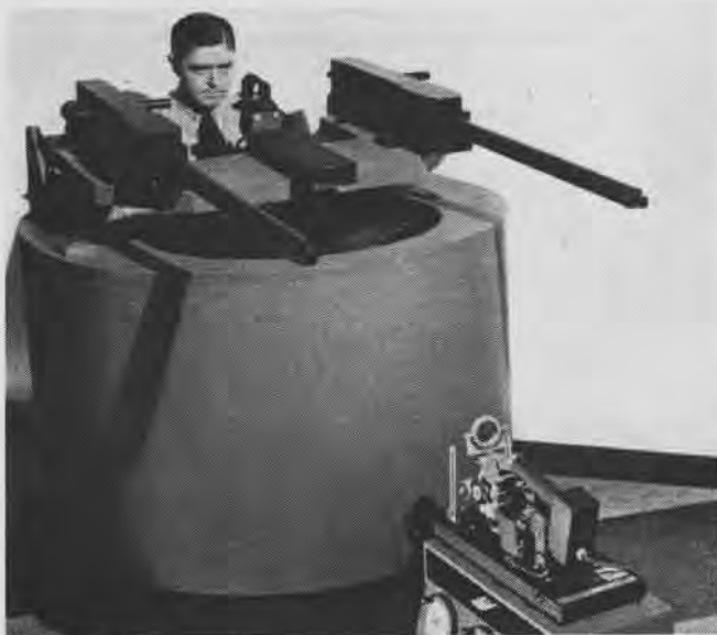
Spotlight animator projects spot of light on wall or screen so that gunner can learn automatic manipulation of turret, sight
