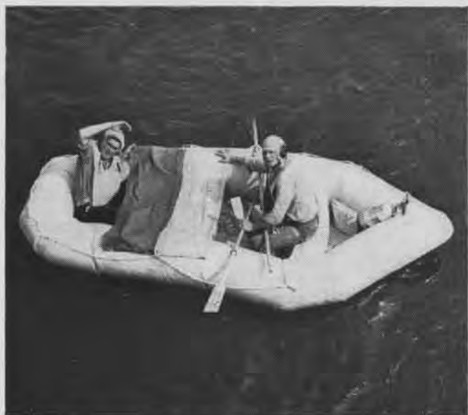
Spread over life raft, the sail signal directs the plane overhead to notify a rescue agency of its position and dispatch aid
