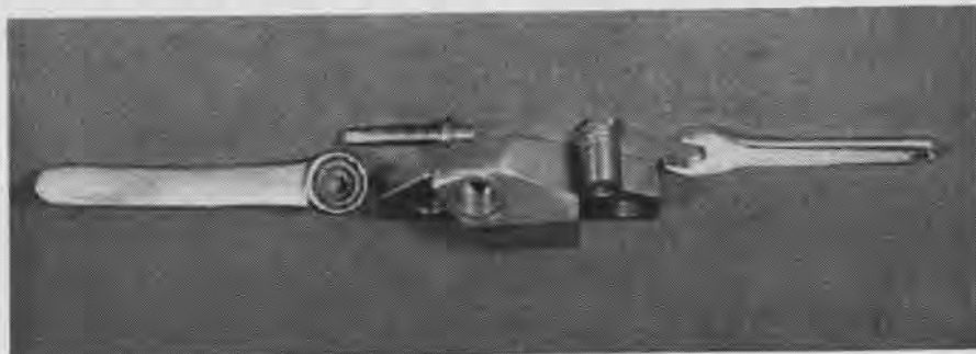
BUSHING AND SCREW DRIVER WORK TOGETHER IN FIXED ALIGNMENT AS OIL JET IS REMOVED
