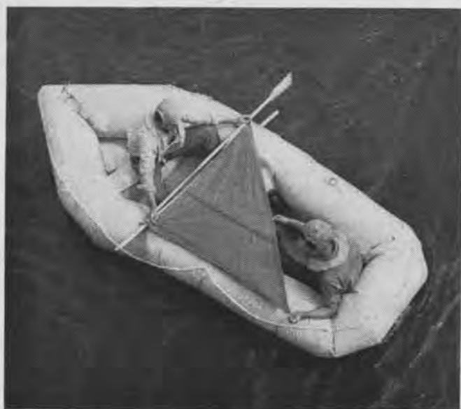
Blue triangle signal notifies the search plane that the men on the raft need equipment which they will indicate by signaling
