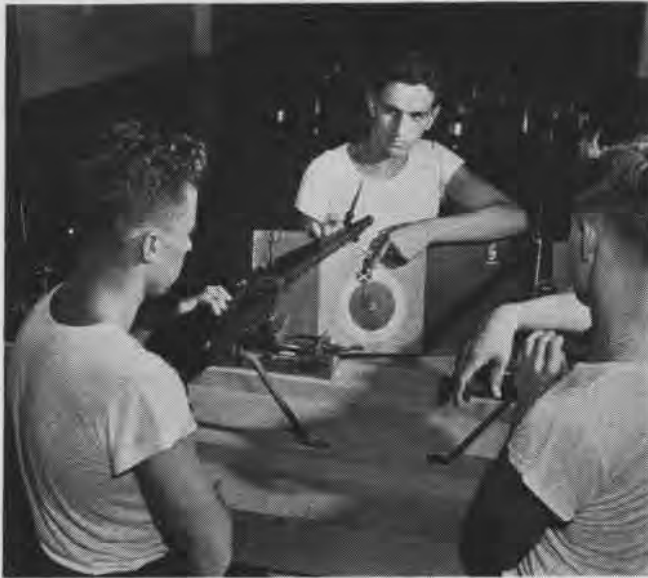
Boresighting of machine guns, to test accuracy of sights, is one of first things taught embryo marksmen at all gunnery schools
