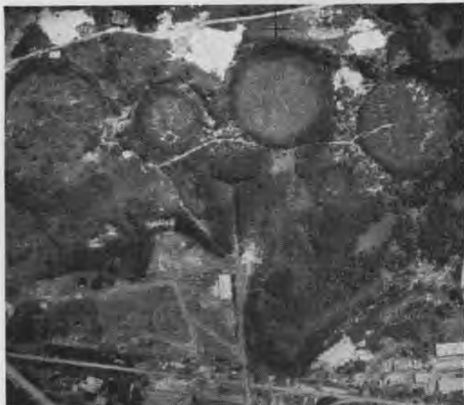
Huge oil tanks buried in hillside at Saipan easily recognized in photographs despite attempt to make them blend in landscape
