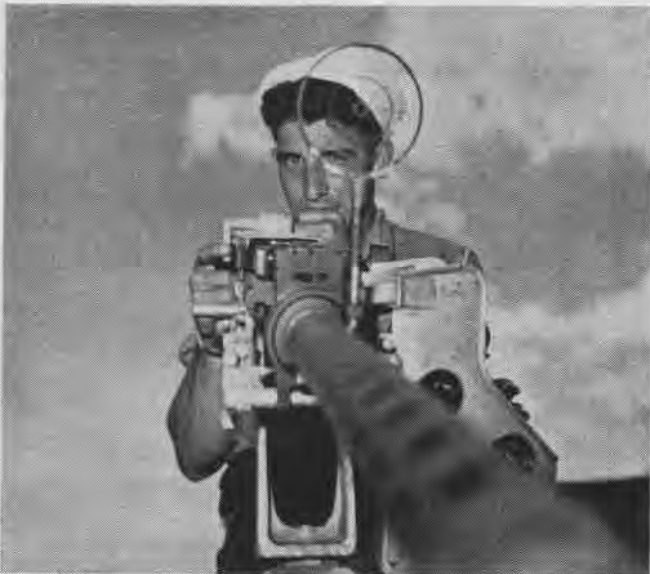
Ringsight helps gunner estimate range, deflection to use when firing at attackers. This operation must be automatic in action
