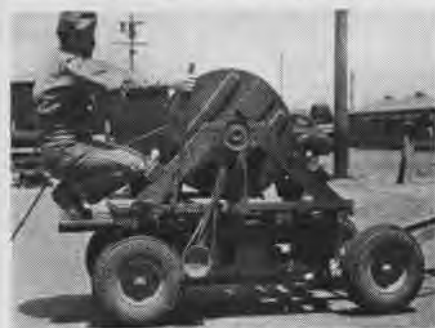
BELT-PULLEY SYSTEM ROLLS UP TARGET LINE
