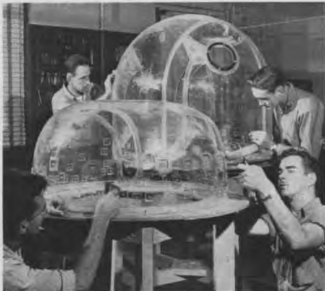
Aviation metalsmith trainees learn proper technique as they polish and repair plastic turrets in the shops at NATTC Norman.
