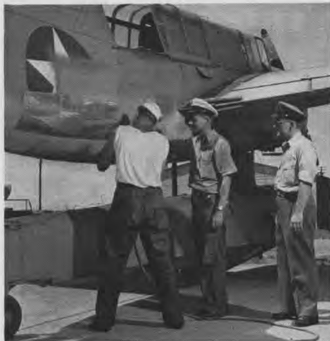
Under watchful eye of instructor, this future AM makes a section skin replacement during on-the-job NATTC training course.
