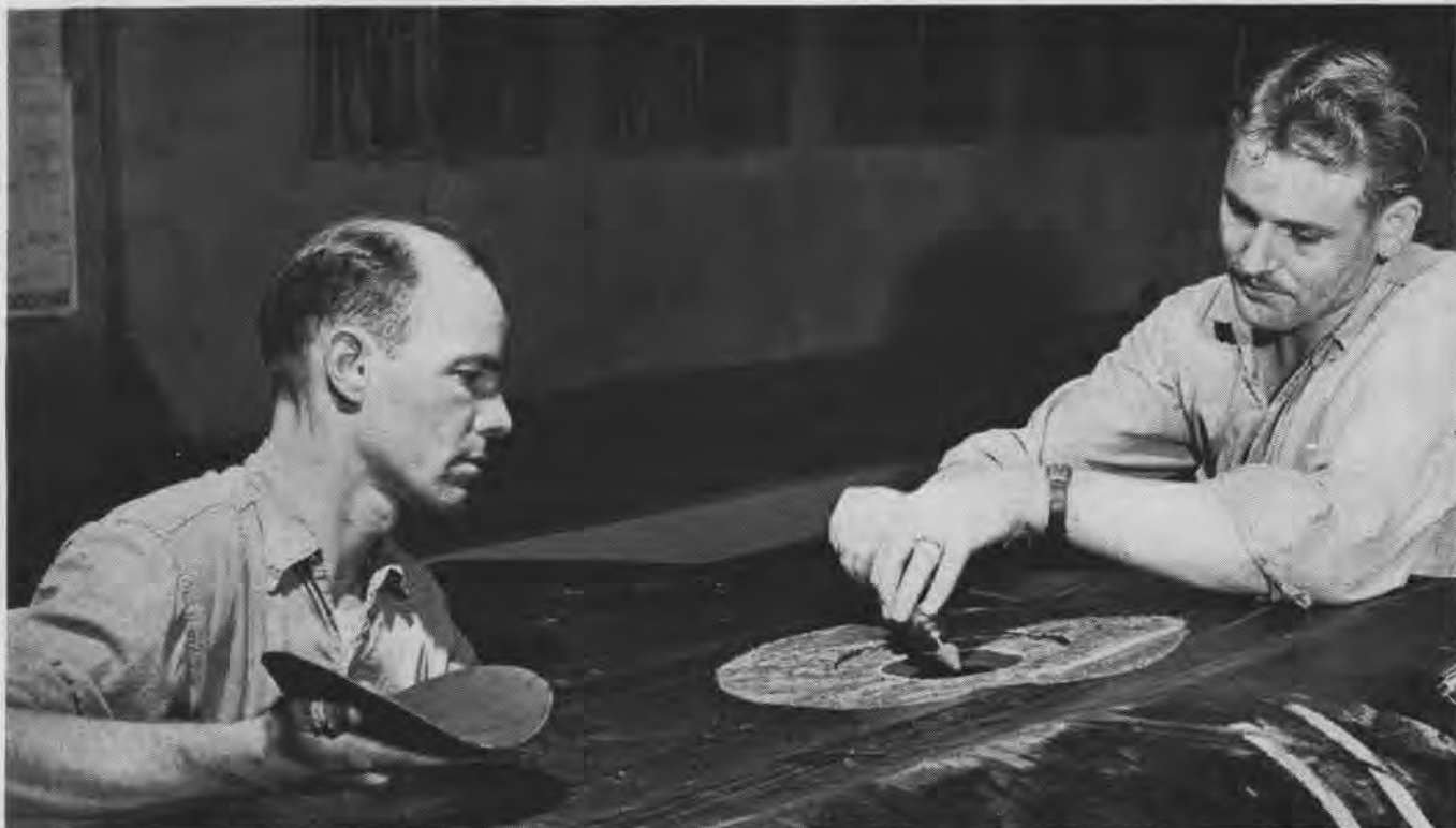
REPAIR OF BULLET-PROOF TANKS, SELF-SEALING CELLS, PART OF TRAINING PROGRAM AT NAVY'S RUBBERIZED EQUIPMENT REPAIR SCHOOL
