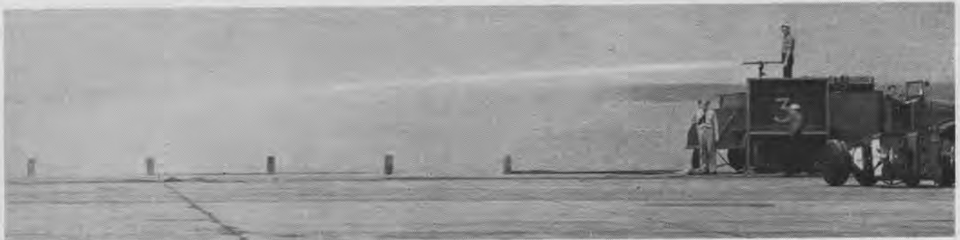
STREAM: Water under 750 lbs. per sq. in. pressure is projected from turret nozzle on a John Bean truck, similar to units now in field. A solid stream under pressure is used to sweep flames away and to cool cabin area. Stream is projected approximately 60 ft.
