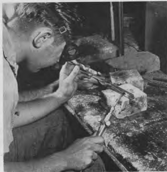
AM's master "know-how" of all aviation welds by actual job training. Aluminum welding is most difficult type to learn.
