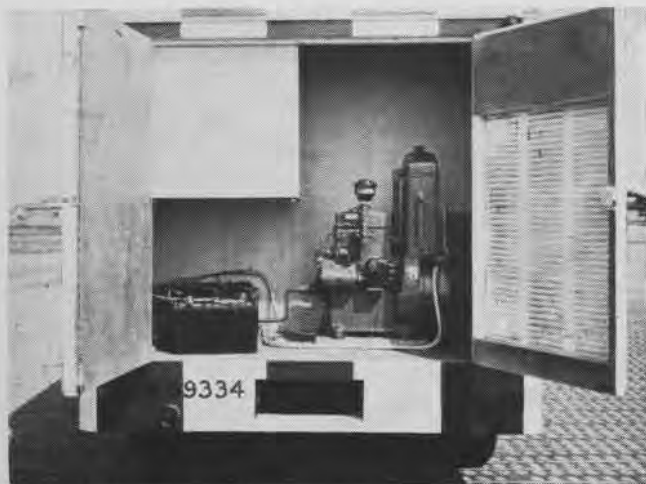
Asbestos-lined walls provide insulation to protect compartment in which is housed 32-volt Kohler motor with batteries to give power
