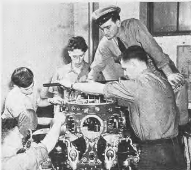
Fresh out of boot camp, AMM strikers tear down a twin-row radial engine under chief's watchful eye as part of training at NATTC
