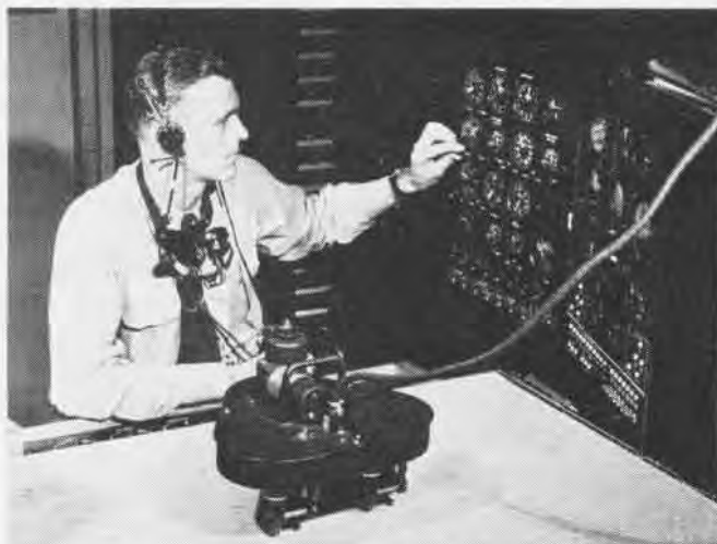
Instructor at control panels watches how pilots in trainer fly the plane. "Crab" in foreground operates same as in regular Link trainer, following the flight problem being flown. Experienced men act as instructors. Device saves tying up planes on the line
