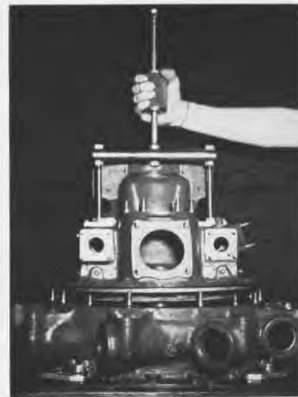
BLOWER PULLER SAVES TIME, REDUCES DAMAGE
