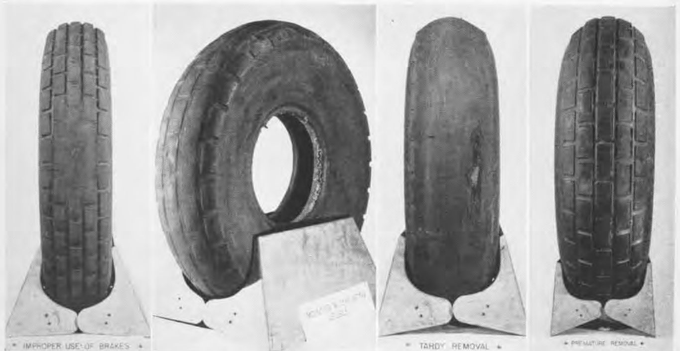
EACH OF THESE TIRES SHOWS A BREAKDOWN IN TIRE CONSERVATION. PROPER INSPECTION AND MAINTENANCE OF TIRES PREVENTS SUCH ABUSES
