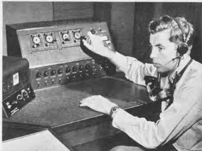
Radio communication between pilot, navigator, radioman and flight engineer is maintained at all times while operational trainer is in use. Instructor at control panel checks on proper procedure and advises students when they are making any bad errors
