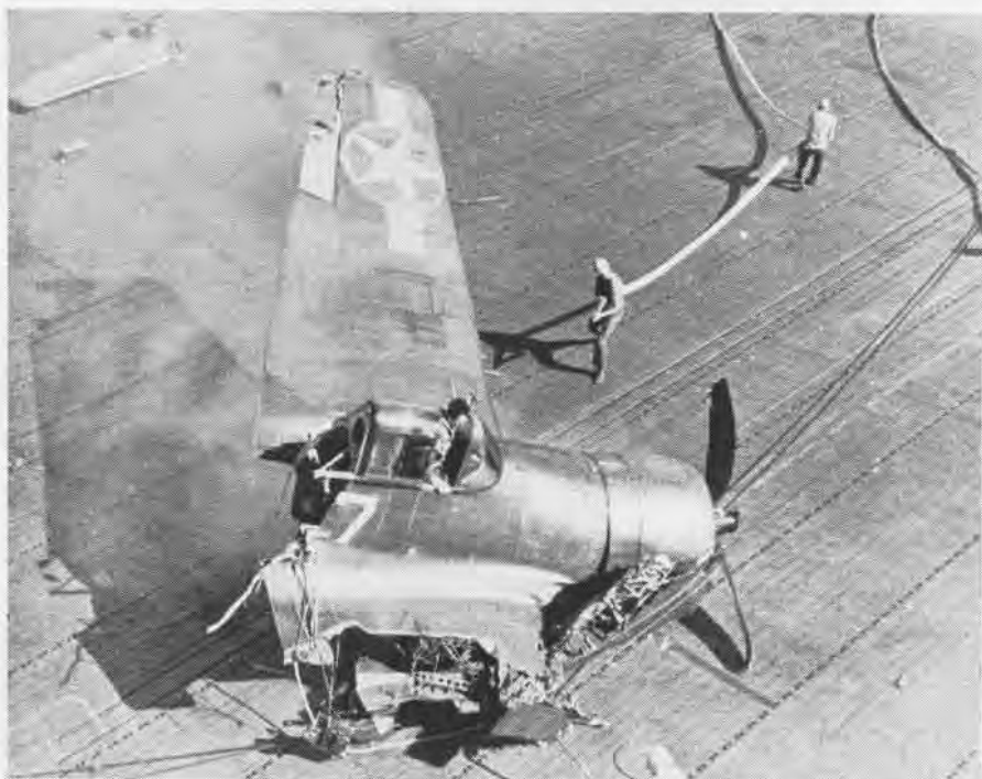
ONE OF THE most remarkable crashes in naval aviation history in which the pilot walked away from what was left of his plane is illustrated above. Shot up over Palau, the ensign started back with his hydraulic system gone, his flaps useless, a large hole in his right wing and his ailerons smashed. Coming in on his carrier he sheared off a wing and the tail on a gun turret, but emerged from his wrecked Hellcat with only a few scratches.
