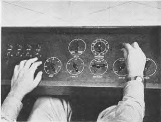
Special instrument panel in control room permits instructor to introduce "trouble" for flight engineer, navigator or pilot by flip of dial. He may increase weight, change wind direction or velocity, or produce rough air or wing ice for them to remedy
