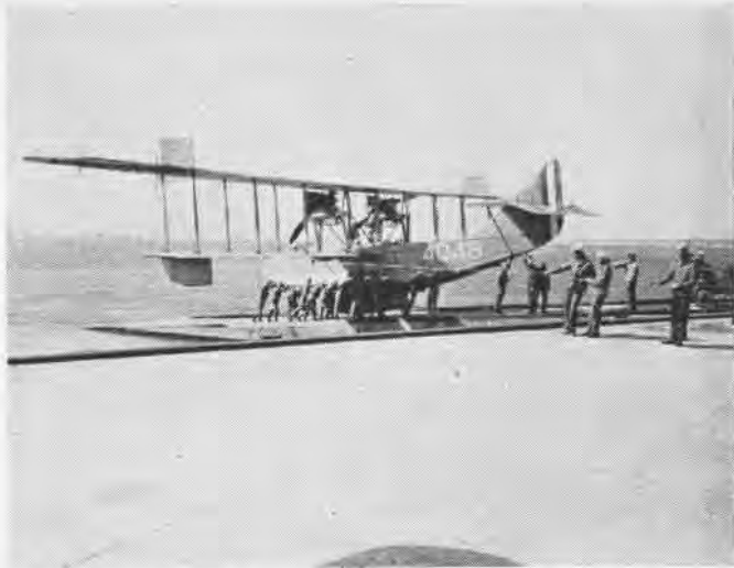
Members of the crew beach one of the H-16 seaplanes by hand on concrete ramps, comparable to World War I seaplane barges
