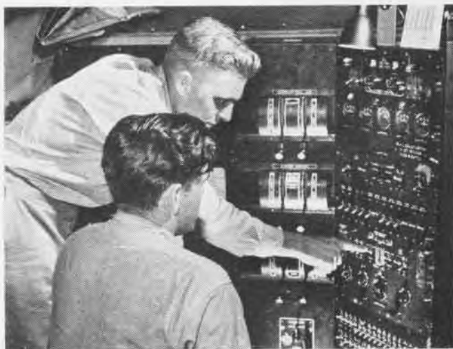
Flight engineer gets the word on PBM engine panel from instructor. Instruments react exactly as though plane was in flight so men get realistic though synthetic training. Crew coordination is an important value gained through use of this special device
