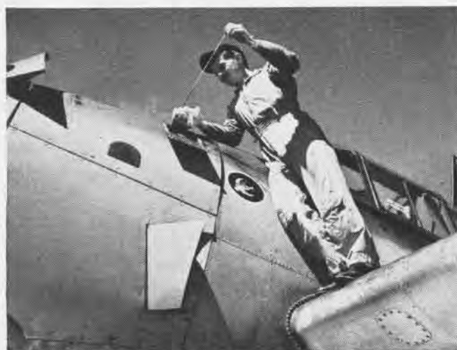
Checking the oil in the engine of TBM Avenger torpedo bomber. Farrell, an experienced mechanic before entering the Navy, has had thorough Navy training as a machinist's mate. With plane captain and deck crew he keeps his plane in tiptop shape
