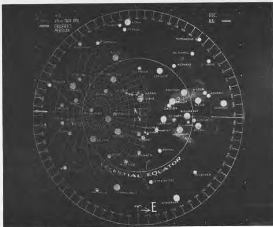
DEMONSTRATION MODEL OF RUDE STAR FINDER IS MADE OF PAINTED PLYWOOD, PLEXIGLAS
