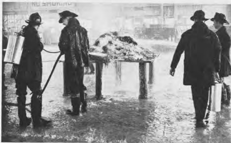
FIRE DRILLS and tests of equipment help to emphasize the importance of fire protection in naval aviation operations. Firemen at NATC Corpus Christi are shown here combining a practice workout with a test of an overhead sprinkling system. They are putting the final touches on a bonfire ignited in one section of a hangar on the enormous base.
