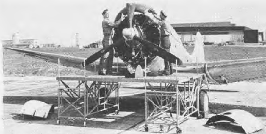
WITH THE CATWALK BETWEEN, STANDS MAKE A WORKING PLATFORM AROUND NOSE OF SBD PLANE
