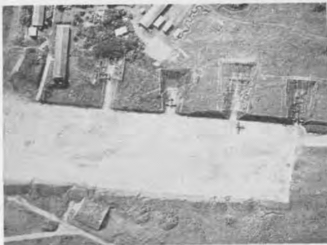
Japs hide their planes in large excavated revetments covered with light framework for camouflage. Each "hide" houses several planes
