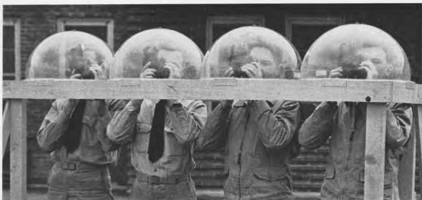
STUDENTS USE ASTRODOME DEVELOPED AT PENSACOLA TO TAKE SIGHTS IN CELESTIAL NAVIGATION WITH THE AIRCRAFT SEXTANT, MARK FIVE
