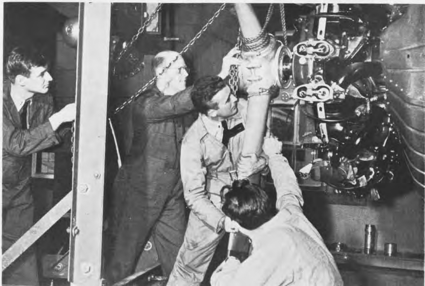
HYDROMATIC PROPELLER IS MOUNTED ON ENGINE BY STUDENTS AT GROUND SCHOOL LAB, QUONSET. ONE-MONTH COURSE TRAINS FOR ACTIVE DUTY
