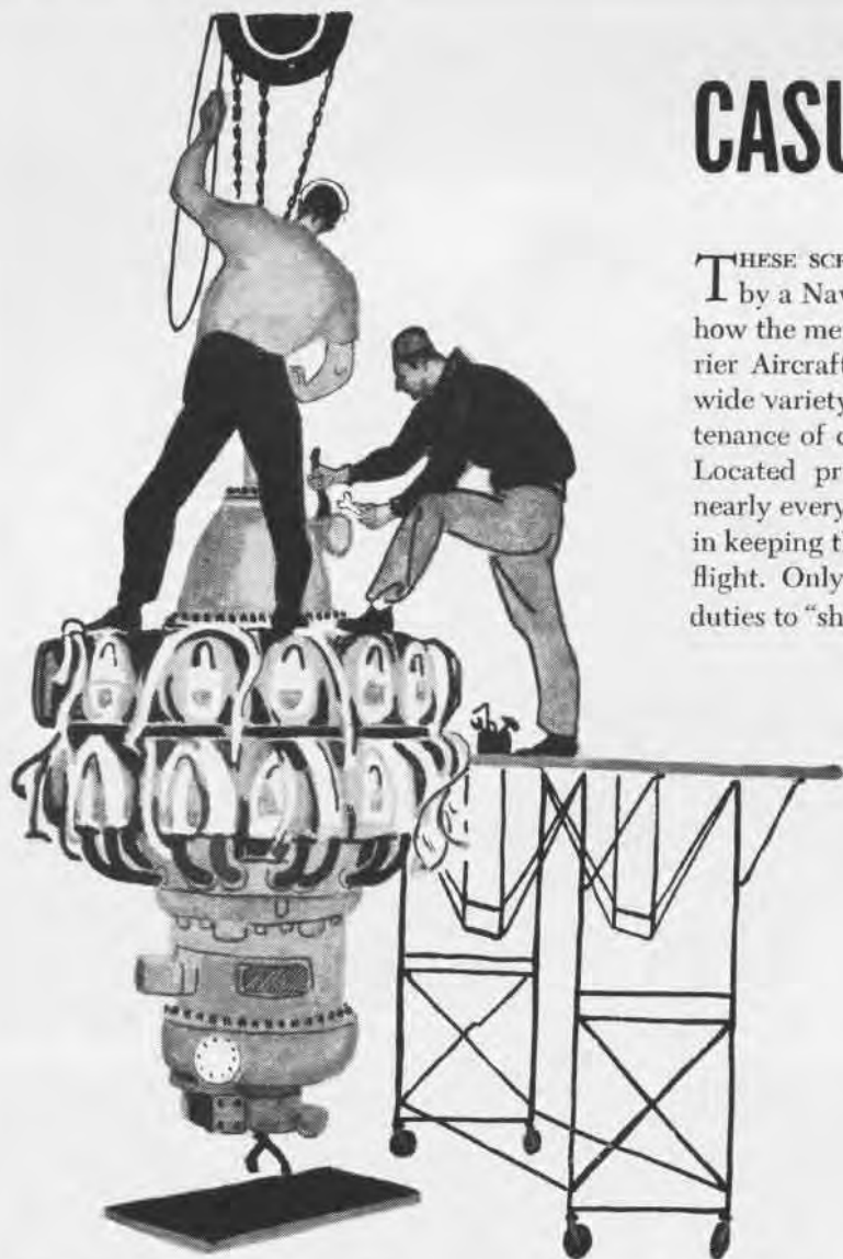
SKILLED MECHS, WORKING AGAINST TIME, REPLACE THE ENGINE IN A FIGHTER PLANE
