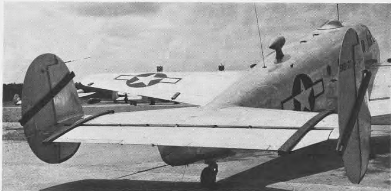
WHITING FIELD'S USE OF BATTENS ON SURFACES PROVIDES DEPENDABLE PROTECTION AGAINST HIGH WINDS OF TYPE THAT PREVIOUSLY DAMAGED 40 SNB
