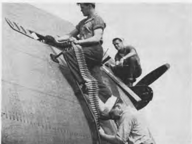
Rearming a TBF's wing guns is done by a CASU ordnance crew when the plane finishes a mission or returns to its station after a gunnery run. Some service units operate their own training schools to keep men up on newest developments in engines or ordnance
