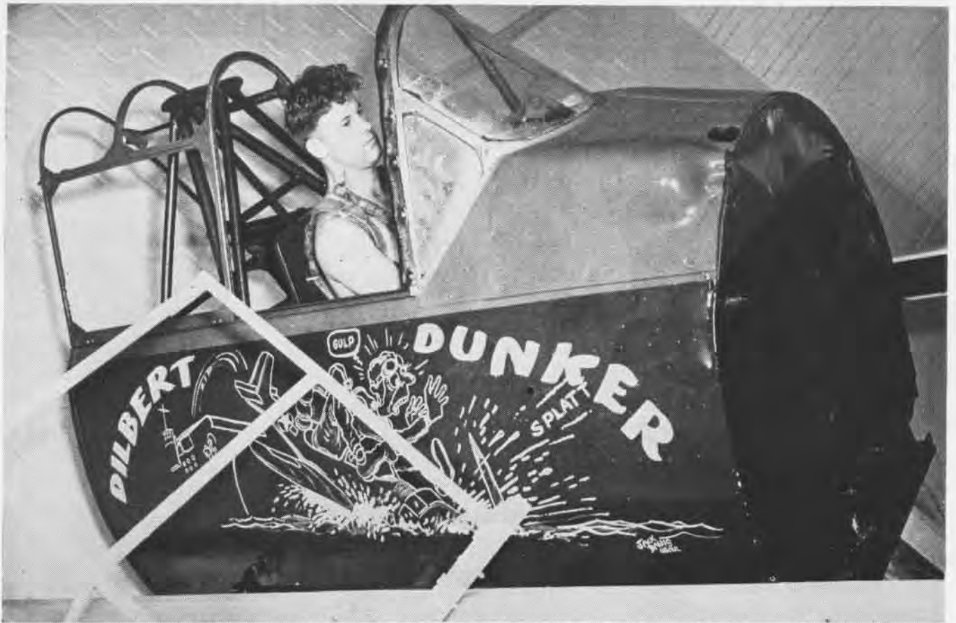
DILBERT DUNKER AT TOP OF 39-FT. SLIDE, READY TO GIVE CADET PRACTICE IN GETTING OUT OF COCKPIT UNDER WATER DEVICE BUILDS CONFIDENCE
