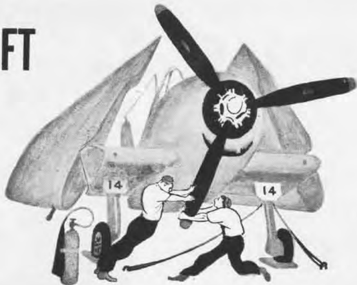
MEN PULL PROP THROUGH BEFORE STARTING ENGINE OF ONE OF THE POWERFUL FIGHTER PLANES PARKED ON THE LINE
