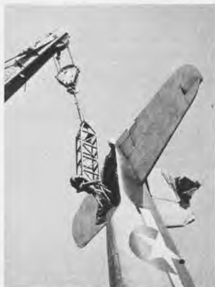
RIGGING PREVENTS DAMAGE TO TAIL SURFACES
