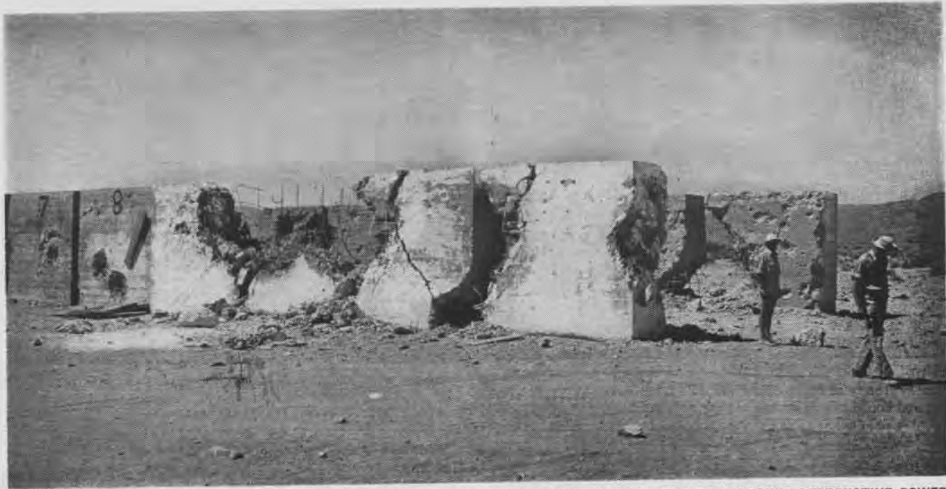
THICK REINFORCED-CONCRETE WALLS AT INYOKERN RANGE GIVE PILOTS A GOOD CHANCE TO STUDY ROCKET DESTRUCTIVE POWER
