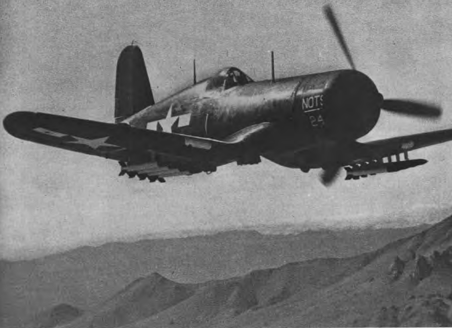
CARRYING EIGHT 5" HVAR ROCKETS IN ITS LAUNCHERS, F4U HAS FIREPOWER OF A DESTROYER AS IT FLIES OVER INYOKERN RANGE
