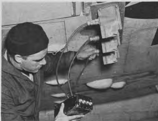
Before rockets are installed on the aircraft, ordnanceman checks the circuits to see that each launcher will be energized on firing. BUAEr has newer style test kit to supplant this model. A stray spark would cause rocket to fire
