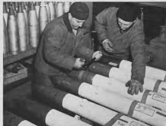
Explosive head with its eight-pound charge of powder is put on tightly. Ordnanceman uses strap and wrench to secure it without damage. Rows of different types of heads are on the bench behind, some explosive, some inert for scientific study
