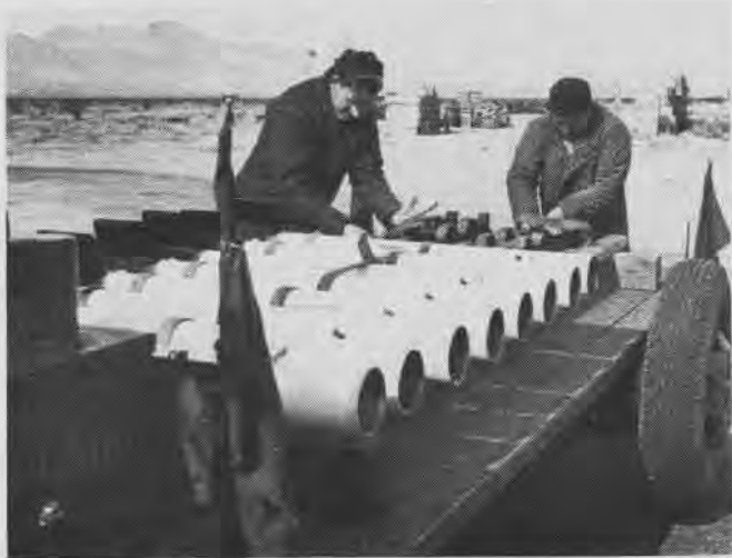
Assembled motors and fins are loaded carefully on truck to avoid breaking powder grain, which would cause rockets to blow up in midair. Smoking always is barred in assembling areas. Fire extinguishers always must be kept close at hand
