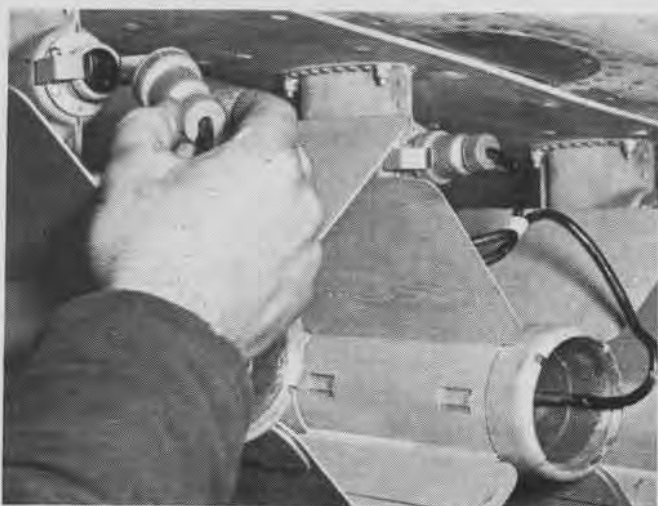
Close-up of rear zero length launcher shows male plug attached to pig tail of a 3.25" motor. HVAR has similar pigtail, which is blown out upon firing. Nose fuze is installed on rocket after it is put on plane, the base fuze only at the assembly shed
