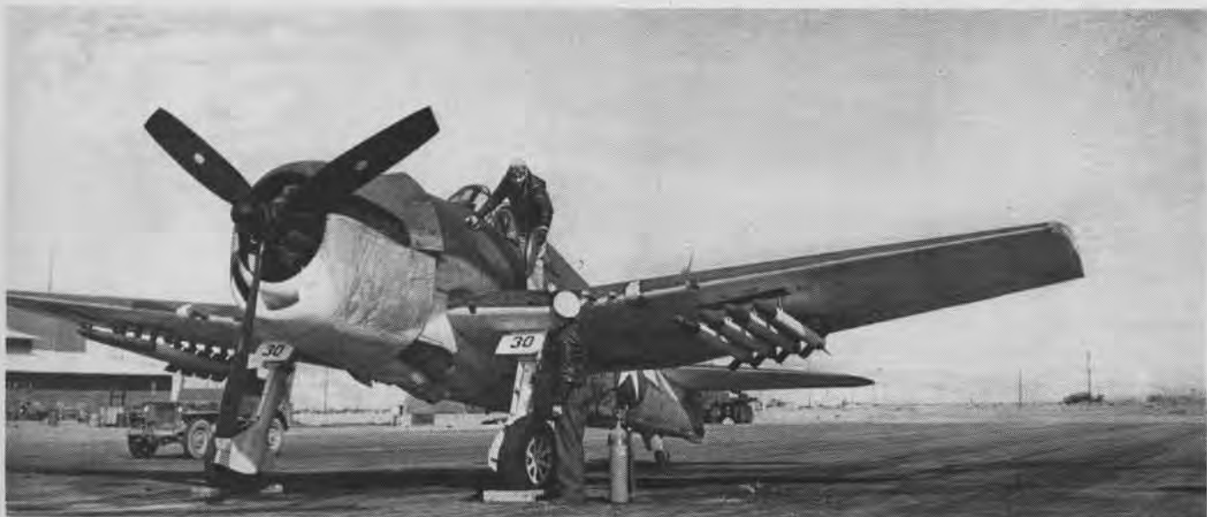
WITH EIGHT HVAR ROCKETS INSTALLED, SAFETY OFFICER HANDS SAFETY PLUG TO PILOT, WHO INSERTS IT IN INSTRUMENT PANEL
