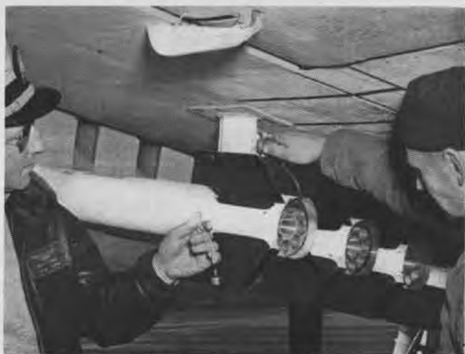
All switches off, safety plug in the hands of safety officer, the ordnanceman makes test with no-voltage light to be sure of energy in circuits, then plugs in rocket pig tail. Workers must stand clear of fore and aft ends of rocket during this operation
