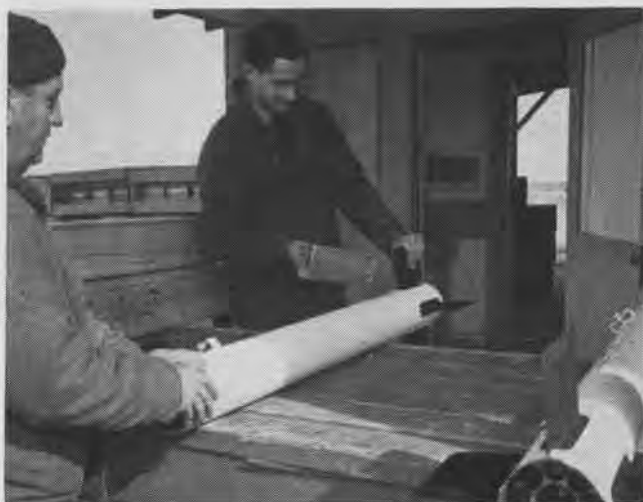
Ordnanceman at Harvey Field uses wooden mallet to hammer fin on early CRT production model rocket. BUORD service production models are fitted with moveable lug bands and one-piece fin assembly. Latest model of HVAR is illustrated on page 25
