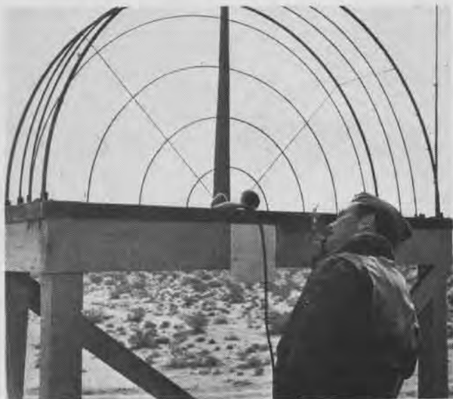
Range officer uses harp to tell the pilot what his dive angle is and when he is in correct range to fire rockets at target
