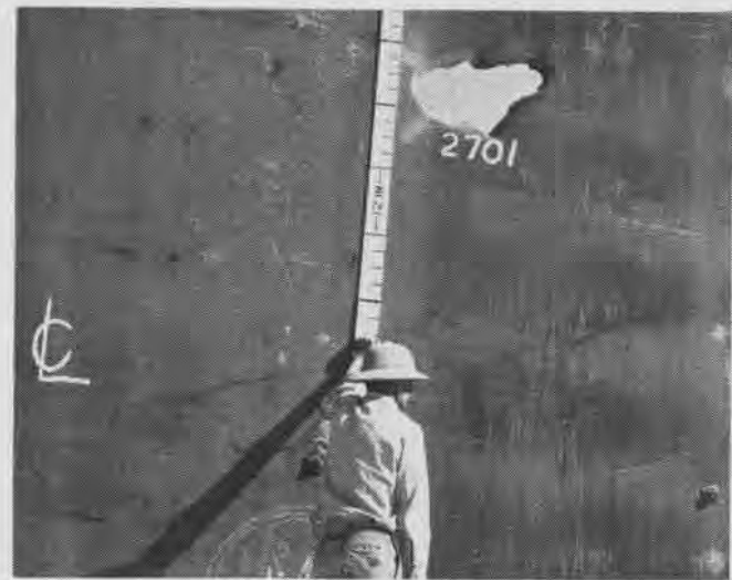
Rockets will pierce armor plate of 1 1/2" or more with ease, as this photo at Inyokern range indicates. Fuzes control firing
