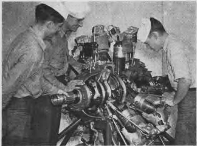
Sectionalized engines are among shop's cutaways. Engines are disassembled, parts are cleaned, sectionalized, then reassembled
