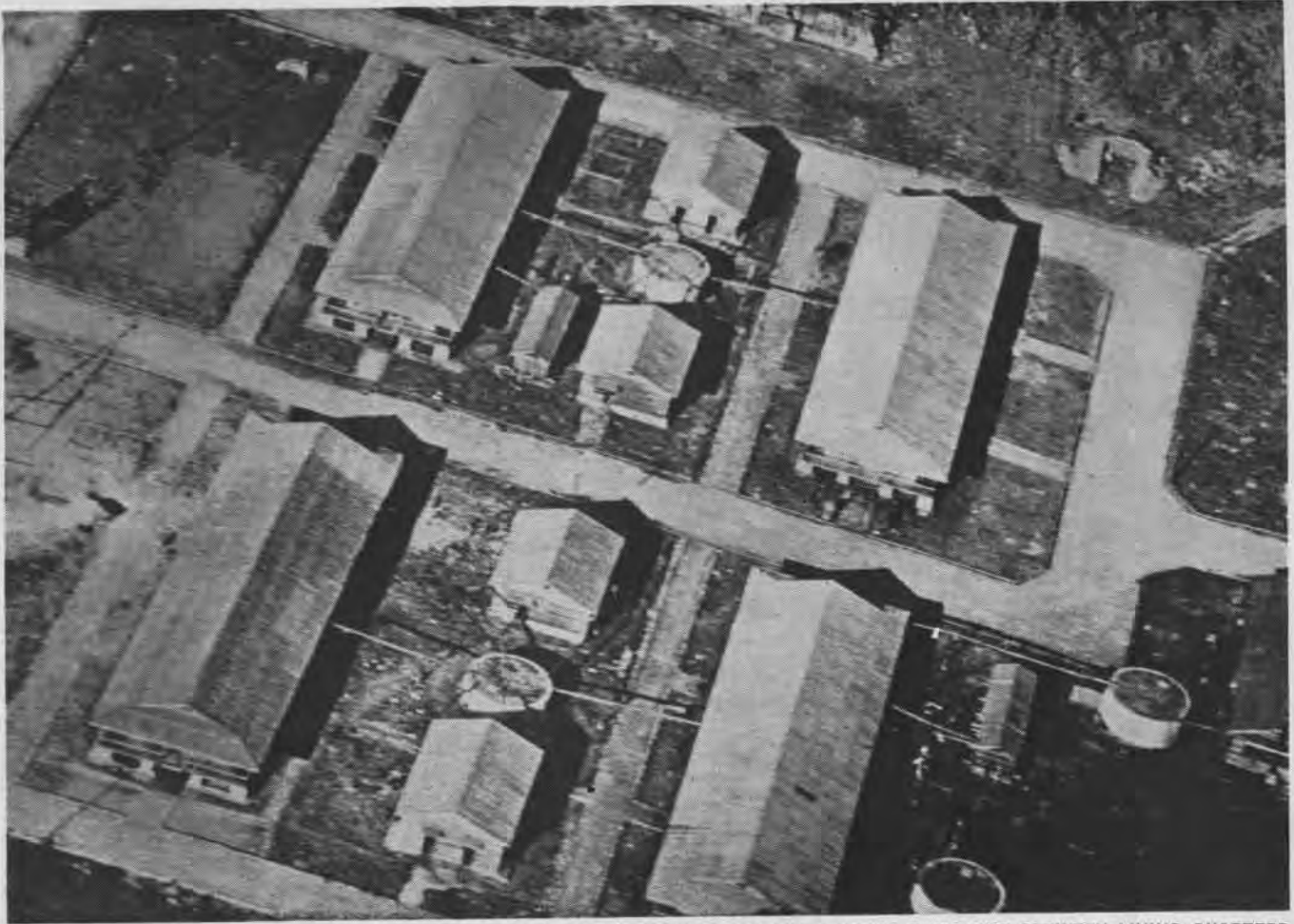
JAPANESE BARRACKS GROUP ON SAIPAN HAD CISTERN AND SMALL LATRINE AND WASH HOUSE BUILDINGS BETWEEN LIVING QUARTERS
