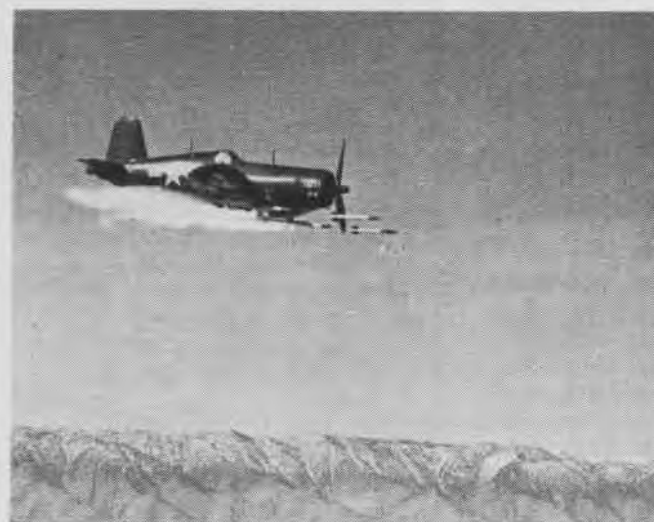
Second pair of HVAR's clear the launchers, close on heels of first two. Firing could be done either in salvo or ripple
