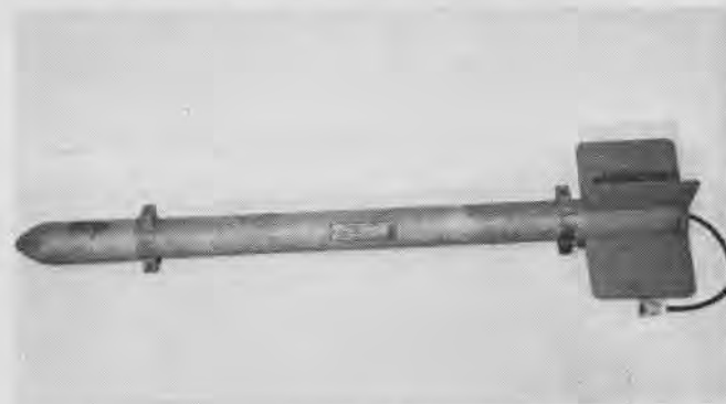
3.5" ROCKET , powered by 3.25" motor, not now in operational use was an early rocket developed. Single ballistite grain in motor provides the rocket with propellant
