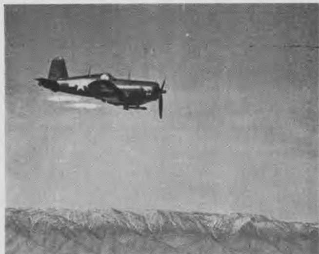
Corsair test plane winging over Inyokern rocket range opens fire with its eight HVAR rockets, arranged to fire in ripple
