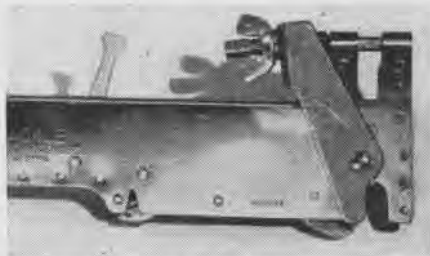
MK3 TYPE SHACKLE BRACKET FITS AN-B10
