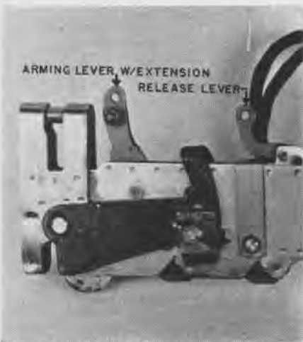
MAG DEVISED ARMING LEVER EXTENSION
