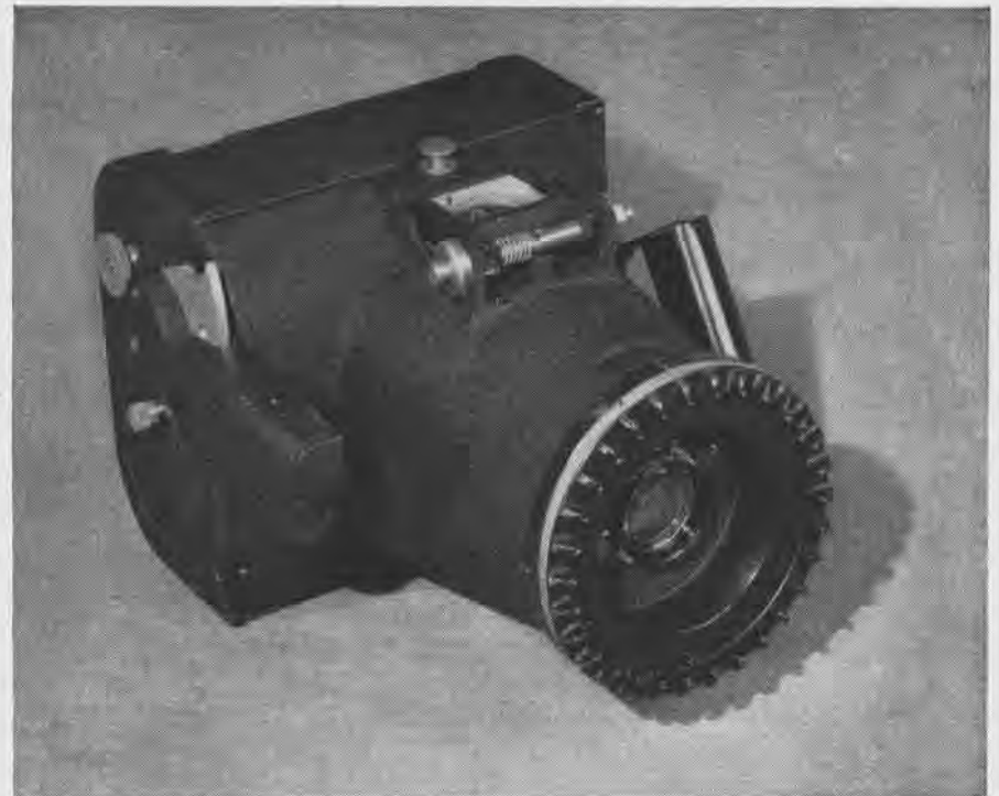
NEW FOCUSING ATTACHMENT CONVERTS THE STURDY K-20 FOR CLOSEUP WORK ON GROUND
