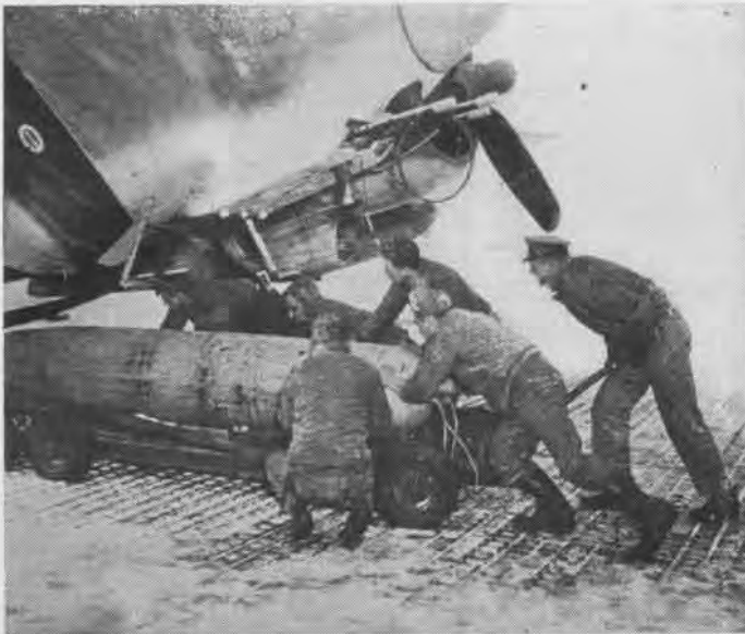
Fleet Air Wing 4 ordnancemen load a torpedo in bomb bay of a Harpoon preparatory to aerial strikes against Japanese shipping
