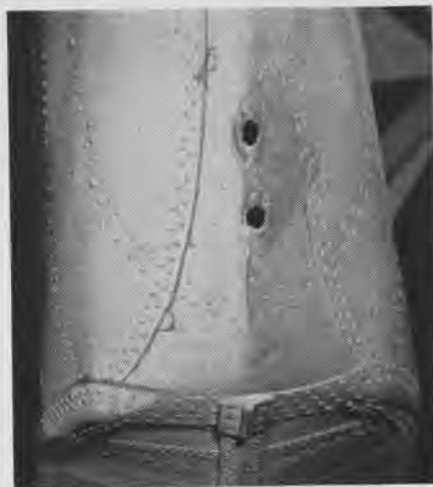
DAMAGE TO FLOAT CAUSED BY LIGHTNING
