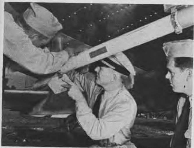
Aviation ordnance officers arm a fighter with rockets. Officers practice with operational type equipment to augment the lessons learned in classrooms. Mk 5 launcher is pictured
