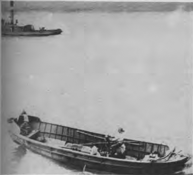
Type B, or "Shohatsu," is used by the initial covering party in landing operations or in barge traffic to transport supplies
