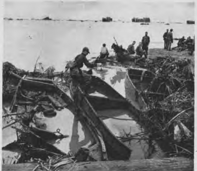
Wooden, collapsible boat has two sections joined by plywood partition. Japs use it crossing rivers and debarking troops and supplies
