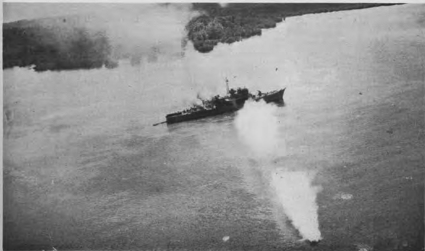
THIS JAP SUBMARINE CHASER PC-13 CARRIES TWO DEPTH CHARGE PROJECTORS AND TWO RACKS AFT. ITS FULL SPEED IS 20 KNOTS
