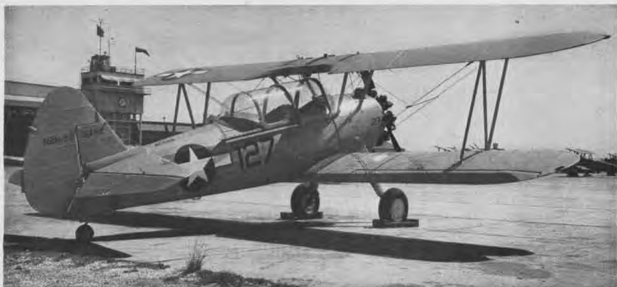
WINTER HOOD ON PRIMARY TRAINER ELIMINATES NOISE ENABLING BETTER INTER-COMMUNICATION BETWEEN INSTRUCTOR AND TRAINEE
