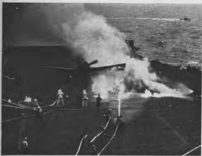
Seconds after tank ignited, carrier fire fighters have blaze under control. Eight lines are readied for use. On right side of deck crewmen battle blaze with high-velocity fog. In center, foam is used. Men on left play low-velocity fog stream
