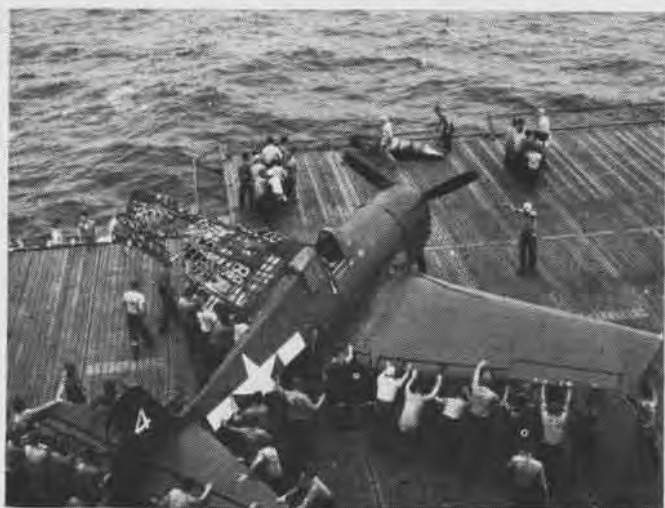
The fire out, crewmen push damaged Hellcat to one side as deck is cleared to take aboard planes that were circling for landing when fire occurred. Port wing, elevator and rudder are badly damaged. Burned-out gasoline tank lies in front of the plane
