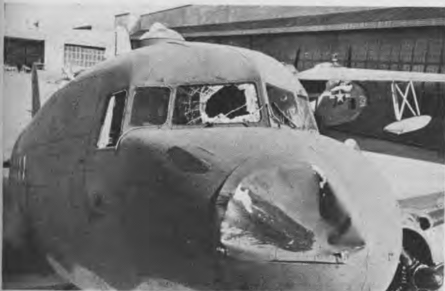
THIS R4D RETURNED SUCCESSFULLY TO BASE AFTER DAMAGING ATTACK BY WEST COAST DUCKS
