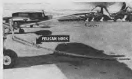
TIE-DOWN STANDS A TEST OF 2000 LBS
