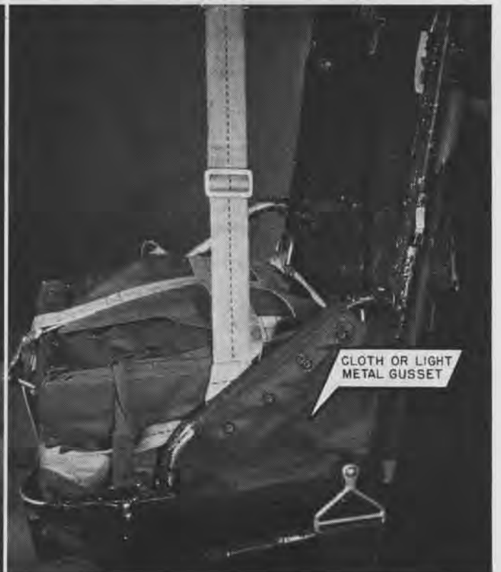
PARACHUTE RETAINING STRAP INCORRECT INSTALLATION
