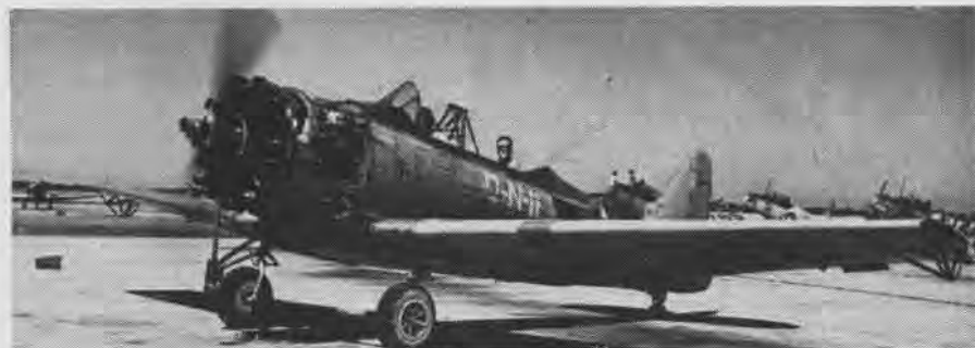
STUDENT PILOTS at NAS CORPUS CHRISTI develop taxi technique in this specially rigged taxi-trainer. At the controls of this airplane, an SNJ rigged with wing tip skids and a nose wheel, students can work out their taxi problems and study methods of avoiding ground loops without endangering either themselves or their plane. Developed at Corpus Christi, the trainer is believed to be the only one of its kind in the Navy.
