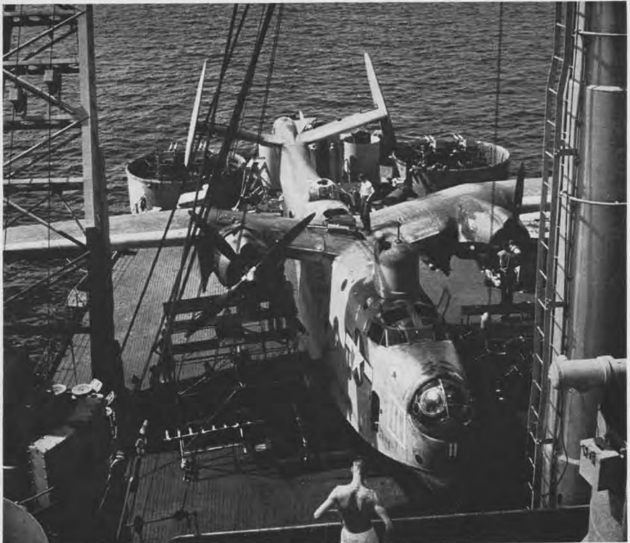
In advanced areas lacking seaplane ramp facilities, tenders have to act as airfields for the Navy's big PBM's. Here one of the 43,000-pound flying boats is standing on beaching gear on the deck while mechanics of tender give it a service in short order
