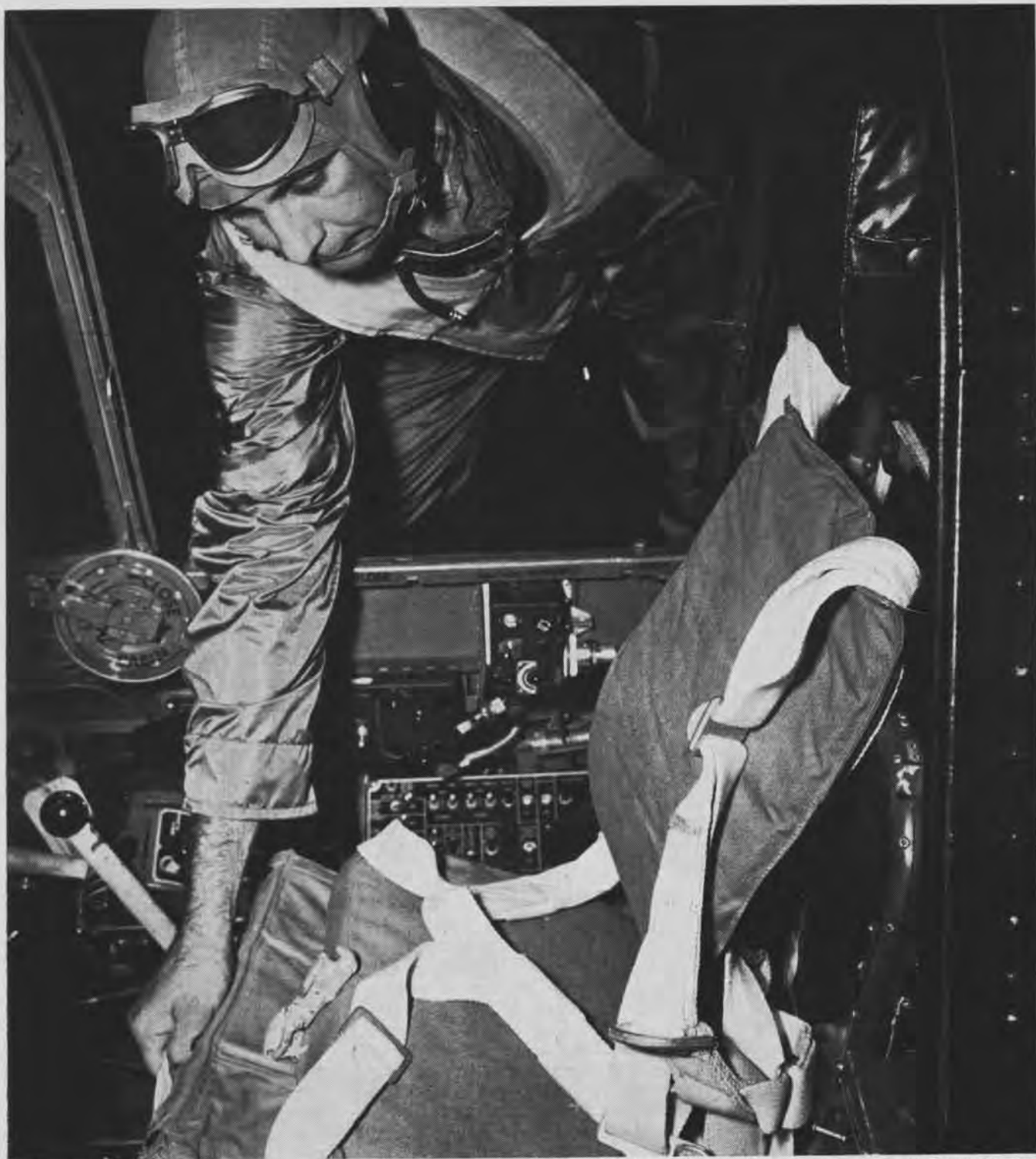
IMPROVED PARARAFT KIT CONTAINER MAKES PARARAFT KIT READILY AVAILABLE AFTER A DITCHING, WHEN EVEN A SECOND COUNTS
