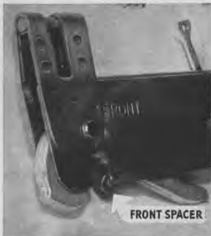
OVERLOAD ON BOMB SHACKLE WILL DAMAGE
