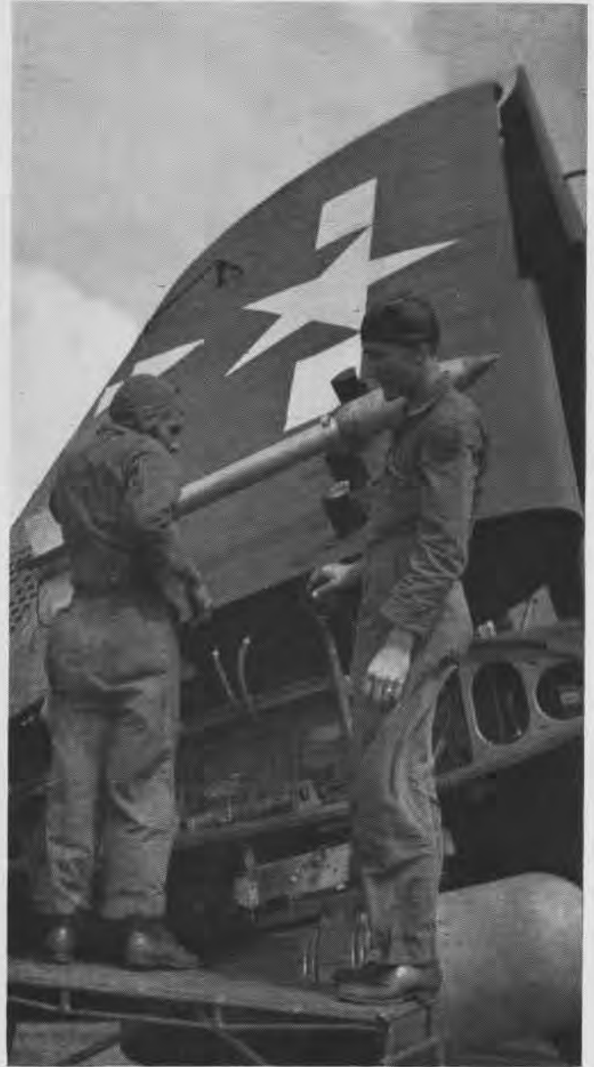
Rearming of planes on island air base is job for CASU ordnance-man. This 5" AR rocket carries plenty of punch for the Japs
