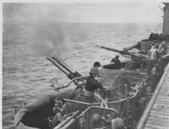
Gunnery crews of CVE get firing practice after first learning fundamentals of aiming on school's synthetic gunnery devices, then firing at Pacific beach range. Gunnery of 40 mm. batteries throw out AA barrage during a lull in flight operations
