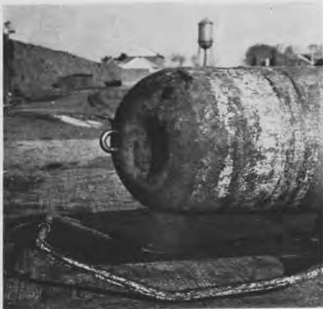
This aircraft torpedo was dropped at high speed without the drag ring attached and suffered dent in heavy exercise head
