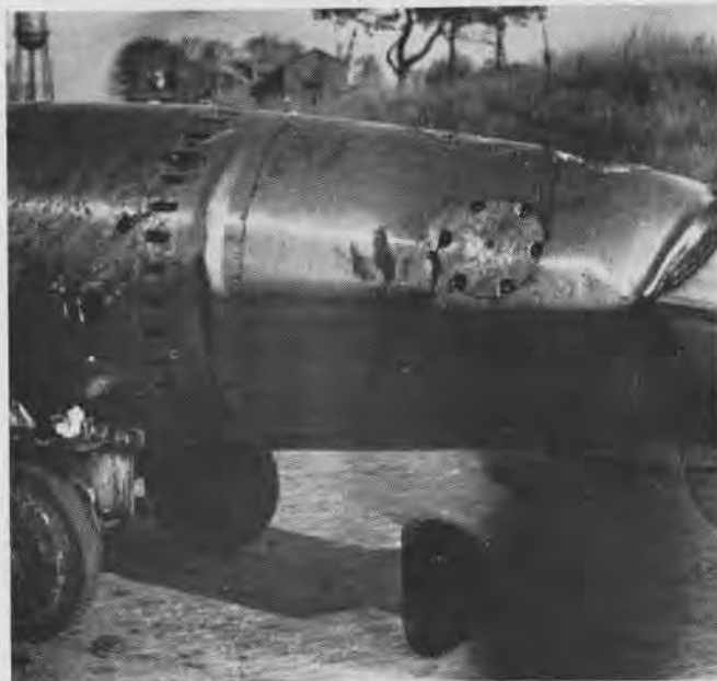
High speed launching without drag ring resulted in accordion-wrinkling of afterbody shell caused by high deceleration of torpedo
