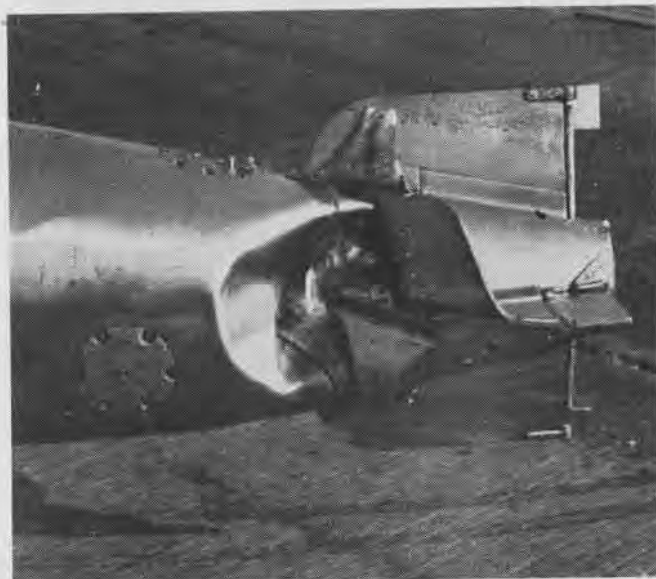
This is another example of "tail slap" damage resulting from Newport trials of torpedoes equipped and not equipped with drag rings
