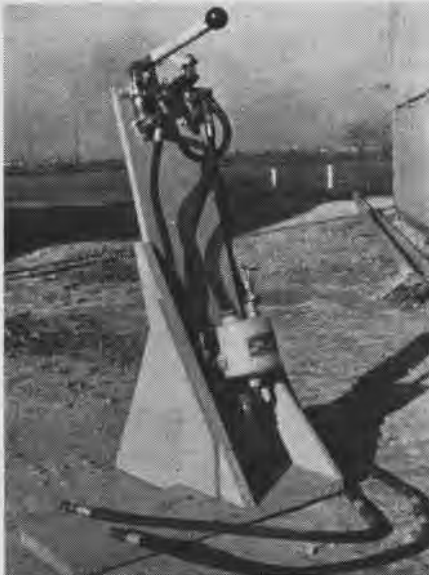
PORTABLE PUMP IS MADE FROM SALVAGE
