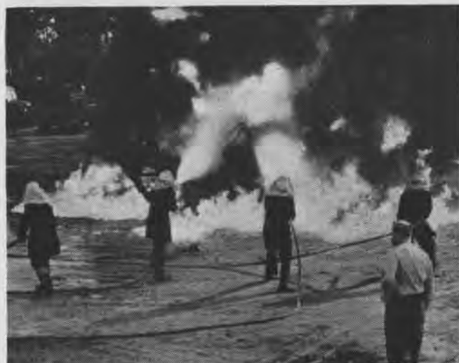
Fog barrier on each side of cockpit shields pilot from flames. Fire is controlled by application of foam over gasoline spill
