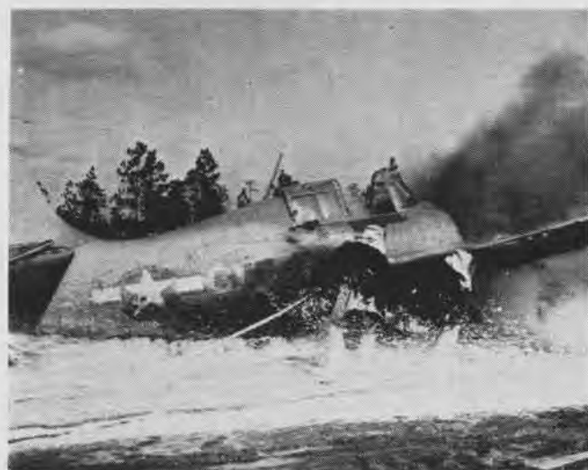
Protecting foam is laid on behind CO 2 fire fighters. Foam prevents flashbacks as men move up to knock down flames under wing
