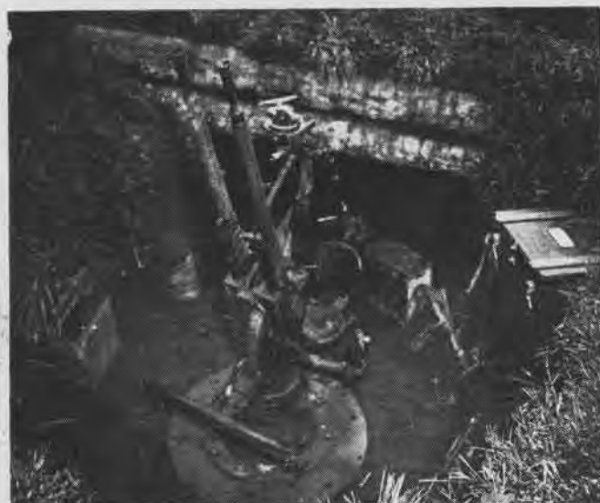
13.2 mm batteries are used to protect heavier AA from strafing; Japs often mount 13.2's in covered pillboxes for beach defense
