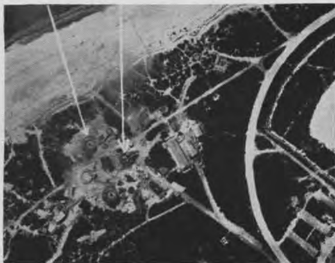
Typical 127 mm layout has three revetments in an arc with the center one empty. Fire control building is opposite empty revetment
