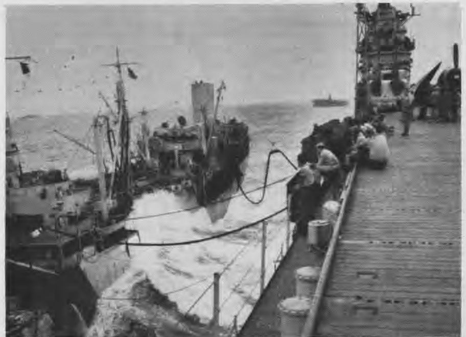
AFTER HARD strikes against important Jap bases, units of a task force rendezvous for refueling at sea. Fuel is pumped aboard the flattop through two lines rigged from the tanker to cv. Ships maintain speed while refueling operation is under way to keep position in task force. Calm sea facilitates refueling. Wash from between the two ships sprays water over the tanker's deck. Smoking lamp is always out during refueling.
