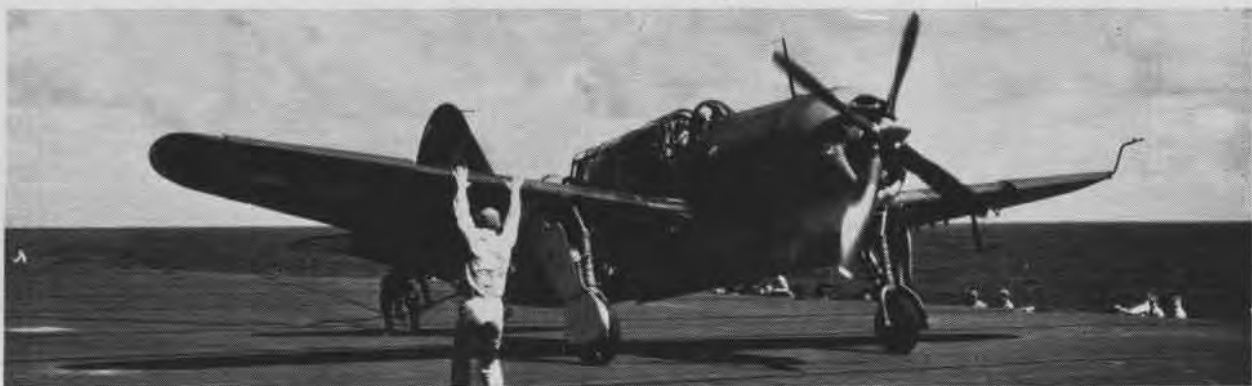
FLY 3 OFFICER SIGNALS "HOLD IT" WHILE HOOKMAN RUNS IN FROM REAR TO FREE HELLDIVER FROM THE ARRESTING WIRE
