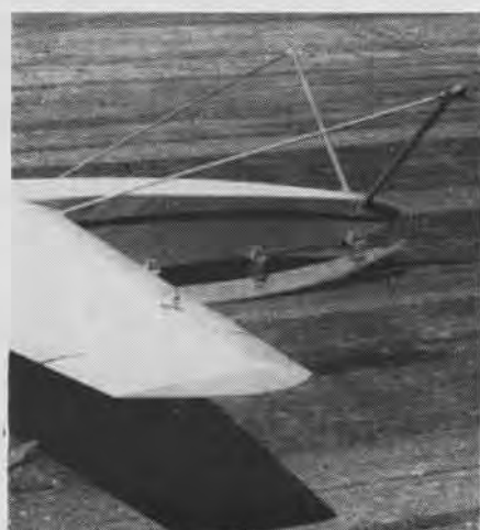
Long rods serve as braces extending from nose of target back to leading wing edge
