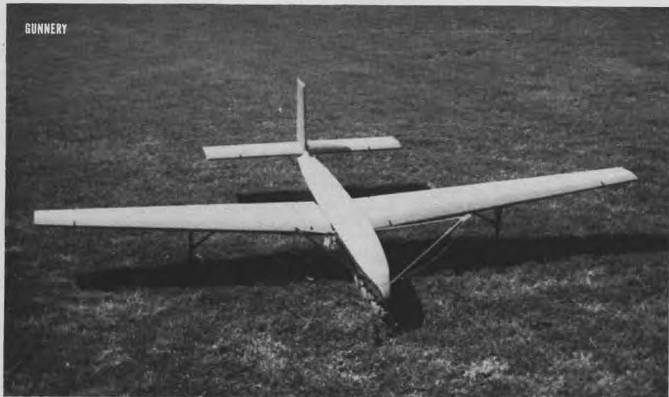
NAVY'S WINGED TARGET IN FLIGHT CLOSELY FOLLOWS ALL MANEUVERS MADE BY THE TOW PLANE TO AVOID AIM OF THE GUNNERS
