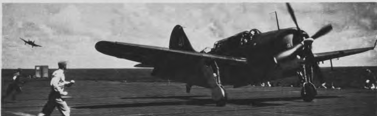
ARRESTING WIRE HALTS SB2C AS FLY 3 OFFICER AND HOOK MAN SPRINT OUT TO PLANE; TEAMWORK SPEEDS OPERATION
