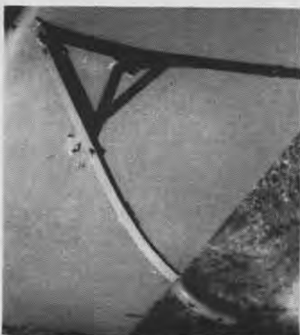
Metal shod skids which are secured to the lower side of both wings prevent dragging
