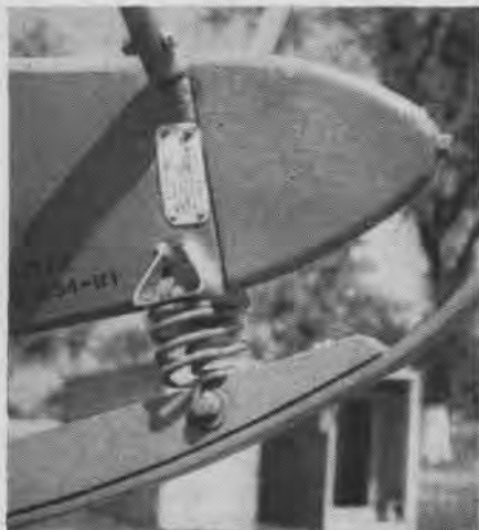
Series of coil springs is built into the main skid to take up major landing shock
