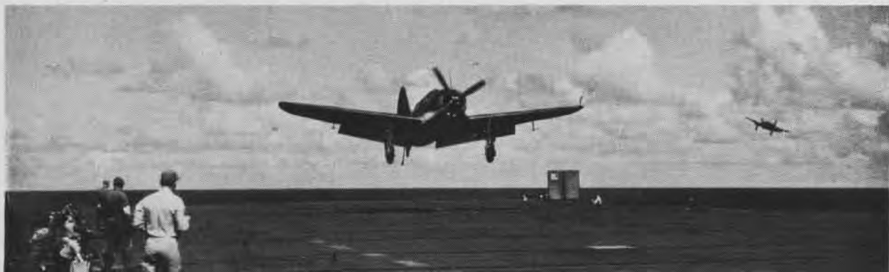
GIVEN A CUT BY THE LSO, AN SB2C COMES IN NICELY OVER THE CENTER OF THE DECK; DECKMEN LINE THE WALKWAY
