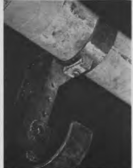
CURVED METAL BRACKETS HOLD ROCKETS
