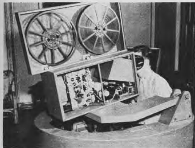
Synthetic devices keep pilots in tip-top shape. Panoramic Gunnery Trainer MK. 2 is used as an advanced practice device for turret manipulation and aerial gunnery sighting. When pilot thinks he is in firing position, he presses trigger, and all hits are recorded
