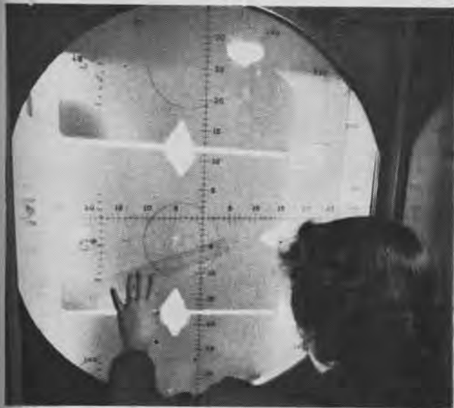
Motion pictures made during assessment runs calibrated on bomb sight projector are accurately read by skilled WAVE operator
