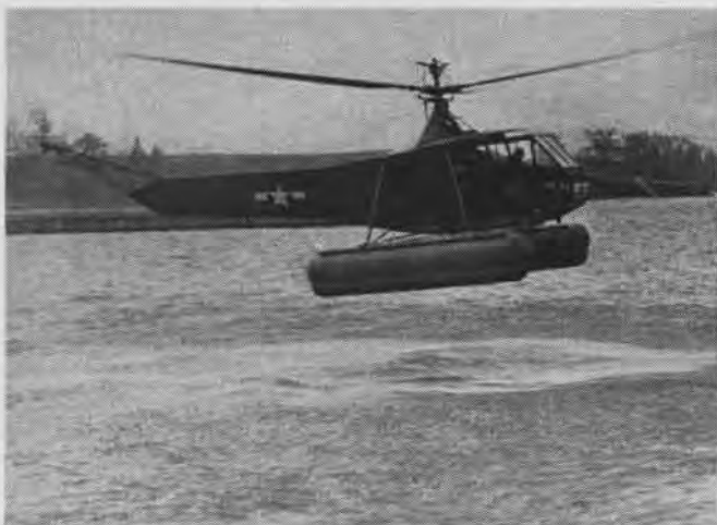
Navy pilots flight-test helicopters to determine water landing characteristics, weight lifting capacities under controlled conditions
