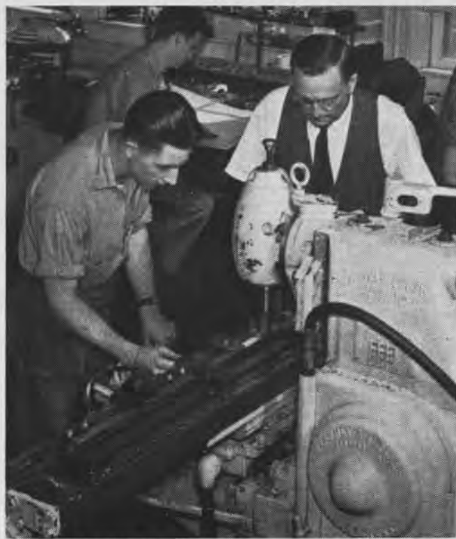
MILLING MACHINE IN INSTRUMENT SHOP IS ACCURATE TO .0005
