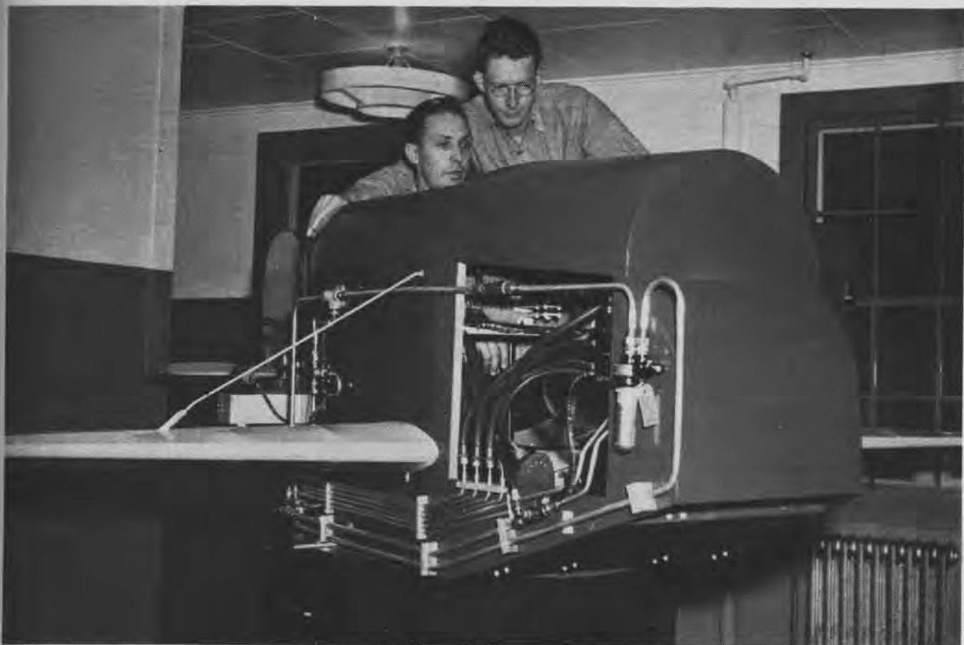
INSTRUCTOR AT THE CONTROLS GIVES A TRAINEE THE WORD ON OPERATION OF A LINK TRAINER RIGGED UP WITH AN AUTO-PILOT
