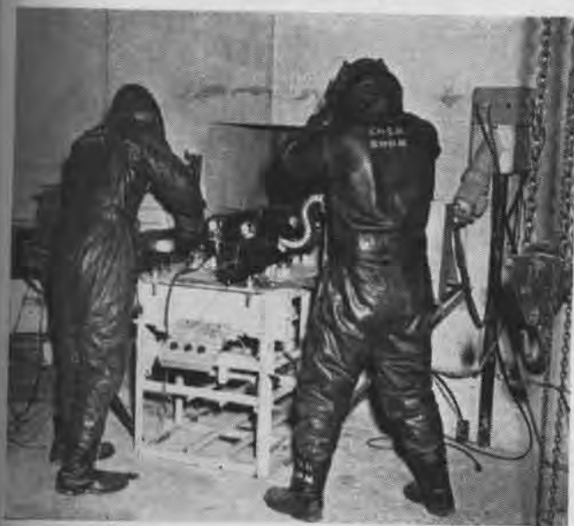
From Armament TEST's specially designed cold chamber, engineers ground fire machine guns and cannon in temperatures of -75^{\circ} F.
