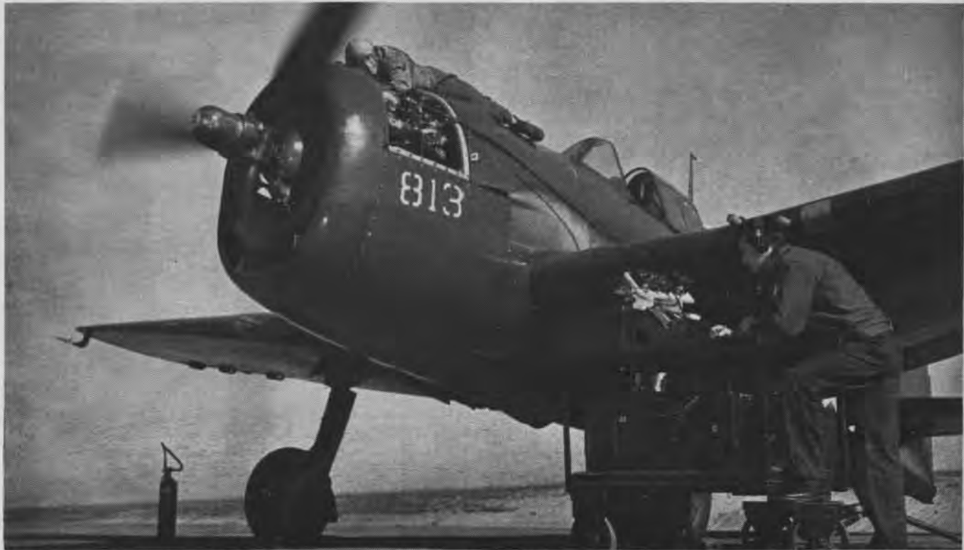
RADIO TEST ART PROBES FOR NOISE INTERFERENCE INCHES BEHIND SPINNING HELLCAT PROP: SECOND ART READS VHF RECEIVER
