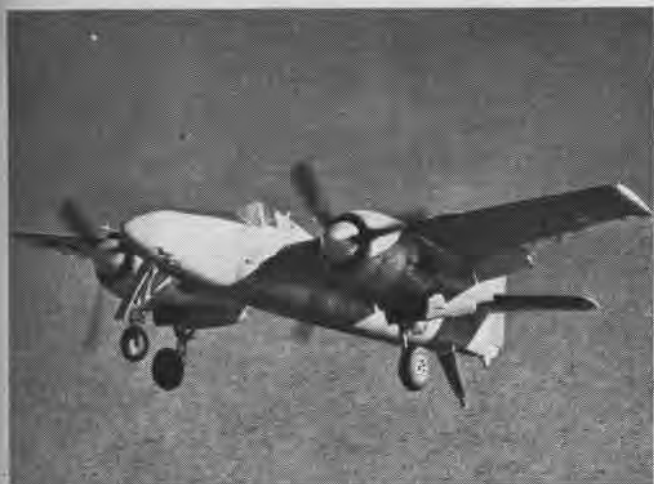
Tigercat with tricycle landing gear and arresting hook down, comes in for simulated carrier landing during Patuxent flight test
