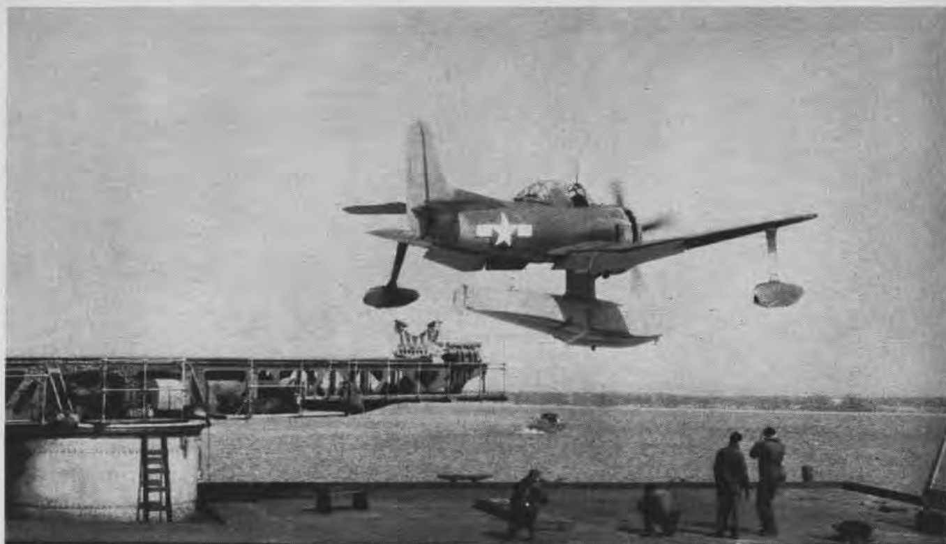
VO/VS PROJECT OFFICERS CONDUCT CATAPULT TRIALS TO DETERMINE THE NEW SEA HAWK'S PERFORMANCE UNDER ALL CONDITIONS
