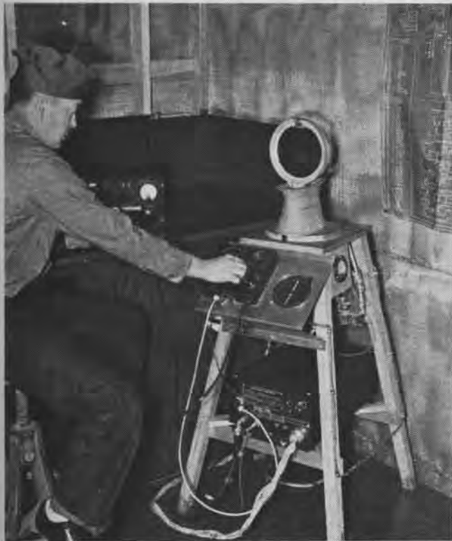
ART BENCH TESTS DIRECTION FINDER IN COPPER SCREEN ROOM
