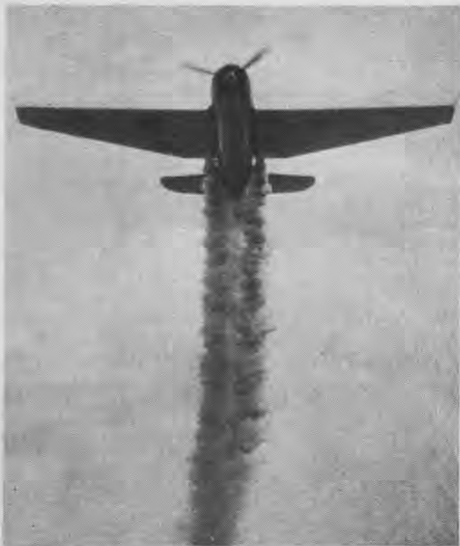
TACTICAL TEST TBF TRAILS SWATH OF DDT OVER A JUNGLE AREA
