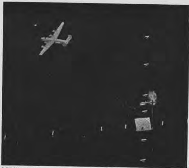
A PB4Y releases a bomb over a specially constructed target in an ARMAMENT TEST project for the evaluation of a new bomb sight
