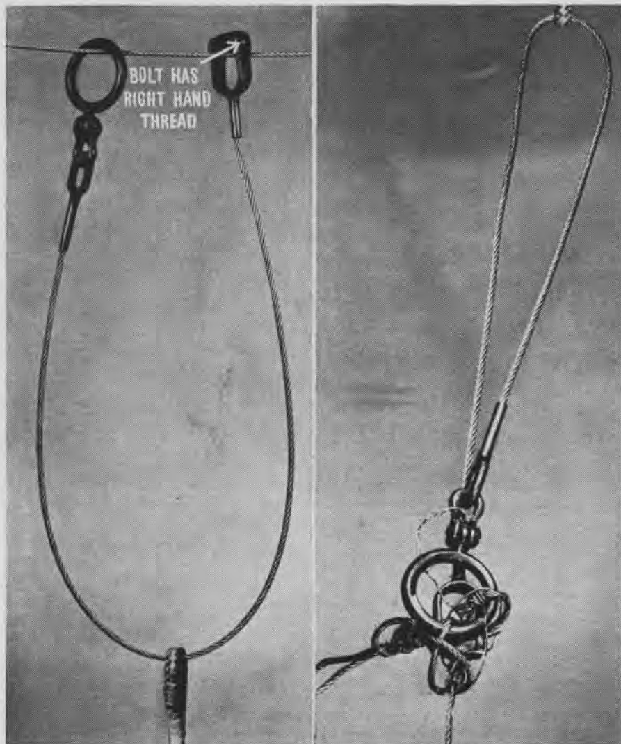
TARGET STREAMS FROM BIGHT OF LEADER; SNARL CATCHER HANGS ON SNARLED CABLE
