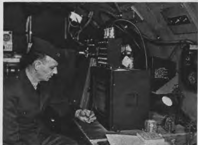
Engineer uses a Brown Recorder to tabulate temperatures and temperature changes of all important engine points during test
