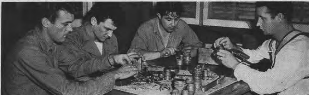
CONVALESCENT PATIENTS CLEAN AND REPAIR CANNON PLUGS FOR ELECTRICAL INSTALLATIONS; EACH MAN HAS WORK TO DO
