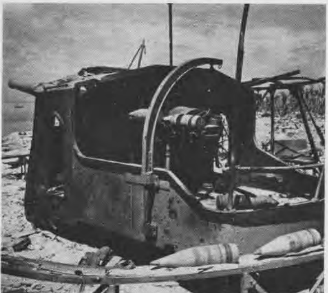
12-INCH STEEL AMMUNITION TROUGH ALMOST ENCIRCLES JAP GUN
