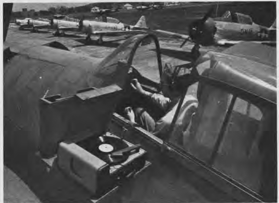
COCKPIT CHECKOUT recordings, developed by BuAer's Special Devices Division, assist flight personnel to check out in various types of aircraft in Cockpitainers or in the operational aircraft itself. A shelf is hung over side of cockpit to hold album and phonograph. A headset is provided for individual instruction. A loudspeaker may be used for large groups. Recordings have been prepared for almost all types of naval aircraft.
