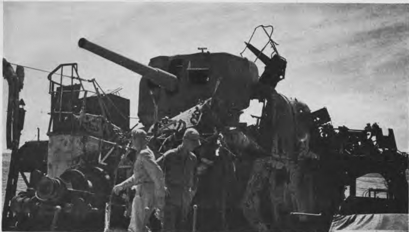
120 MM. NAVAL GUN, FOUND ON DD'S OF MINEKAZE, WAKATAKE AND MOMI CLASSES, OFTEN IS USED ASHORE FOR COAST DEFENSE WORK
