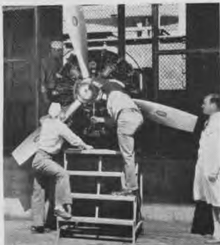
Engine test stand gives students chance to trouble shoot, and perform engine run-ins
