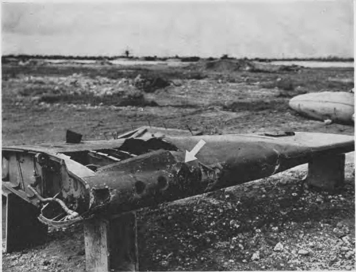
CORSAIR WING SHOWS DAMAGE DONE BY OVERHEATED GUNS WHICH THREW BULLETS OUT BLAST TUBE, CAUSING EXPLOSION IN WING
