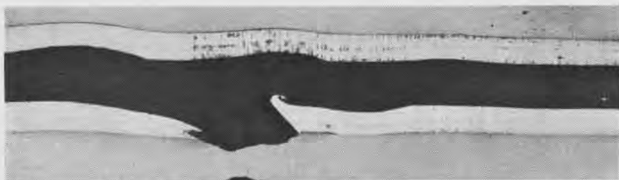
.50 CAL. GUN BARREL IS SO DEFORMED BY OVERHEATING THAT BULLETS GO OUT SIDE
