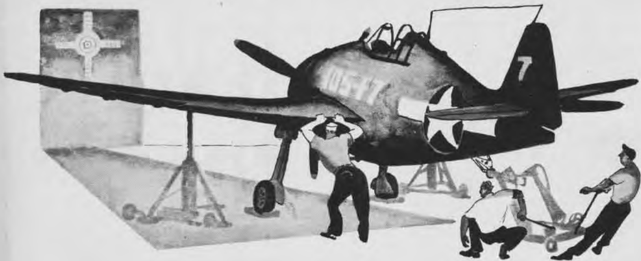
BORESIGHTING ACCURACY PAYS OFF WHEN A ZERO IS IN THE PILOT'S SIGHTS. HERE CASU MECHS LINE UP THE GUNS ON A HELLCAT TO INSURE THE ACCURACY OF DISPERSION PATTERN
