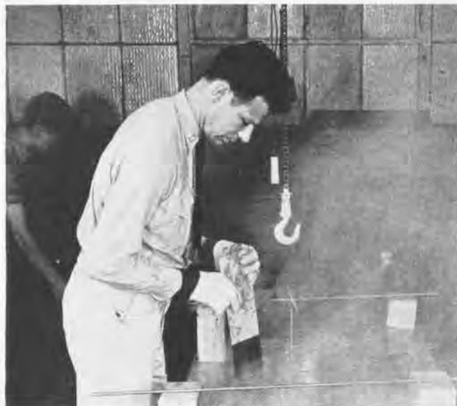
1 First step in preparing plastic bath for preservation of guns is to get the solution at proper temperature for dipping
