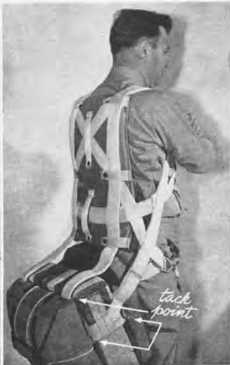
New pans fit next to body with the seat type parachute. Seat pan cuts discomfort from sitting long hours on chute, raft
