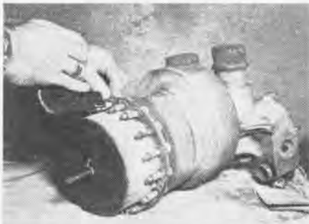
CLECO'S HOLD MASKING CUP IN SANDBLAST
