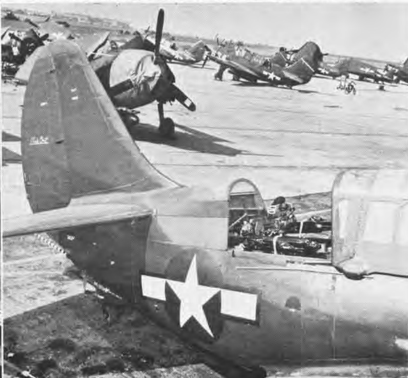
GUNS CAN BE SHIPPED LASHED TO MACHINE GUNS IN SB2C COCKPIT
