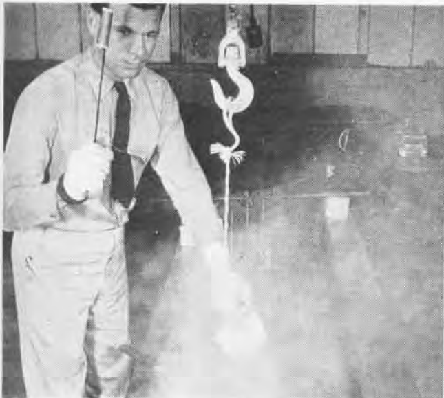
3 After temperature of plastic solution is at 375° F, machine gun is suspended from hoist and given 1/16" protective coat
