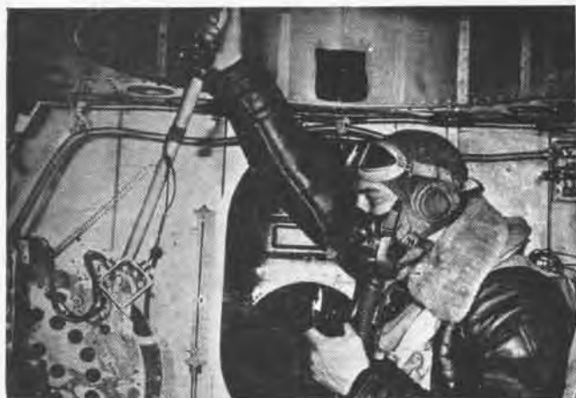
Once the target is streamed, the ordnanceman controls speed of the cable rolling off reel. Navy provides electrical, hydraulic or wind-driven reels to take care of thousands of feet of cable
