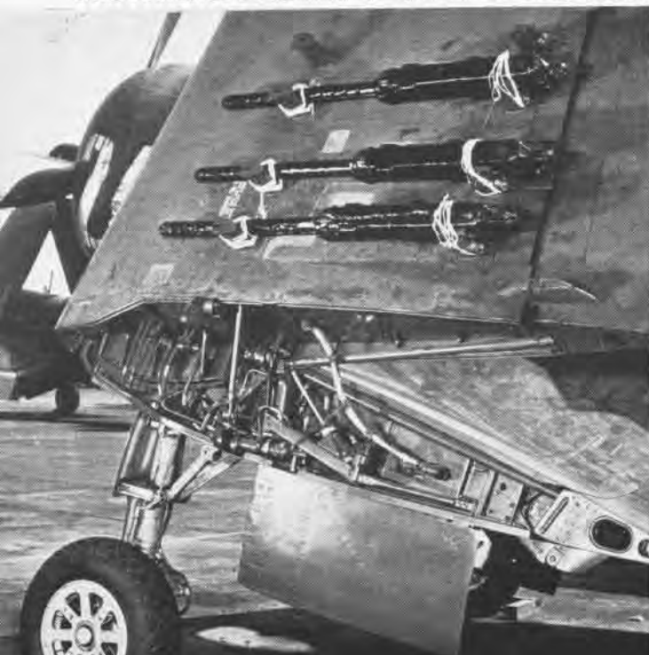
GUNS PROTECTED BY COATING TIE TO WING FOR TRANSPORTING
