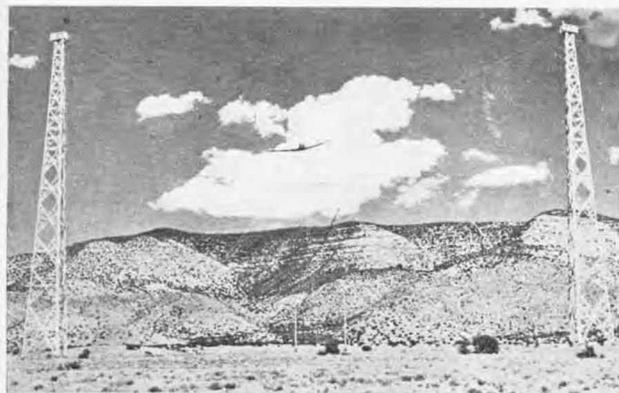
SUSPENDED MODEL AIRPLANE WAS USED AS A TARGET AT NEW MEXICO PROVING GROUND
