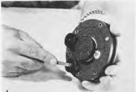
FILE SCREW DOWN ON SHUTTER SPEED KNOB
