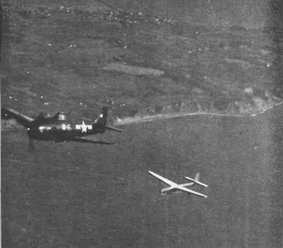
STRAFING HIGH SPEED TARGET; THIS TYPE CAN BE SNATCHED FROM CARRIER DECK OR LAND
