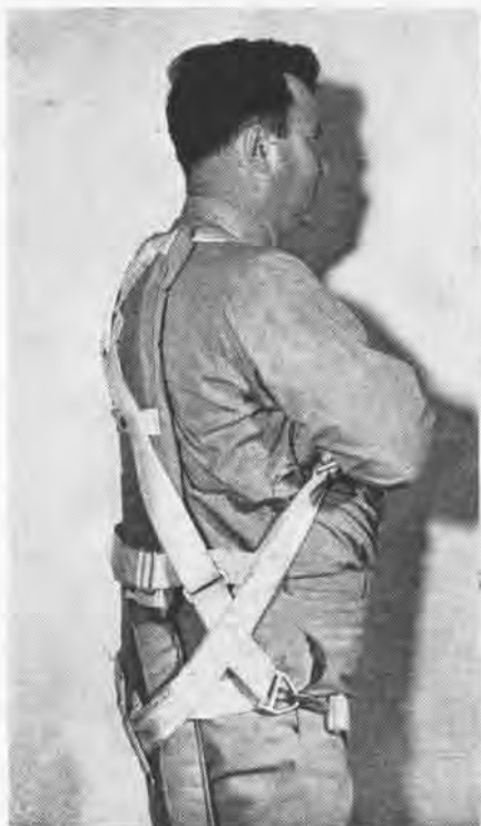
Seat and back pans are shown installed on quick attachable type parachute harness to increase pilot comfort on long hops
