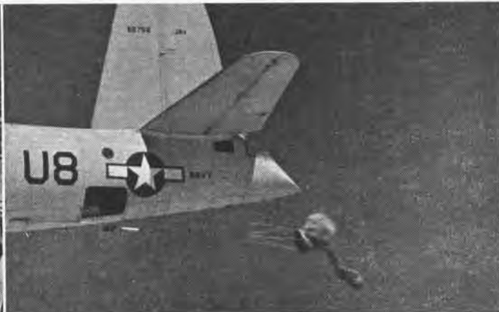
Secured by numerous cables, a tow target sleeve catches the wind after release from JM. Firing at targets such as this has helped train gunners who later shot down more than 17,000 Jap aircraft
