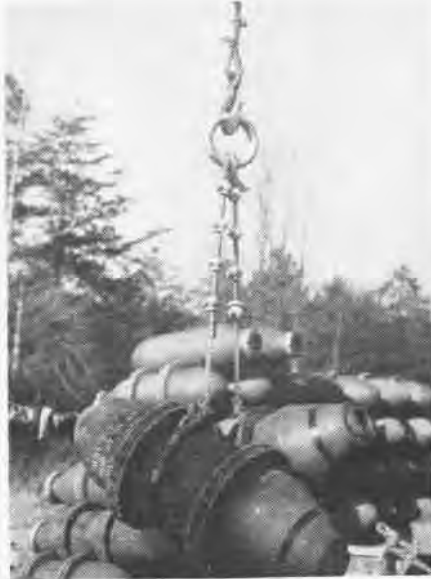
MK 25 SLING CABLES LOOPED ON BOMBS
