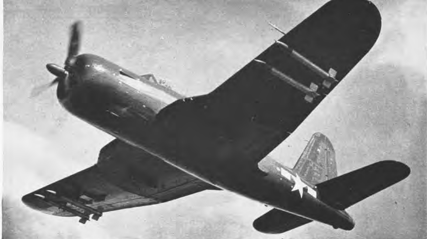
FR-1 CARRIES FOUR 50-CALIBER MACHINE GUNS AND TWO 1000-POUND BOMBS; CAN BE RIGGED FOR DETACHABLE ROCKET RAILS
