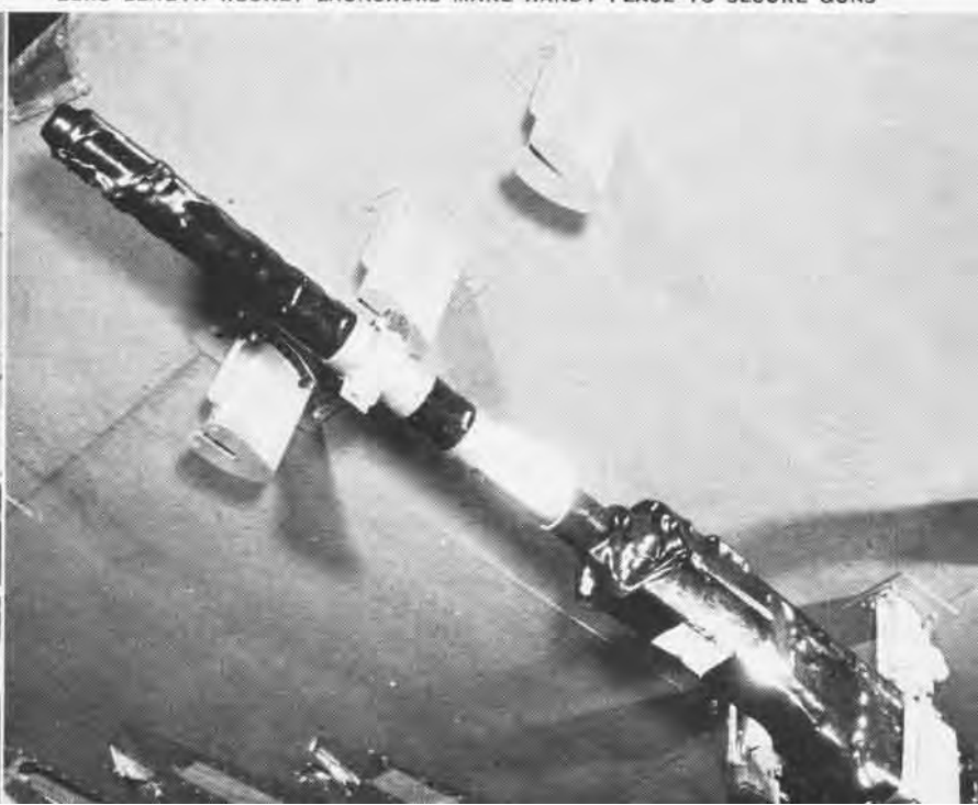
ZERO LENGTH ROCKET LAUNCHERS MAKE HANDY PLACE TO SECURE GUNS
