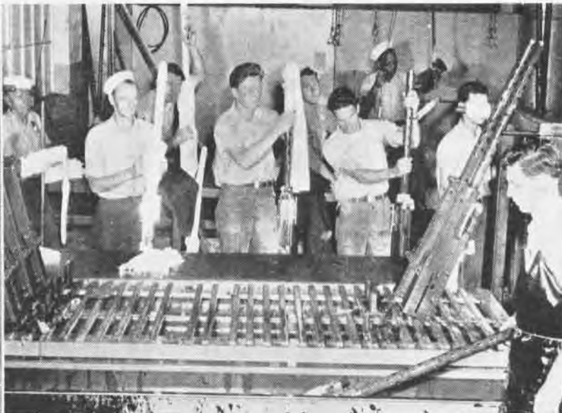
2 Ordnancemen preparing the guns for dipping. Cloth bags are slipped over them and sewn at rear end after cleaned gun is inserted
