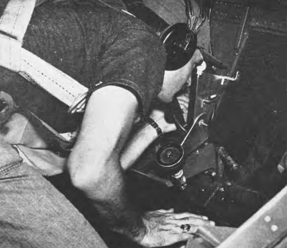
OPERATOR ADJUSTS SIGHT BUBBLE TO ALTITUDE OF PLANE, DROPS GEAR FOR SURVIVORS
