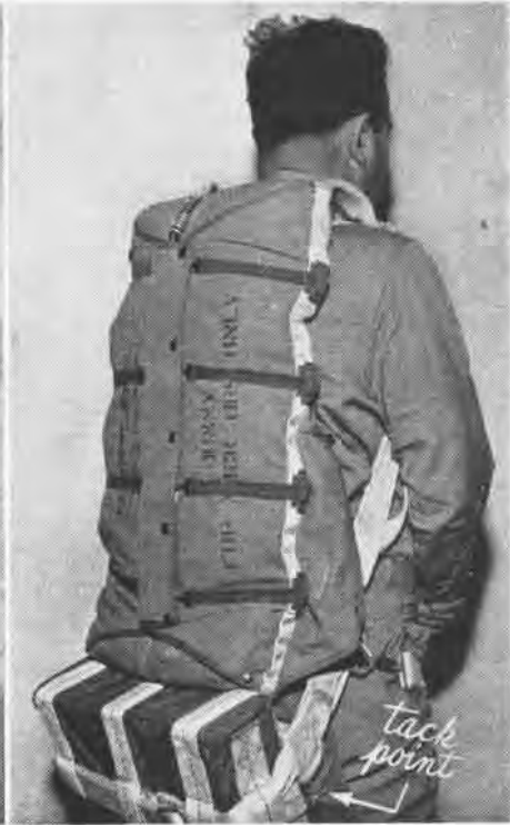
When used with back-type parachute, no back pan is necessary, but the seat pan is installed as usual, tacked to raft
