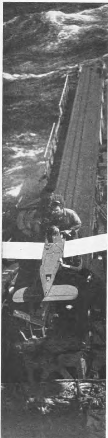
Hundreds of TDD drones, launched from catapults on battleships or other large vessels, furnished gunnery training for their anti-aircraft batteries during lulls between action in Pacific. TDD-3 has a 20 hp motor
