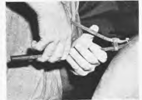
RIVET SETTER UTILIZES LEVER PRINCIPLES
