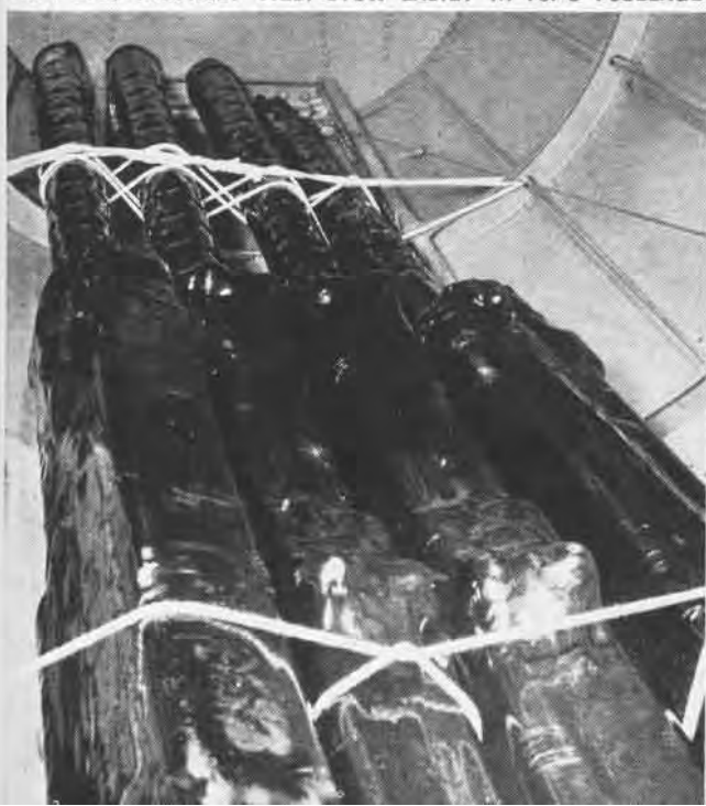
FOUR 50'S, SECURELY TIED, STOW EASILY IN F8F'S FUSELAGE
