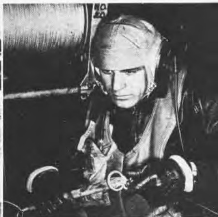
VJ-15 ordnanceman attaches target to tow cable by slipping ring of target onto exchange device at the end of the wire cable
