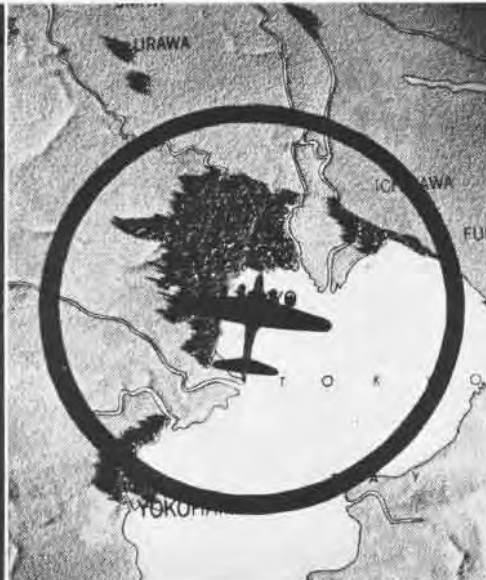
Small circle in center shows plane's altitude at 10,000 ft. Scope of radar gear attached to trainer device picks up the landmarks that are seen on a real bombing mission
