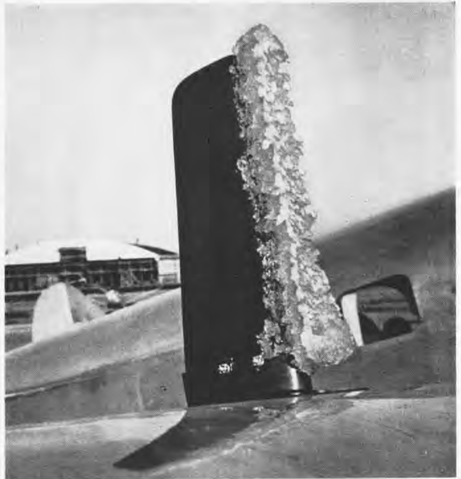
TELL-TALE STRUT COLLECTED RIME ICE (WHITE) AND GLAZE ICE ON SPECIAL FLIGHT TEST
