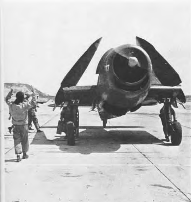
CHOCK MEN pull out wheel stops as plane director guides the aircraft up the flight "deck." Teamwork of ground crew is vital in this work
