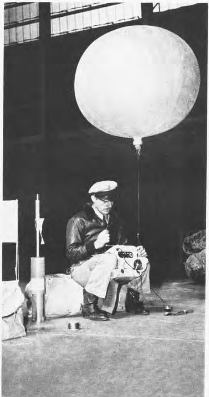
IN NORMAL OPERATION SET IS BETWEEN KNEES. POWER CRANKED
