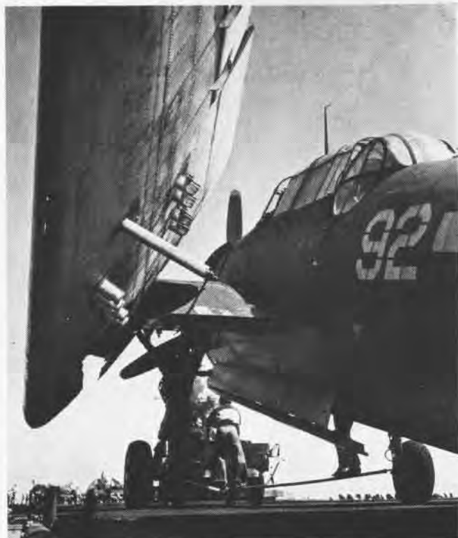
EACH MAN has a specific job. These men practice spotting using a tractor to tow a TBM into its proper place on the flight deck
