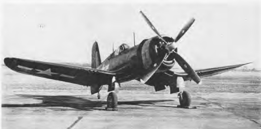
THE NAVY'S newest version of the battle-tested Corsair is the F4U-4, a souped-up model with more power, climb and speed. Chief apparent change in the plane is its four-bladed propeller and the chin scoop, new with the Corsair but present in the F6F and SB2C. The new model has a 2100-hp. Pratt & Whitney Double Wasp engine, larger and fewer cowl flaps, 1000 feet a minute more climb and a boost in its top ceiling.
