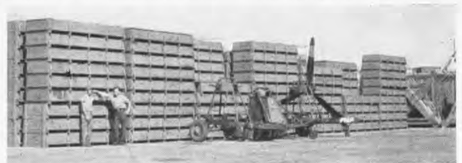
IN SPECIAL BOXES, PROPELLERS MAY BE STORED IN THE OPEN WITHOUT DETERIORATION
