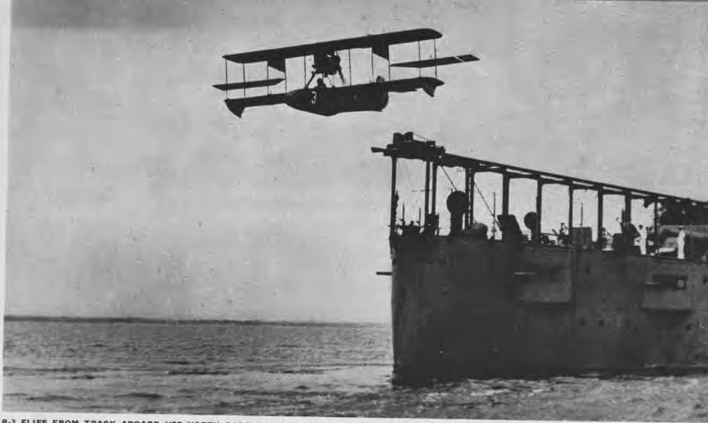
B-3 FLIES FROM TRACK ABOARD USS NORTH CAROLINA, ONE OF SEVERAL CRUISERS EQUIPPED WITH THE LAUNCHING DEVICE BY 1916
