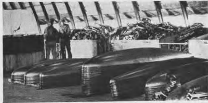
AFTER Knock-down tanks save precious cargo space. Overseas unit does the assembly job for Naval Aviation
