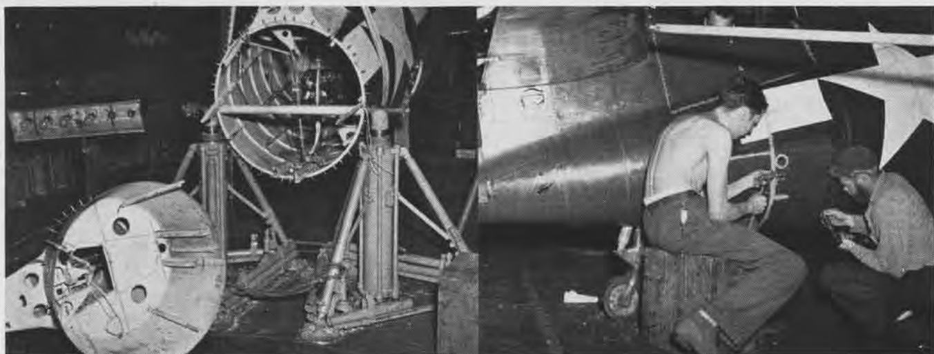
AN FM2 WAS BADLY NEEDED SO SPLICING WAS CALLED INTO PLAY
