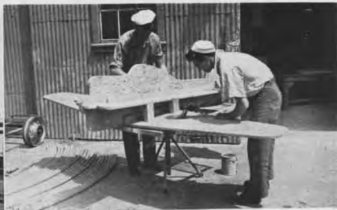
Combat aircrew training units employ yellow-painted, wooden model Zeros as truck-towed targets. Training Devices Unit built
