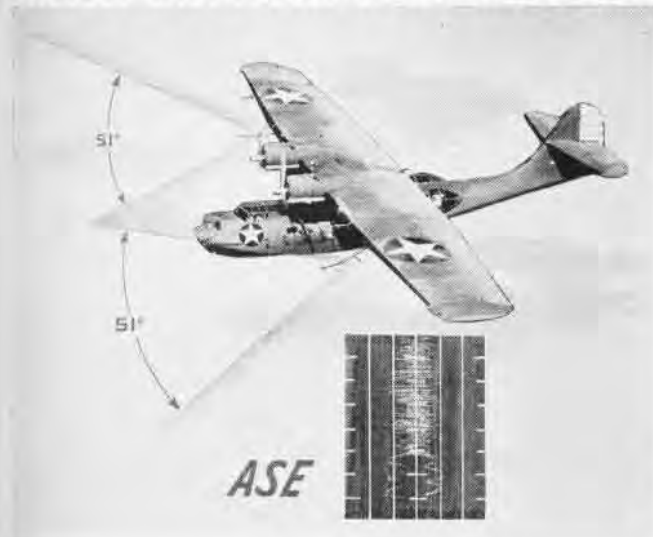
First U.S.-produced radar used in naval aircraft was Easy . Widely used in Aleutians and SoPac, it was heavy, gave azimuth check
