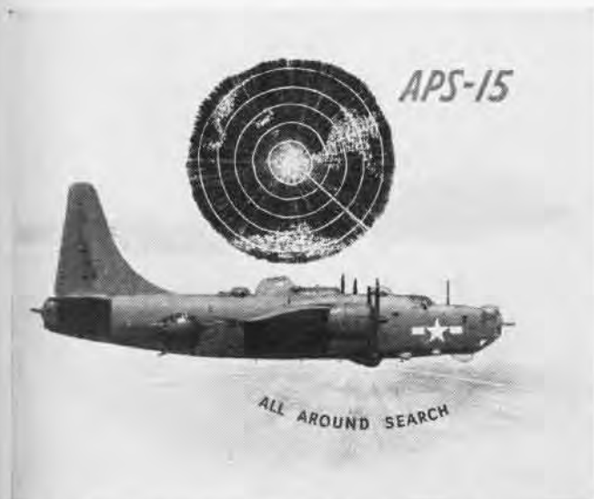
To permit bombing in foul weather, Navy combined George and Dog 's best features to produce Mickey . It was Jap ship scourge
