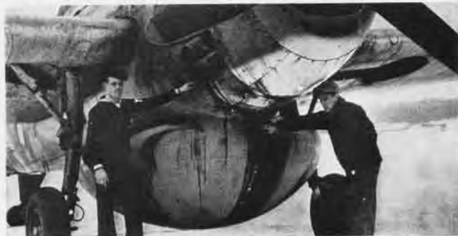
BULBOUS 8x3 FT. RADOME MAKES THIS TBM A PILOT'S PROBLEM
