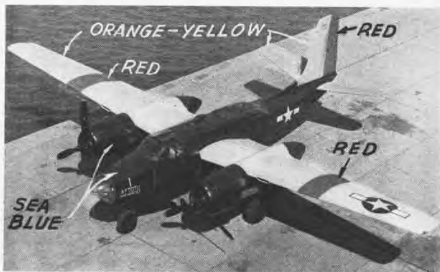
VARI-COLORED PAINT JOB OF RED, ORANGE-YELLOW AND BLUE MAKES THE JD-1 VISIBLE
