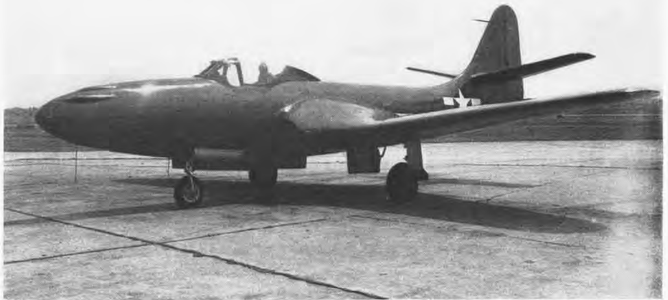
First Navy fighter plane to be powered exclusively by jet engines, the Phantom XFD-1 is propelled by Westinghouse gas turbines. Designed for carrier operation, the XFD-1 does better than 500 mph and may herald faster Navy jet propelled planes of future.
