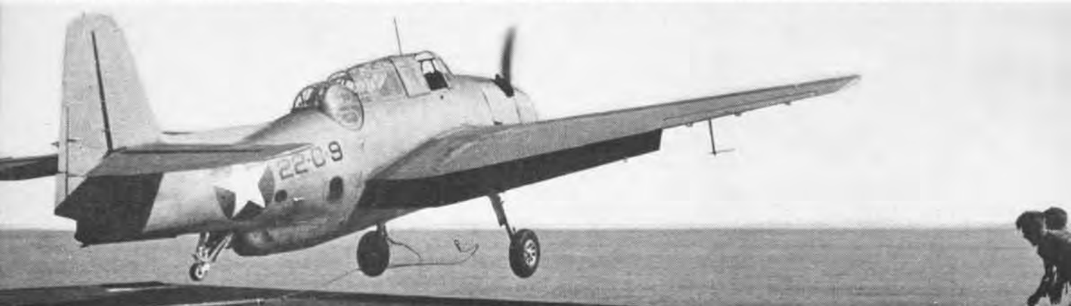
6. Holdback man signals catapult panel board operator "proper tension now applied." New improvements will gain seconds by eliminating this procedure by using automatic tensioning.
