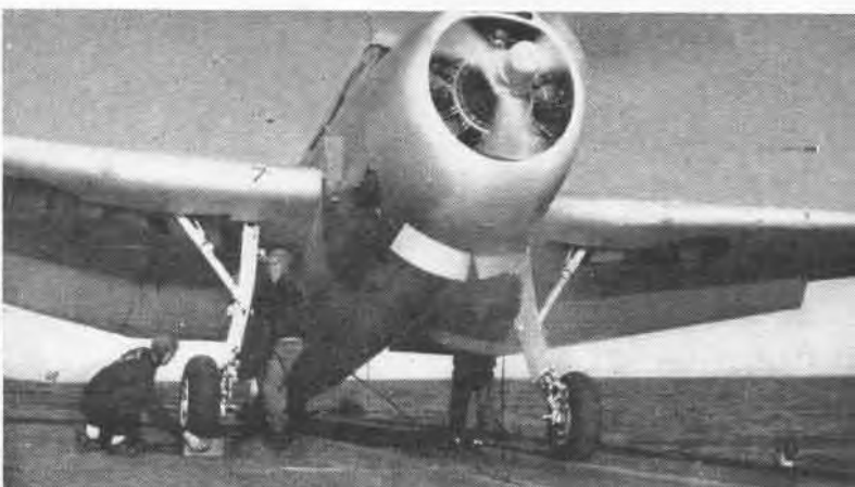
5. While bridle is being attached, the wheel chock is removed and system is being made ready for tensioning. Bridle men stay at their positions until tension is properly set.
