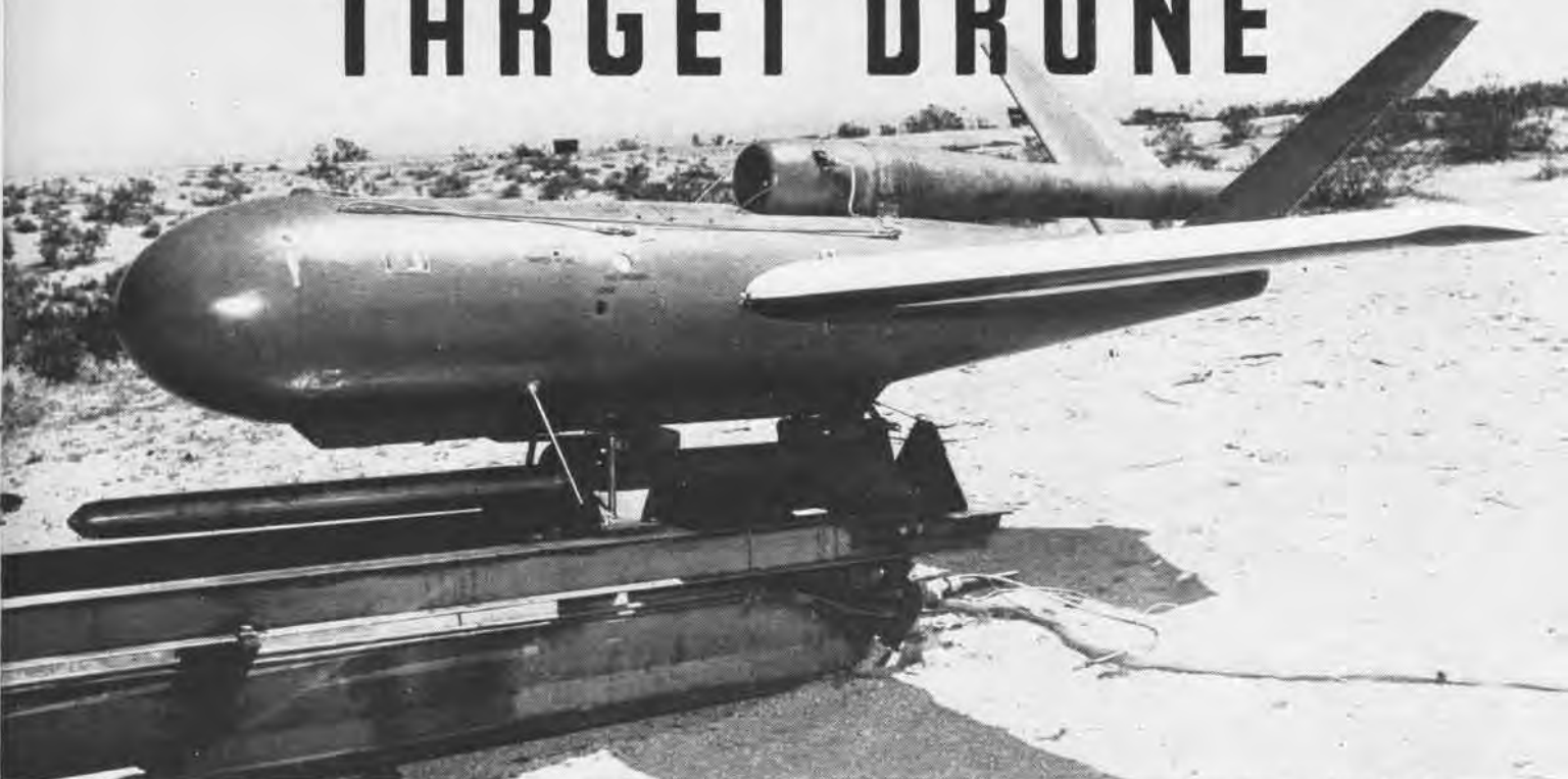
KDD-1 POISES ON COMPRESSED AIR CATAPULT AT MOJAVE; PISTON BELOW DRONE PENETRATES WATER 'CUSHION' AT END TO HALT CAR
