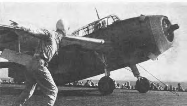
7. Signal is given by catapult officer to fire catapult. Signal is relayed to operator below deck. Terrific power of catapult is accomplished by a hydraulic ram under compressed air.
